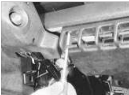
7.2a Removing the switch panel screws - early models
