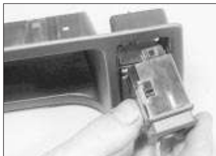
7.3 Removing a switch from the instrument panel surround
