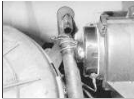
11.2 Disconnecting the heater hoses
