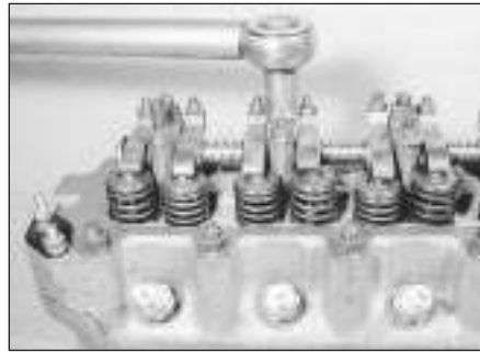
4.13 Tightening the cylinder head nuts
