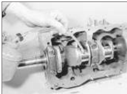
9.19b Lubricating a crankpin
