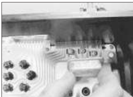
15.3 Extracting the voltage stabilizer
