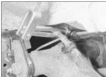
30.14 Clamp fitted to rear brake hose
