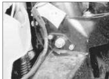
6.9 Front suspension upper arm pivot front retaining plate
