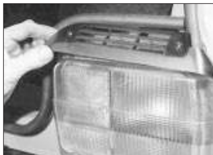
12.8 Removing the rear lamp cluster air vent
