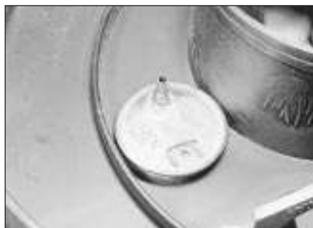
4.2 Air cleaner temperature sensor (inside air cleaner body)
