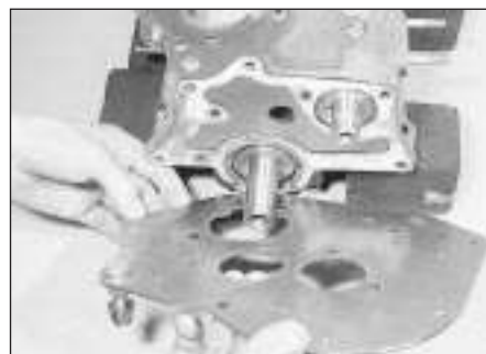
10.3 Removing the engine front plate
