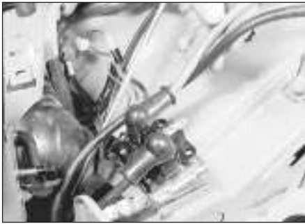
3.3 Removing the solenoid
