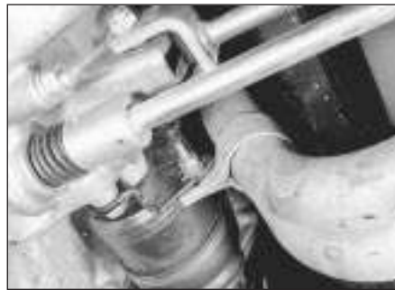
27.5b Exhaust system front mounting clamp (1.3 HLS)
