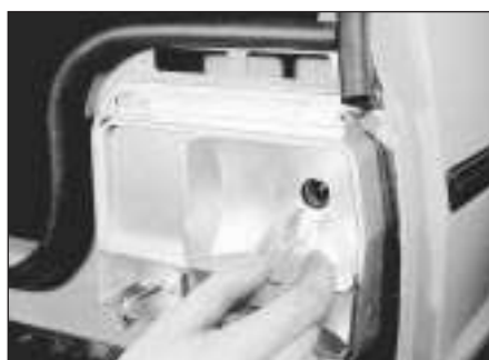
12.10 Removing a stop light bulb
