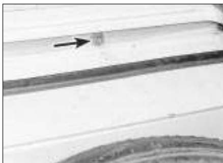
30.17b Hydragas unit inner strap bolt viewed from the spare wheel well
