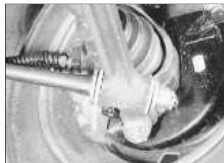
5.4 Anti-roll bar-to-lower suspension arm joint
