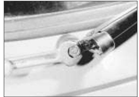
21.3 Unscrewing the wiper arm spindle nut
