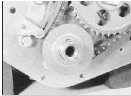
6.9 Correct location for the crankshaft oil thrower
