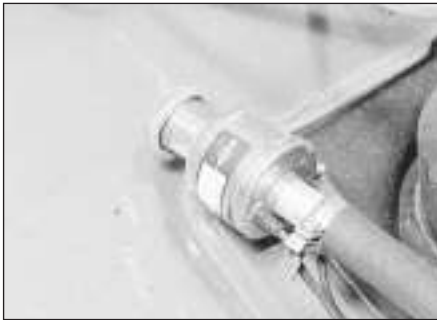
17.1 Anti-run-on valve is mounted on bulkhead
