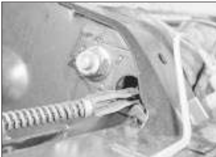
30.21b . . . and withdraw the handbrake cable ends through the access holes
