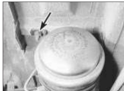
30.17a Hydragas unit outer strap bolt (arrowed)
