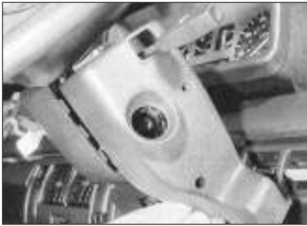
5.4 Removing the right-hand steering column cowl
