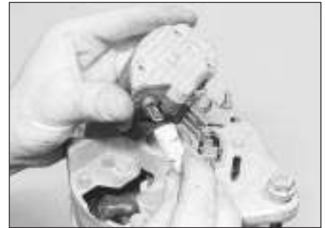
13.3C . . . and disconnect the wiring
