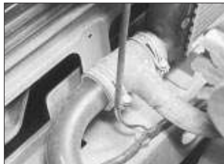
1.4 Bottom hose with take-off for oil cooler
