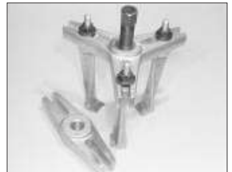
Two- and three-legged bearing puller
