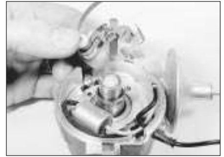
34.3 Removing the contact breaker set (Lucas)
