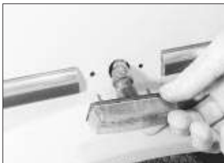
12.7 The side repeater lamp being refitted with adhesive
