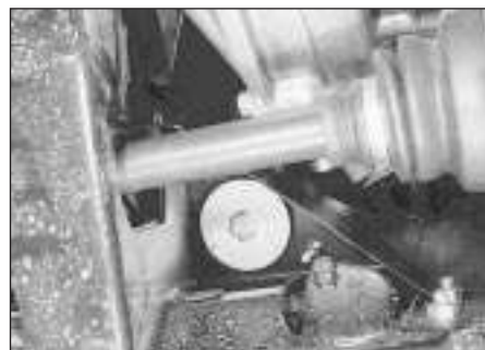
3.29b Right-hand rear engine mounting (from below)
