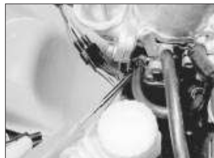
15.8 Adjusting the mixture
