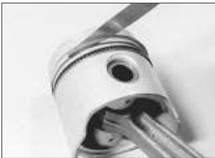
9.17 Checking the compression ring groove clearance (1275 cc engine)
