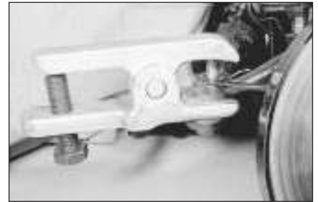
17.3b Using a separator tool to release the tie-rod end balljoint
