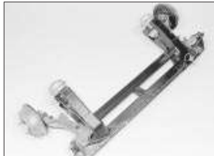
30.22 Rear subframe removed from the car
