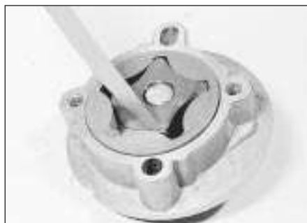
8.9e . . . and rotor lobe clearance (off centre)
