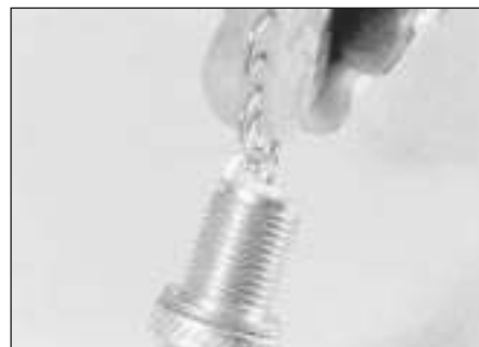
6.9c . . . and adjusting the gap using a special tool
