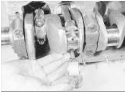
9.6 Removing a big-end bearing cap
