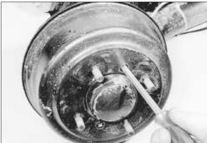
5.2 Removing the brake drum
