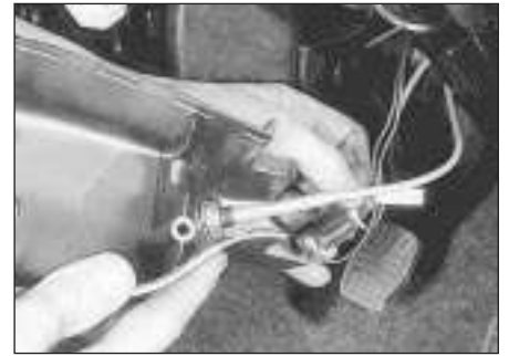
10.7 Choke warning switch and cable connection to steering column cowl
