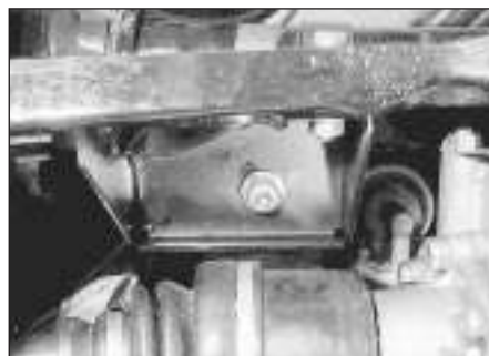
3.29c Left-hand rear engine mounting (from below)
