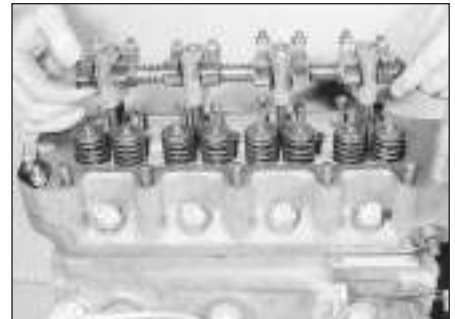
4.4 Removing the rocker shaft assembly
