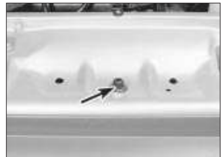
5.3c Radiator upper left-hand mounting (arrowed)
