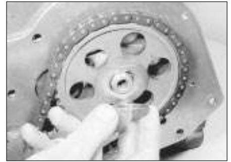
6.10 Removing the camshaft gear retaining nut
