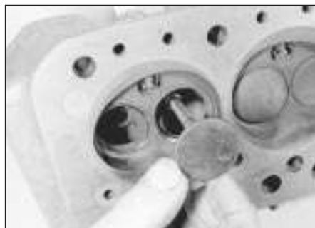
6.3a Removing an inlet valve
