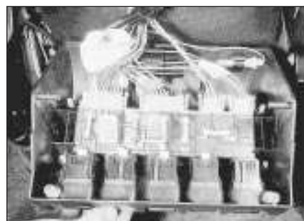
2.1b Switch board and fuses - early models
