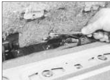
11.6b Removing the rear heater mounting bolt
