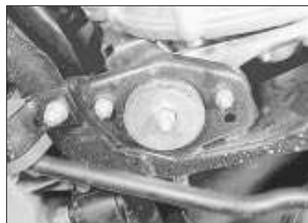
3.28e Right-hand front engine mounting (from below)
