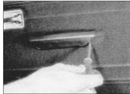
15.1b Removing the armrest
