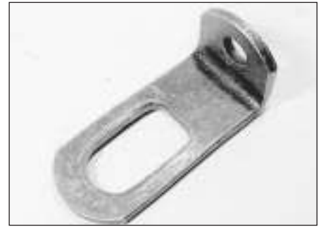
3.27 Suitable engine lifting bracket
