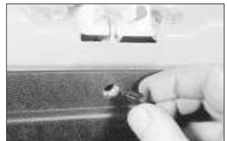
22.4 Removing a tailgate trim panel fastener
