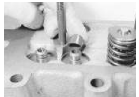
6.2 Removing an inlet valve guide oil seal (1275 cc engine)
