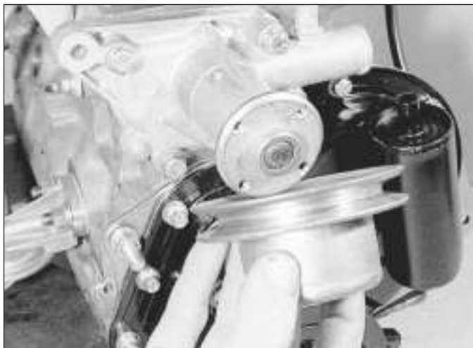
7.4 Removing the water pump pulley
