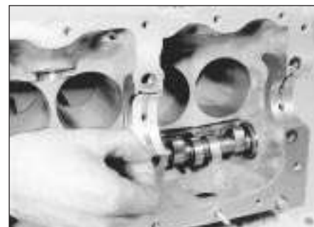
10.8 Removing a main bearing shell
