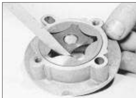
8.9d . . . rotor lobe clearance (central) . . .
