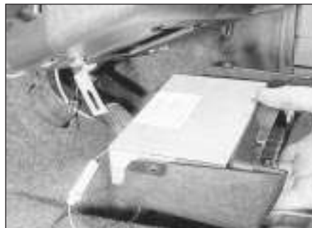
29.4 Removing the radio
