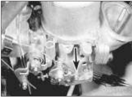
10.2 Choke cable - inner cable and clamp pin
