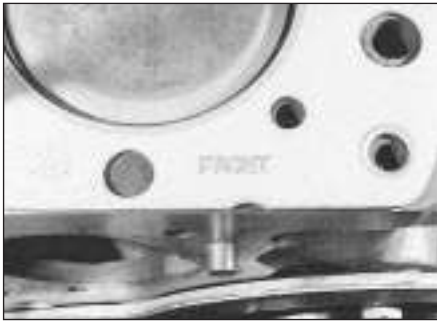
4.9 Cylinder head gasket "FRONT" marking
