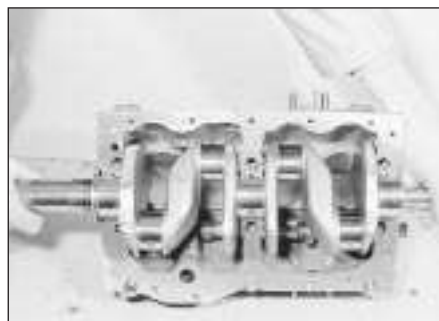
10.7 Removing the crankshaft
