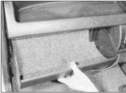
29.2 Removing the glovebox
