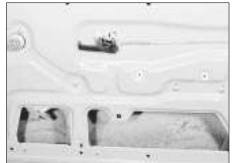
17.5a Inner door handle and rod
