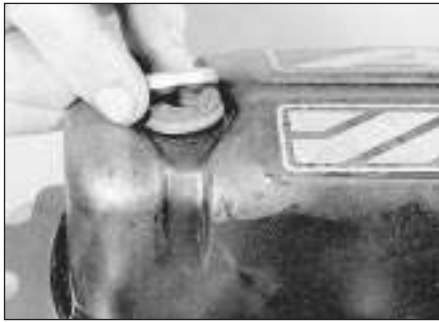
4.1a Rocker cover washer and seal
