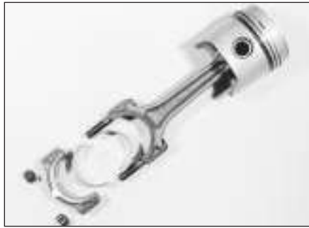
9.10 Piston and connecting rod components (1275 cc engine)
