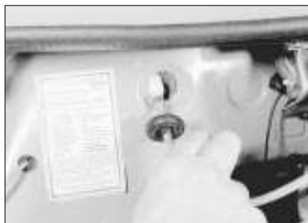
18.3 Removing the speedometer cable from the head
