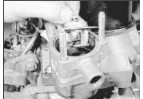
6.4 Removing the thermostat
