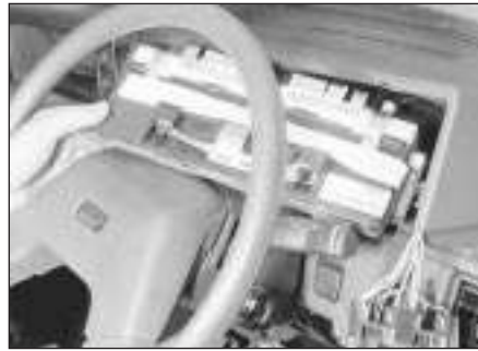
14.19b Removing the instrument panel
