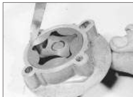
8.9c . . . outer rotor clearance . . .
