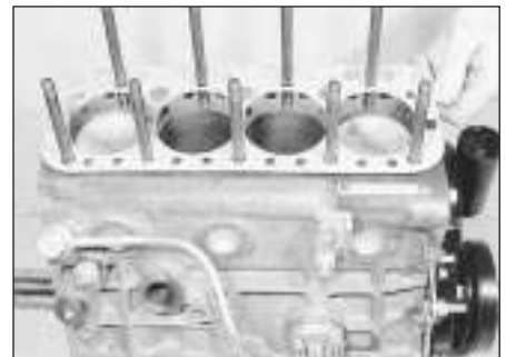
4.7 Removing the cylinder head gasket (1275 cc engine)
