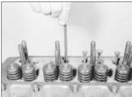
4.5 Removing a pushrod
