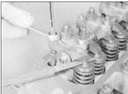
5.4 Checking the valve clearances
