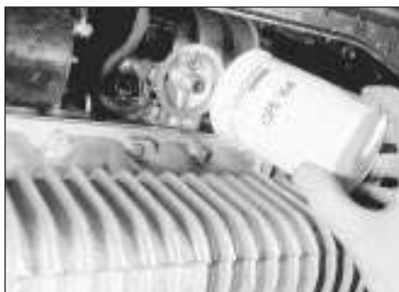
3.7b Removing the oil filter cartridge
