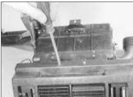
11.8b Removing the heater cover panel
