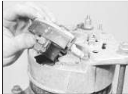
13.3B Withdraw the regulator and brushbox . . .
