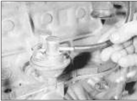
5.6a Disconnecting the feed pipe from the fuel pump
