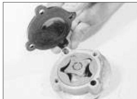
8.5 Removing the oil pump cover
