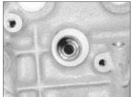
7.21c Installed position of the distributor driveshaft
