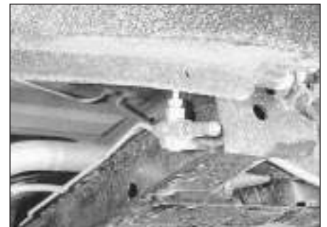
10.8 Rear Hydragas interconnecting pipe and three-way connector
