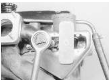
19.4a Remove the retaining nuts . . .
