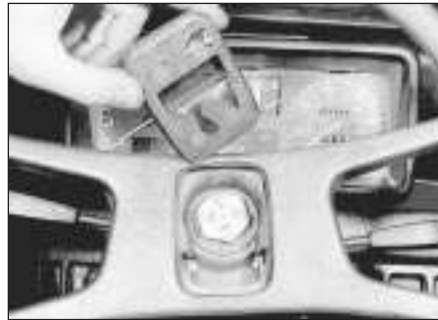
14.2 Removing the steering wheel central cover
