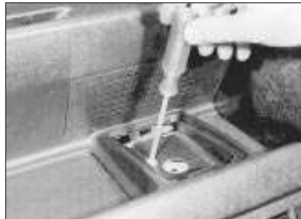
29.6b Removing the centre facia retaining screw
