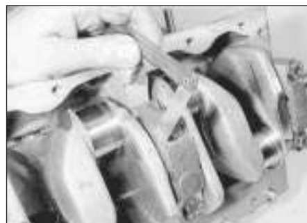
10.5 Checking the crankshaft endfloat with a feeler blade
