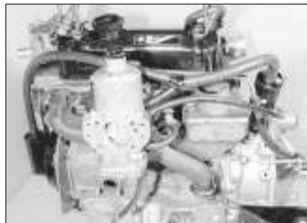
8.1 Showing the location of the crankcase ventilation hoses (1275 cc engine)
