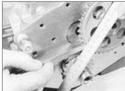
6.19a Checking the timing gear alignment by comparing the camshaft gear teeth-to-rule dimension...
