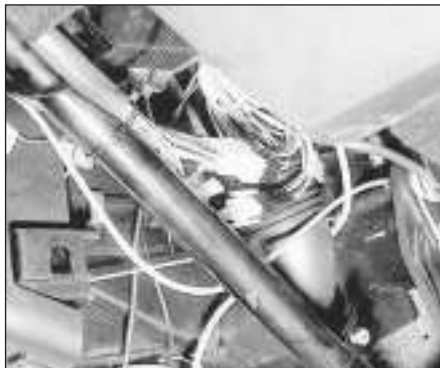
15.3 Steering column and wiring multi-plug
