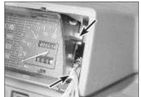
14.18 Instrument panel side screws (arrowed)
