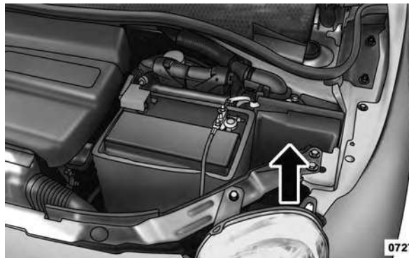
Front Distribution Unit
