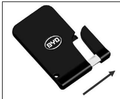
How to use the mechanical key in the card smart key
