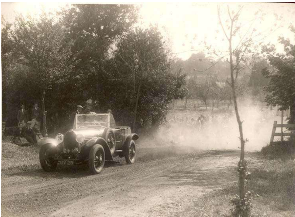
Pic: The chassis is shortened 19 inch; the rear doors have been removed, here pictured at the BOC Chalfont St Giles Hillclimb in 1934 where it became the fastest sports car (Photo W.J. Brunell courtesy of Moyra James-Bear)
