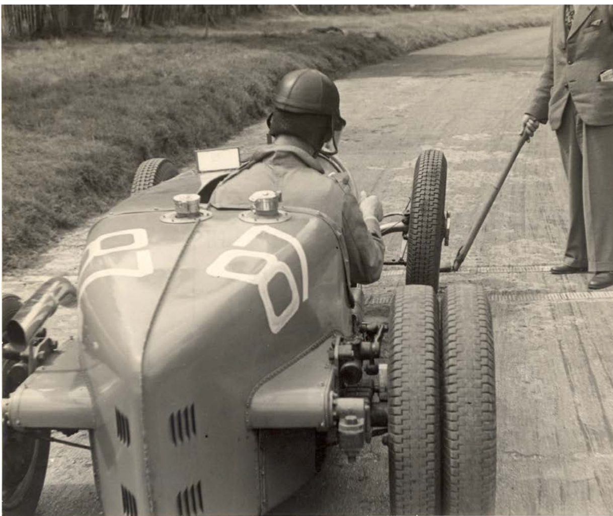
Fig: Kenneth Bear in 59121, this time with the 4 wheels on the rear, a feature specific for Bear, which he also had on the Bear Special and on 55155 (Photo courtesy of Moyra James- Bear)
