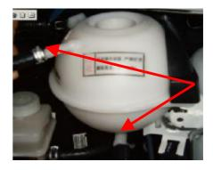
——To pry out the protecting hood of expansion reservoir by using a screw drive.
