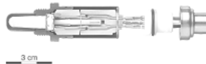
Interior structure of oxygen sensor
