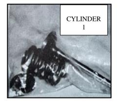
Put one set of valve, valve cotter, spring and spring seat into one plastic bag, each of which shall be tagged with numbers for installing them back to the original position.
