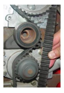
Hold the middle of the right belt that is away from both the crankshaft gear and camshaft gear with the thumb and the first finger. If the tension of the belt is up to standard, the belt shall be able to twist at  $90^{\circ}$  at this point.
