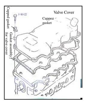
Remove the valve cover and gasket assembly. Take the sheet gasket out.
