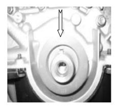
Check whether the TDC indicator on the cam shaft gear lines up with that on the front end of cylinder head. If not, rotate the crank shaft clockwise in one full circle to make them line up with each other. At this time, the engine is in the position of TDC of the first cylinder.
