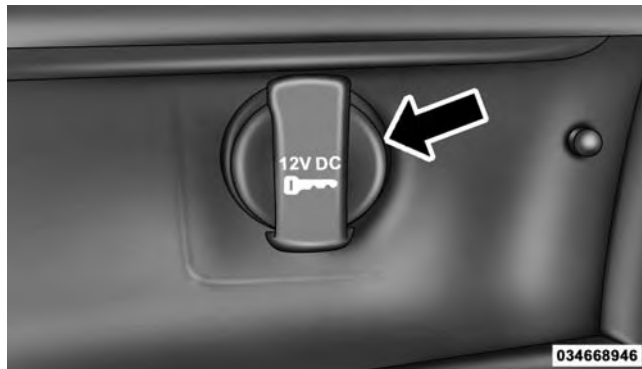
Front Power Outlet
