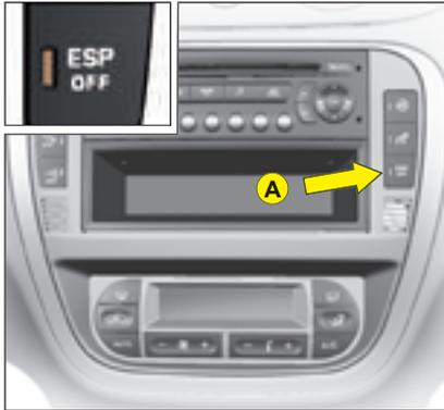
This system is associated with the ABS and in addition to the ABS. In the event of a loss of control of the vehicle by the driver, the ESP system acts automatically on one or more wheels and also on the engine to bring the vehicle back on trajectory.
