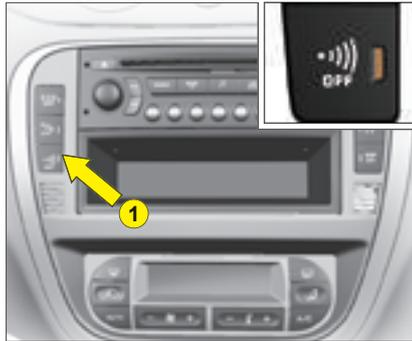
Your vehicle may be equipped with an ANTI-INTRUSION ALARM. This provides:
