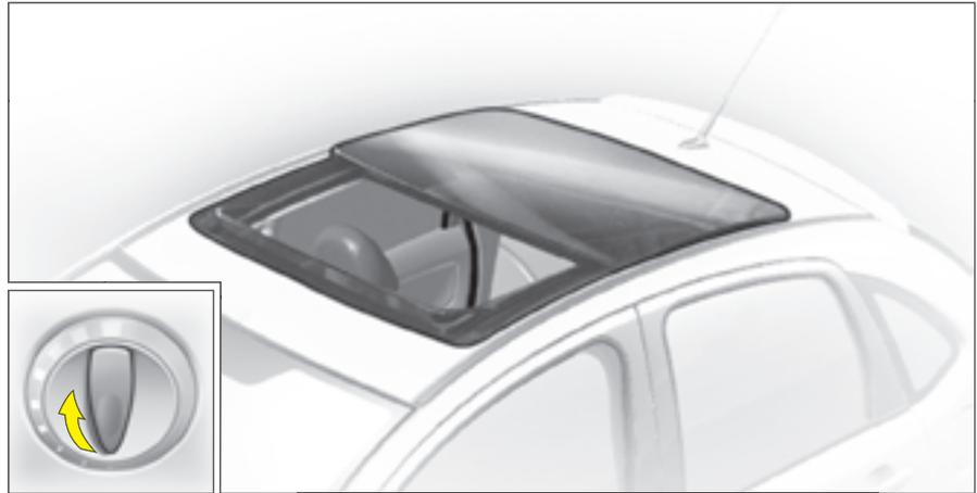
It is controlled electrically and sequentially, by a rotary switch with nine opening positions located on the roof lining between the two front sun visors.
