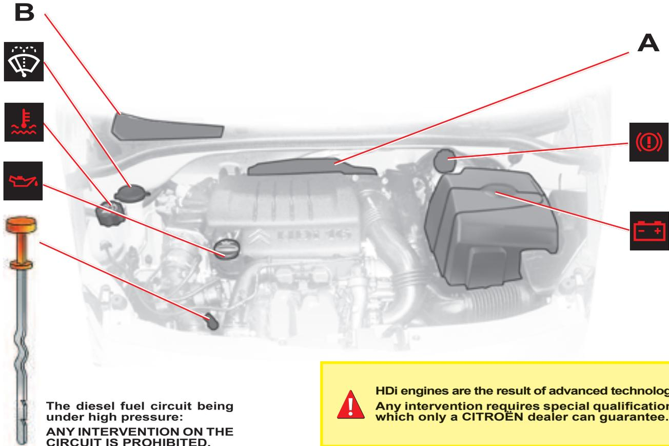
The diesel fuel circuit being under high pressure:
