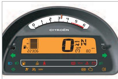
When the ignition is switched on, the orange and red warning lamps light up.
