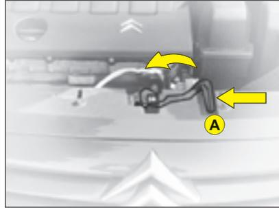
Operate the lever **A**, located above the grille, to the right of the chevrons, then lift.
