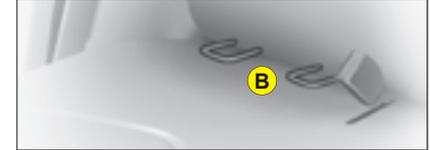
Two rings **B**, located between the backrest and the seat cushion, allow a child seat to be fitted.
