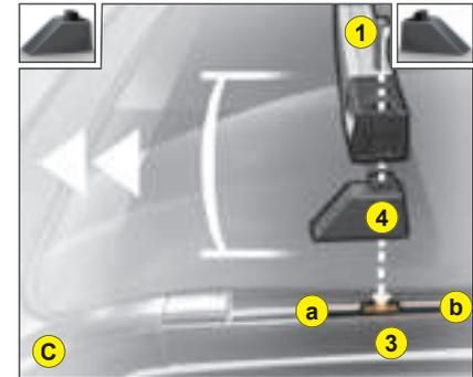
To install the transversal roof bars, use the accessories that are to be found in the stowage drawer underneath the front seat, then:
