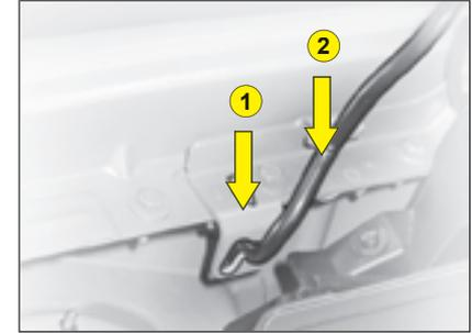
**Bonnet stay:** Unclip and swivel the strut, to insert it in notch **1**, then in notch **2**.
