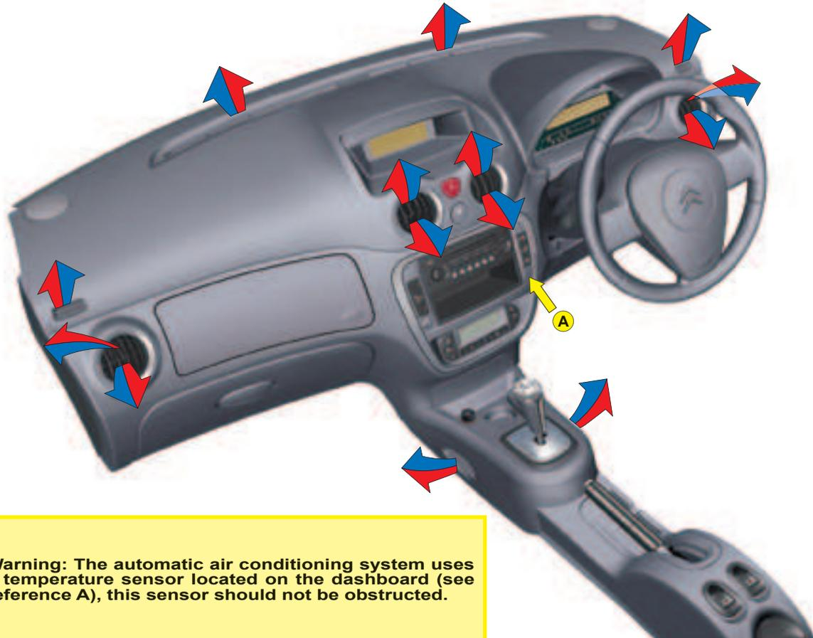
**Warning:** The automatic air conditioning system uses a temperature sensor located on the dashboard (see reference A), this sensor should not be obstructed.
