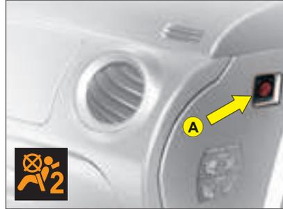
1. With the ignition off, insert the key in switch **A**.
