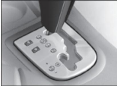
**The engine can only be started when the lever is at position P or N.**
