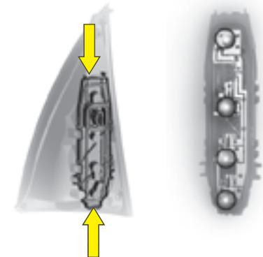
Refit the assembly after replacing the bulb.
