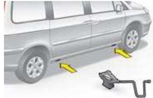
**Never get under a jacked up vehicle unless it is correctly supported by axle stands. The jack is designed specifically for your vehicle, do not use it for other applications.**
