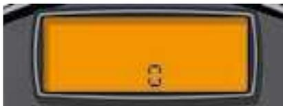
**Note:** the maintenance spanner will come on, and the display will read “0” if the maximum length of time between services is attained before the mileage limit is reached.
