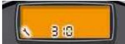
A few seconds after that, the engine oil level indicator is displayed, then the total mileage recorder resumes its normal role and the maintenance symbol remains lit up.
