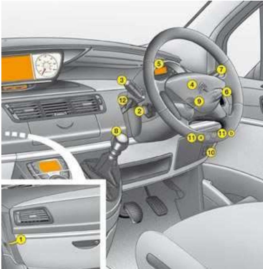
1. Volumetric alarm deactivation switch.
