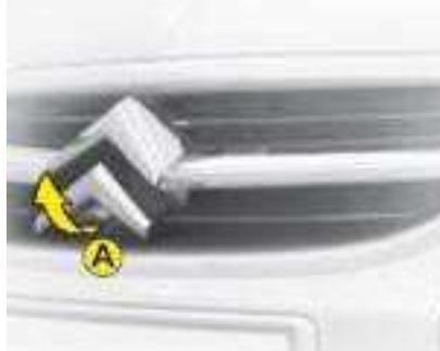
Lift latch **A**, located under the centre forward edge of the bonnet and pull the bonnet up.
