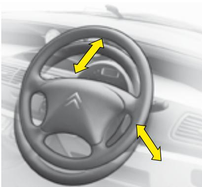
Both the height and reach of the steering wheel can be adjusted.
