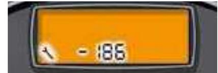
A few seconds after you have switched on the ignition, the total mileage recorder returns to its normal operation and the maintenance symbol remains illuminated.
