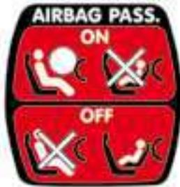
III The front passenger's airbag can be deactivated.
