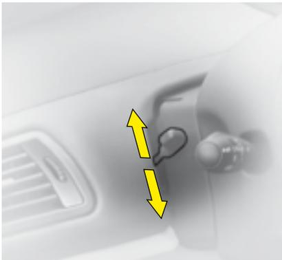
Unlock the steering wheel by pushing the control downwards.
