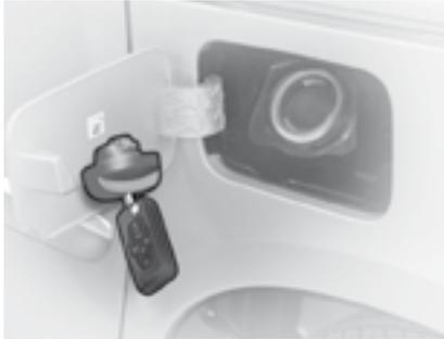
To open the fuel flap, pull at its notched edge. A label showing the correct fuel quality will be found on the inside of the flap (See “Fuel quality”).
