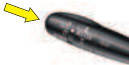
Press on the end of the lighting control stalk. Activation of the function is confirmed by a beep and by the opening of a window on the display.
