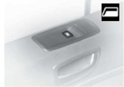
The front passenger's electric window is operated from the control located on the door.
