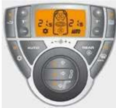
Automatic with separate regulation. Press, AUTO is displayed, this is the normal operating mode.
