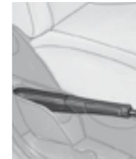
Pull the button on the end of the parking brake lever forwards. The parking brake lever goes back down. You can now rotate the seat. To resume normal operation of the parking brake, pull the lever upwards until it clicks into place.
