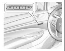
The SET, "1," "2," and (Exit) buttons on the driver door are used to manually save and recall memory settings for the driver seat, outside mirrors, and power tilt and telescoping steering column.
