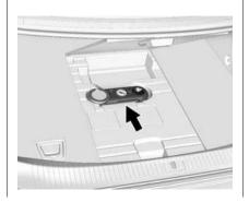
3. Remove the tire sealant and compressor kit.
