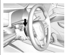
Regen on Demand allows increased deceleration by pressing and holding either of the steering wheel paddle switches. It works in D (Drive) and L (Low). The accelerator pedal must be fully released for it to work.
