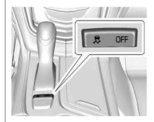
The button for TCS and StabiliTrak is on the center console, behind the shift lever.
