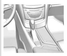
**P (Park):** This position locks the front wheels. It is the best position to use when starting the propulsion system because the vehicle cannot move easily.
