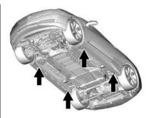
The front lifting points can be accessed from either side of the vehicle, behind the front tires.
