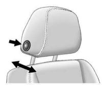
To adjust the head restraint forward, grasp the head restraint and pull forward until the desired locking position is reached.
