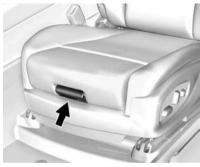
If equipped, adjust the manual leg extension by pulling up on the lever, and then pulling or pushing on the support to lengthen or shorten it. Release the lever to lock it in place.
