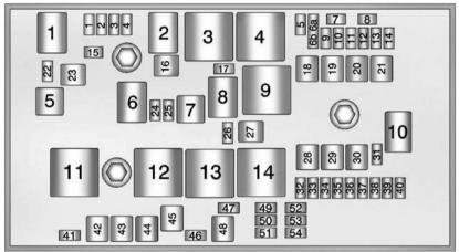
**Engine Compartment Fuse Block**
