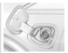
Plug in the vehicle plug of the charge cord into the charge port on the vehicle. Verify that the charging status indicator illuminates on top of the instrument panel and a horn chirp occurs. See Charging Status Feedback on page 9-59.
