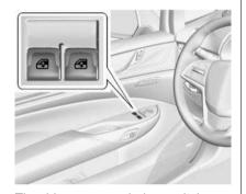
The driver power window switches control all the windows. The passenger switch only controls that window.
