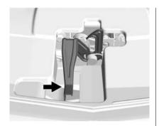
Go to the front of the vehicle and locate the secondary release lever under the front center of the hood. Push the secondary hood release lever to the right to disengage.
