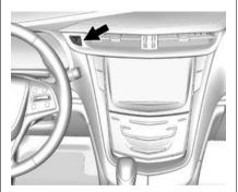
The vehicle has an electronic pushbutton start. The POWER  $\circlearrowleft$  button light is on steady when in
