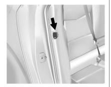
Remove the guide from its storage pocket on the side of the seat.
