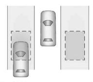
The SBZA sensor covers a zone of approximately one lane over from both sides of the vehicle, or 3.5 m
