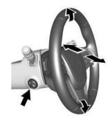
Press the control to move the tilt and telescoping steering wheel up and down or forward and rearward.
