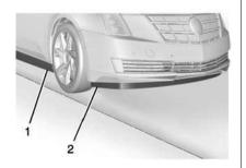
If the vehicle is parked off the shoulder of the road, at an angle that it cannot be pulled onto a flatbed, a hook/chain can be placed into either of the front torque box openings to pull the vehicle onto a flat surface. Make sure that the chains do not come in contact with the rocker panel (1) or the front fascia (2).
