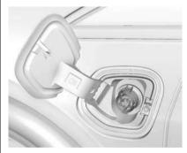
5. Plug in the vehicle plug of the charge cord into the charge port on the vehicle. Verify that the charging status indicator illuminates on top of the instrument panel and a horn chirp occurs. See Charaina Status Feedback on page 9-59.
