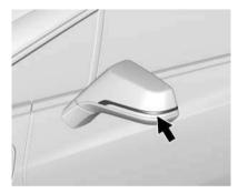
The outside rear view mirrors are equipped with green LEDs used to indicate high voltage battery system charging status. The OSRVM CSI indicates the following:
