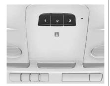
This system provides a way to replace up to three remote control transmitters used to activate devices such as garage door openers, security systems, and home automation devices.
