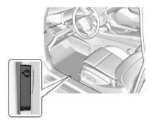
From inside the vehicle, pull the driver door manual release lever.
