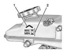
With the vehicle not running for at least one minute, the maximum fluid level (1) is at the top of the reservoir body. With the vehicle running, the fluid level should be in the proper operating range (2) between the MIN and MAX marks. If it is not, have the brake hydraulic system checked to see if there is a leak.
