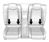
Lift the flap below the label to access the anchors.
