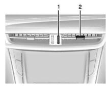
Use the thumbwheels (1) near the air vents to open or close off the airflow.
