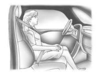
If a person of adult size is sitting in the front outboard passenger seat, but the off indicator is lit, it could be because that person is not sitting properly in the seat. Use the following steps to allow the system to detect that person and enable the front outboard passenger frontal airbag and passenger knee airbag:
