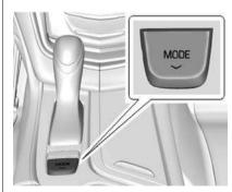
Press the MODE switch to display selectable drive modes in the Driver Information Center (DIC). Continue pressing to scroll through the modes.
