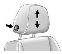
Pull the head restraint up to raise it. Try to move the head restraint to make sure that it is locked in place. To lower the head restraint, press the button located on the side of the head restraint, and push the head restraint down. Try to move the head restraint after the button is released to make sure that it is locked in place.
