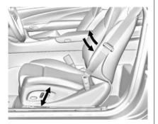
If equipped, to adjust the bolster support:
