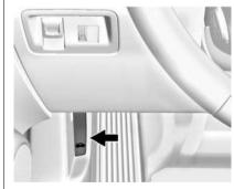
Pull the release handle with this symbol. It is below the instrument panel outboard of the steering wheel.
