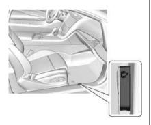
From inside the vehicle, pull the passenger door manual release lever.
