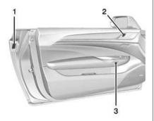
For Keyless Access, the RKE transmitter must be within 1 m (3 ft) of the door handle sensor (1). Grip and press to open.
