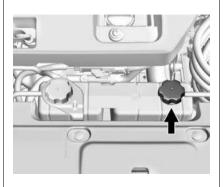
Check to see if coolant is visible in the power electronics and charger modules coolant reservoir. If coolant is visible but the coolant level is below the cold fill line, there could be a leak in the cooling system.
