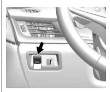
The vehicle has an Electric Parking Brake (EPB). The switch is to the left of the steering wheel. The EPB can always be activated, even if the vehicle is off. To prevent draining the 12-volt battery, avoid repeated cycles of the EPB system when the vehicle is off.
