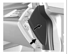
The right instrument panel fuse block is on the right side end of the instrument panel, behind the end cap. To access the fuses, insert a plastic tool between the end panel and the instrument panel, and carefully release the end cap retaining clips. When all clips are released, remove the panel.
