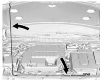
Lift the hood and release the hood prop rod from its retainer above the radiator support.
