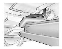
When lifting the vehicle from the front, place the service jack directly under one of the cradle mounts.
