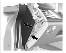
The left instrument panel fuse block is on the left side end of the instrument panel, behind the end cap. To access the fuses, insert a plastic tool between the end panel and the instrument panel, and carefully release the end cap retaining clips. When all clips are released, remove the panel.
