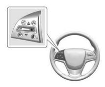
(On/Off): Press to turn the system on or off. A white adaptive cruise control indicator comes on.
