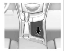
Cupholders in the front center console have a power retractable cover. Push the handle forward to express open. Pull the handle rearward to express close.
