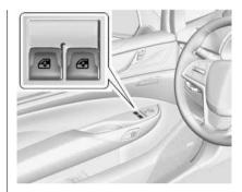
The power window switches are on the driver door. The passenger door also has a window switch for only that window.
