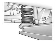
When lifting the vehicle from the rear, place the service jack directly under one of the spring seats.
