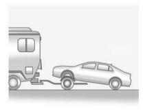
The vehicle can be towed from the front using a dolly. To tow the vehicle using a dolly:
