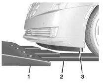
Ramps (2) are required for the front fascia (3) to clear the flatbed (1). The ramp height should be approximately 102 mm (4 in). Lower the flatbed onto the set of ramps.
