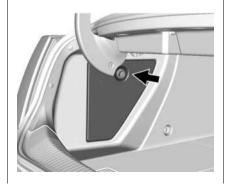
There are two rear compartment fuse blocks, located on the left side of the trunk behind a cover.
