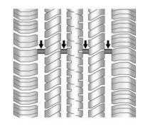
Treadwear indicators are one way to tell when it is time for new tires. Treadwear indicators appear when the tires have only 1.6 mm (1/16 in) or less of tread remaining. See *Tire Inspection on page 10-54* and *Tire Rotation on page 10-54*.
