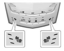
The buttons are near the climate controls on the center stack. To operate, the ignition must be in ON/RUN/START.
