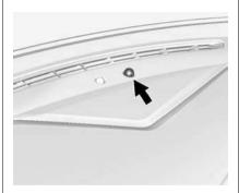
The solar sensor monitors the solar heat.
