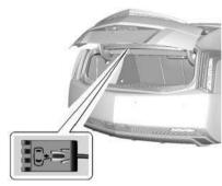
From outside the vehicle, open the trunk and pull the manual door release lever.
