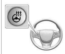
(Heated Steering Wheel): Press to turn the heated steering wheel on or off. A light next to the button displays when the feature is turned on.
