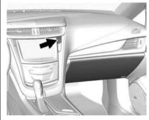
To open, press the button. Close the glove box manually.
