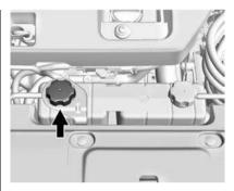
Check to see if coolant is visible in the high voltage battery coolant reservoir. If coolant is visible but the coolant level is below the cold fill line, there could be a leak in the cooling system.
