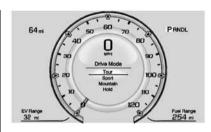
Highlight either the Mountain, Sport, or Hold Mode, then release the MODE switch. After three seconds. the new drive mode will become active
