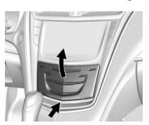
Touch the bottom of the climate control system panel until the door automatically starts to open. There is a USB port inside. See the infotainment manual.
