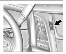
Press the top of the switch to move the pedals closer to your body. Press the bottom of the switch to move the pedals away.
