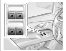
The windows work when the vehicle is in ON/RUN, ACC/ACCESSORY, or when Retained Accessory Power (RAP) is active. See *Retained Accessory Power (RAP)* ⇒ 209.
