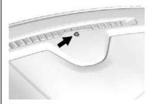
The solar sensor, on top of the instrument panel near the windshield, monitors the solar heat.
