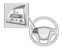
(5): Press to turn the system on and off. A white indicator appears in the instrument cluster when cruise is turned on.
