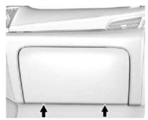
Before opening the glove box, remove the two lower screws (out of view).
