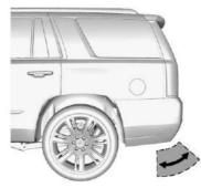
To operate, move your foot in a forward kicking motion under the center of the rear bumper, then pull it back
