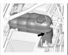
The coolant level should be at or above the FULL COLD mark. If it is not, there may be a leak in the cooling system.
