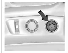
If equipped, use the transfer case knob next to the steering wheel to shift into and out of four-wheel drive.
