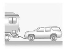
Only dinghy tow four-wheel-drive vehicles with a two-speed transfer case that have an N (Neutral) and a Four-Wheel Drive Low  $(4 \downarrow)$  setting.
