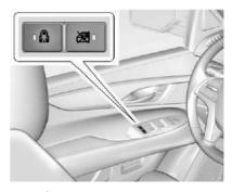
Press at to activate the safety locks on the rear doors. The indicator light comes on when activated.
