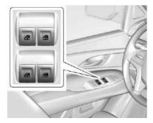
The windows work when the vehicle is in ON/RUN, ACC/ACCESSORY, or when Retained Accessory Power (RAP) is active. See *Retained Accessory Power (RAP)* ⇒ 209.
