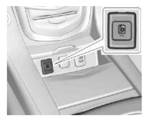
If equipped, press to turn on the cooled compartment inside the center console storage.
