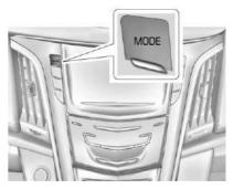
The vehicle is normally in Tour Mode. Sport Mode and Snow/Ice Mode are engaged when the Magnetic Ride Control MODE button on the center stack is pressed. Press the button to select the desired mode.
