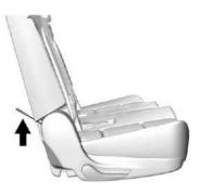
Pull the strap on the bottom rear of the second row seat to release the seatback. The seatback will fold forward.
