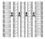
Treadwear indicators are one way to tell when it is time for new tires. Treadwear indicators appear when the tires have only 1.6 mm (1/16 in) or less of tread remaining. Some commercial truck tires may not have treadwear indicators. See *Tire Inspection*  $\Rightarrow$  313 and *Tire Rotation*  $\Rightarrow$  313 for additional information.
