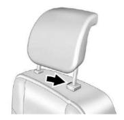
The third row seat head restraint can be lowered to allow for better visibility when the rear seat is unoccupied. To lower the head restraint, press the button located on the top of the seatback and push the head restraint down.
