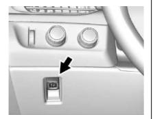
If equipped with an Electric Parking Brake (EPB), the switch is to the left of the steering wheel on the instrument panel, below the exterior lamp controls. The EPB can always be activated, even if the ignition is off. To prevent draining the battery, avoid repeated cycles of the EPB when the engine is not running.
