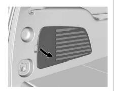
The rear compartment fuse block is behind the access panel on the left side of the compartment.
