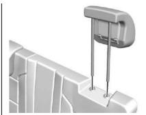
rearward, insert the head restraint posts into the holes in the top of the seatback.
