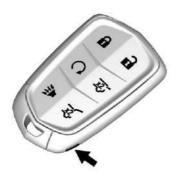
Press the button on the side of the transmitter near the bottom and pull the key out.
