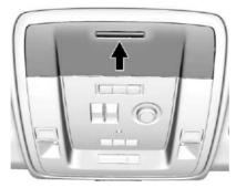
If equipped, sunglasses storage is on the overhead console. Press the fixed button on the cover and release to access. There may be a child-view mirror located within the sunglasses bin. Release the bin and then push up halfway to secure in position.
