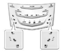
The buttons are near the climate controls on the center stack. To operate, the engine must be running.
