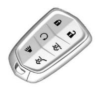
$\mathbf{\Omega}$ : If equipped, press and release  $\widehat{\mathbf{Q}}$ , then immediately press and hold  $\mathbf{\Omega}$  until the turn signals flash or for at least four seconds. The engine may be started from outside the vehicle using the RKE transmitter. See *Remote Vehicle Start*  $\Rightarrow$  36.
