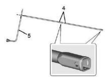
Assemble the two jack handle extensions (4) and wheel wrench (5).
