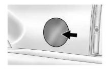
Locate the fuel door. The fuel gauge has an arrow to indicate the side of the vehicle the fuel door is on. If equipped, the fuel door is locked when the vehicle doors are locked.
