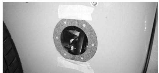
Figure 185: Gasket positioned on back panel
