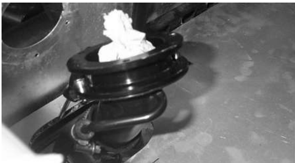
Figure 187: Spacer fitted to filler neck
