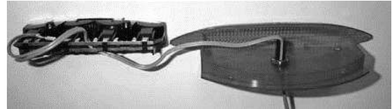
Figure 193: Wire routing through light unit
