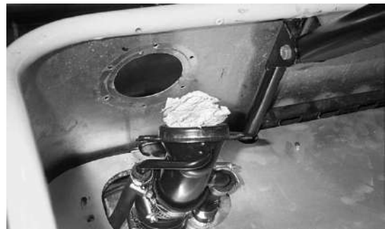
Figure 184: Old filler boss removed
