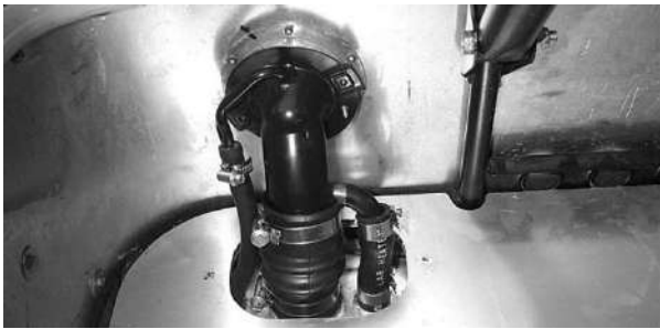
Figure 182: Filler cover and boot carpet removed
