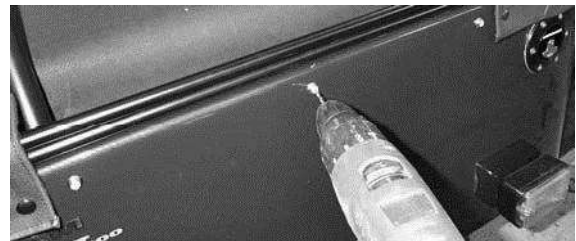
Figure 191: Drilling central popper on SV
