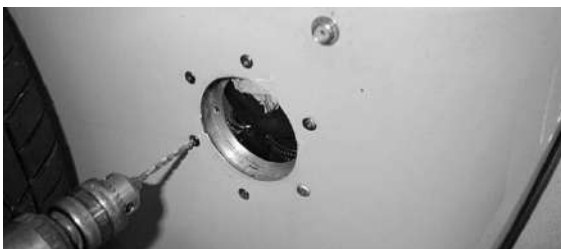
Figure 183: Drill out the six rivets
