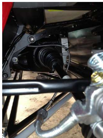
Figure 132: Handbrake cable routing S3 (non-adjustable side)
