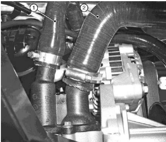
Figure 48: Bottom hose engine connection (viewed from bellow)
