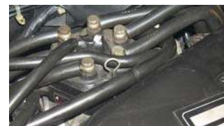
Figure 38 Unacceptable adj. plug
