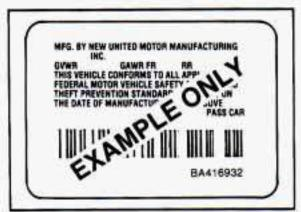
The other label is the Certification label, found on the rear edge of the driver's door. It tells you the gross weight capacity of your vehicle, called the GVWR (Gross Vehicle Weight Rating). The GVWR includes the weight of the vehicle, all occupants, fuel and cargo. Never exceed the GVWR for your vehicle, or the Gross Axle Weight Rating (GAWR) for either the front or rear axle.
