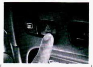
Press the button to make your front and rear turn signal lights flash on and off.
