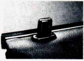
From the inside: To lock the door, push down the button on the door.
