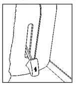
Pull up on the release lever labeled 1 and then pull up on the seatback until the seatback locks into the upright position.
