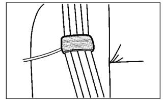
3. Be sure that the belt is not twisted and it lies flat. The guide must be on top of the belt.
