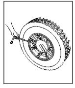
To remove the center cap, place the flat end of the wheel wrench in the slot on the wheel and carefully pry the center cap out.
