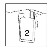
3. To unlatch the rear of the seat from the floor, pull up on the release lever labeled 2, at the rear of the seat, and lift the rear of the seat up from the floor.
