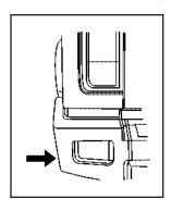
Locate the affected taillamp which is behind and under the bumper.
