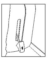
5. Pull up on the release lever labeled 1 and then pull up on the seatback until the seatback locks into the upright position.
