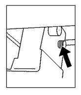
Once the knob is torqued, install the cotter pin through the hole in the end of the knob's threaded shaft.
