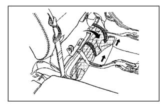
Remove the strap from the seat rail. Then carefully slide the tool bag out from under the seat rail as shown. 4. Open the tool bag. You will find the following tools needed to remove the spare tire and flat tire:
