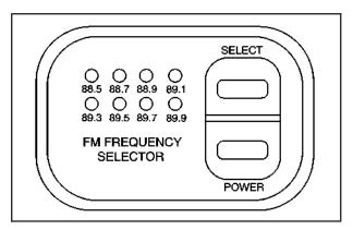
**SELECT:** Press this button on the FM Modulator control to match the frequency selected on the radio.
