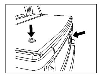
Your tonneau cover will have two lock cylinders on it. One lock cylinder is to secure the cover closed and the other lock cylinder will allow you to secure the tailgate closed.
