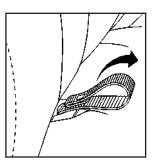
Pull up on the strap loop located at the rear of the seat cushion and pull the seat cushion up and fold it forward.
