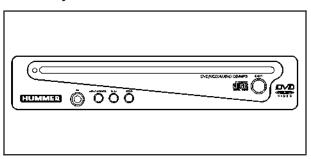
**AV INPUT (Audio/Video Input Jack):** The audio/video input jack allows viewing of auxiliary sources such as portable DVD players, game stations, or video cameras, on each monitor individually.
