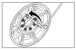
Turn the wheel wrench counterclockwise to loosen the wheel nuts. Do not remove them yet.You will now need to jack the vehicle up using the
