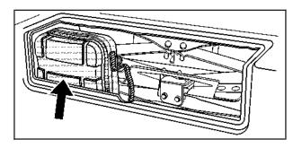
Remove the tool kit/first aid kit to gain access to the tire changing equipment.
