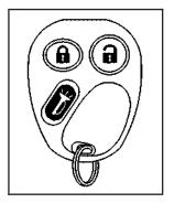
(Unlock): Press this button once to unlock the driver's door. The interior lamps will come on. Pressing unlock again within three seconds will cause the remaining doors to unlock.
