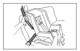
5. To tighten the belt, push down on the child restraint, pull the shoulder portion of the belt to tighten the lap portion of the belt and feed the shoulder belt back into the retractor. If you are using a forward-facing child restraint, you may find it helpful to use your knee to push down on the child restraint as you tighten the belt.
