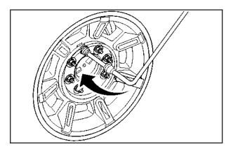
Use the wheel wrench and wheel wrench extension for the to tighten the nuts firmly. Try to move the tire back and forth slightly to be sure it is secure.
