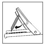
Remove the wheel blocks from the tool bag. Then, lift the wheel block as shown to lock it into place.
