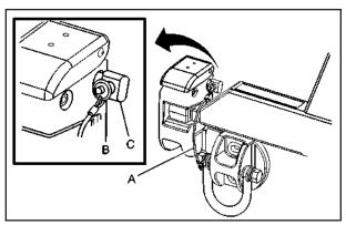
Press the button on the pin (B), which is attached to the cable (A), to remove the pin from the latch nut (C).
