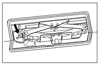
Release the jack by turning the end of the jack handle counterclockwise.
