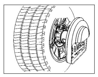
6. Slide the license plate holder onto the spare or flat tire. Secure it from the back of the tire carrier with the wing nut. If you choose not to reinstall the spare or flat tire on the vehicle, you will still need to reinstall the license plate holder on the spare tire carrier.
