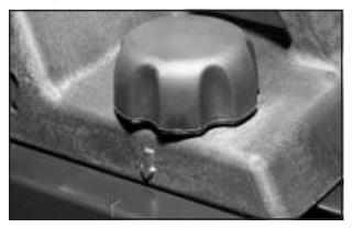
Loosen the lock knobs on the crossrail supports by turning the knobs counterclockwise. Only loosen them enough to allow the crossrails to slide easily.
