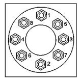
14. Tighten the nuts firmly in a crisscross sequence as shown by turning the wheel wrench with the wheel wrench extender clockwise.
