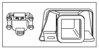
Your vehicle is equipped with a trailer towing harness. This harness with a seven-pin universal heavy-duty trailer connector is attached to a bracket on the hitch platform.
