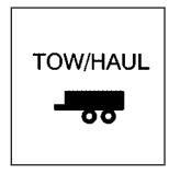
Press the button on the instrument panel to the right of the steering wheel to enable the tow/haul mode.
