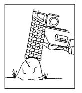
Do not straddle large rocks; drive over them, letting the tire cover the rock. The tread of the tire is thicker and tougher than the sidewall of the tire and is more resilient to impact than underbody components.
