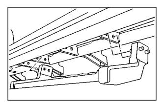
Guide the pins on the side step brackets into the holes in the vehicle's rocker panel protector brackets.
