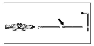
Rear Flat Tire: Assemble the jack together with the jack handle and the jack handle extensions. Press the retention clip on the jack handle extension (arrow) so it engages into the jack handle. Slide the wheel wrench onto the jack handle extension.
