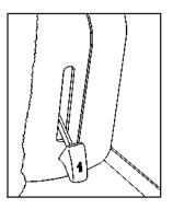
Fold the seatback forward onto the seat cushion by using the lever labeled 1. The seat cannot be removed unless the seatback is folded.
