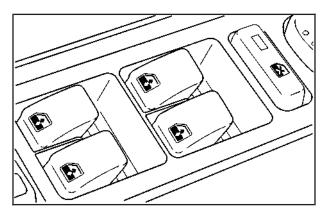
A power window switch is located on the armrest of each side door. The switches operate while the ignition is in RUN or ACCESSORY or while Retained Accessory Power (RAP) is active. See *Retained Accessory Power (RAP)* on page 2-27.
