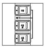
The transfer case buttons are located to the right of the instrument panel cluster. Use these switches to shift into and out of the different Full-Time Four-Wheel Drive modes.
