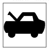
Pull the handle with this symbol on it. It is located inside the vehicle to the lower left of the steering column.
