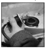
Turn the bulb socket counterclockwise and remove it from the lamp housing.
