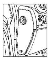
The fuse block access door is located on the driver's side edge of the instrument panel. Pull off the cover to access the fuse block.
