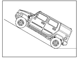
Design specifications required a minimum gradeability of 60% (31°) slope, with the vehicle fully loaded, on high friction surfaces at 6 mph (9.7 km/h). The vehicle is expected to traverse this grade only for short durations. Never stop and idle the vehicle or park it on this grade.
