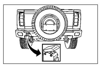
Lift up on the latch on the left side of the vehicle to release the spare tire carrier from the vehicle. The handle will stay in the raised position until the spare tire carrier is closed and latched properly.
