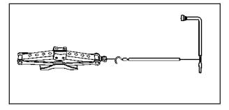
Front Flat Tire: Attach the jack handle with the hook end connected to the u-hook/clevis on the jack. Slide the wheel wrench onto the jack handle extension.
