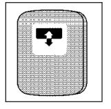
The vehicle may have a power sliding sunroof. The ignition must be on or in the accessory position, or Retained Accessory Power (RAP) must be active.
