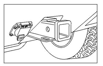
Connect the adapter with the tab pointing up. The flip cap on the vehicle's seven-wire harness will lock onto the tab (see arrow in the previous graphic) and help hold the adapter in place. Plug the four-way round pin connector onto the adapter.
