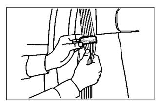
2. Place the guide over the belt and insert the two edges of the belt into the slots of the guide.
