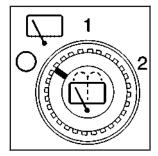
If your vehicle has a rear window washer/wiper, the control knob is located on the instrument panel to the left of the steering wheel.
