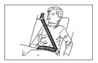
A safety belt that is not properly worn may not provide the protection needed in a crash. The person wearing the belt could be seriously injured. The shoulder belt should go over the shoulder and across the chest. These parts of the body are best able to take belt restraining forces.
