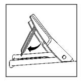
To use a wheel block, lift the wheel block as shown to lock it into place.
