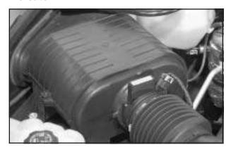
Loosen the screws on the engine air cleaner/filter cover.
