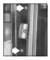
Remove the two screws from the rear lamp assembly and remove the rear lamp assembly.
