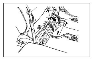
Remove the strap from the seat rail. Then carefully slide the tool bag out from under the seat rail as shown.
