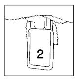
2. Unlatch the seat from the floor by pulling up on the lever labeled 2, located on the rear of the seat.
