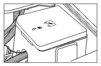
The underhood fuse block in the engine compartment is located on the driver's side of the vehicle near the battery. Lift the cover for access to the fuse/relay block.
