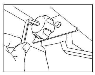
Hand-tighten the knob by turning it clockwise until it is seated against the rocker panel protector bracket and then tighten it to 10 lb ft (13.5 N•m) with the tool as shown.
