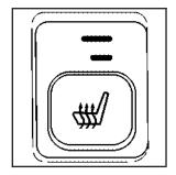
If your vehicle has this feature, the buttons used to control this feature are located on the back of the center console. The engine must be running for the heated seat feature to work.
