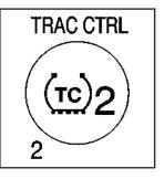
To enter this mode, press the TC2 button located on the instrument panel to the right of the steering wheel.
