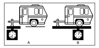
The trailer tongue weight (A) should be 10 percent to 15 percent of the total loaded trailer weight (B), up to a maximum of 500 lbs (227 kg) with a weight carrying hitch. The trailer tongue weight (A) should be 10 percent to 15 percent of the total loaded trailer weight (B), up to a maximum of 700 lbs (318 kg) with a weight distributing hitch.
