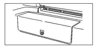
To remove the cover, unlock it and then pull the cover off.
