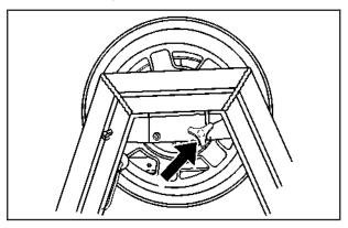
2. Unscrew the wing nut on the back of the tire carrier.
