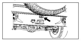
The camera uses a special lens. The distance of the image that appears on the screen differs from the actual distance. The area displayed by the camera is limited. The camera does not display objects which are close to either corner of the bumper or under the bumper. The spare tire and carrier extends rearward of the rear bumper. The area displayed on the screen may vary according to vehicle orientation or road conditions.
