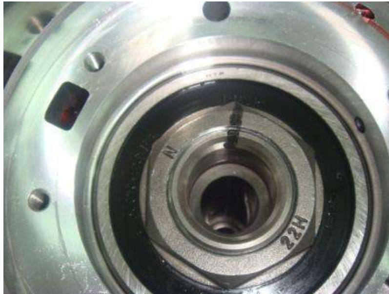
Fig. 7-1: Mark primary nut and shaft
