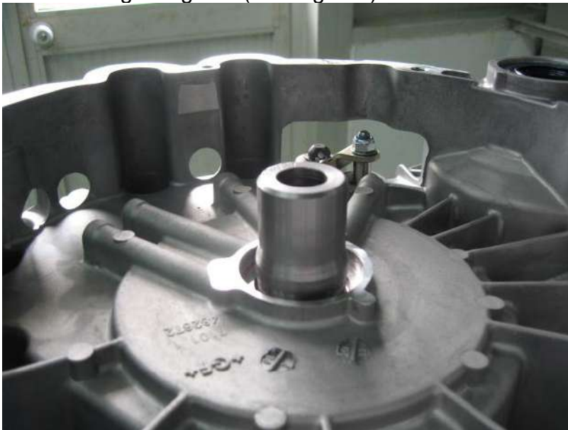
Fig. 3-2: Put special tool on input shaft (480129)
