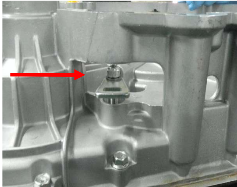
Shift lever NOT in P position, NOT OK for cable adjustment
