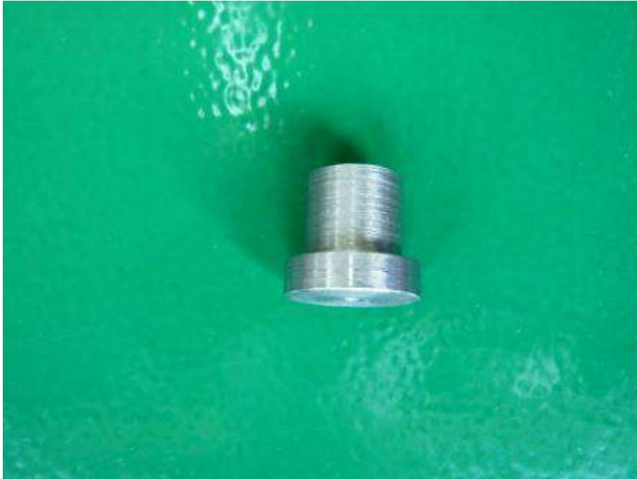
Plug – Primary bearing (drawing 480139)
