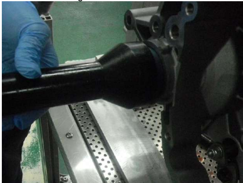
Fig. 2-2: Installing new seal with special tool
