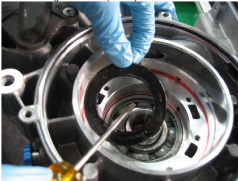
Fig. 7-2: Lever out seal from primary bearing
