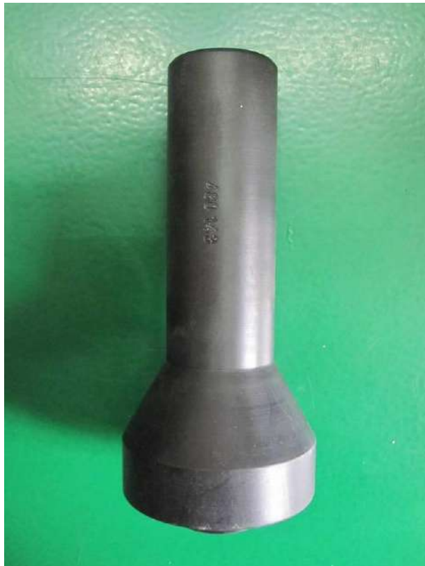
Stamp – oil seal differential (drawing 480143)
