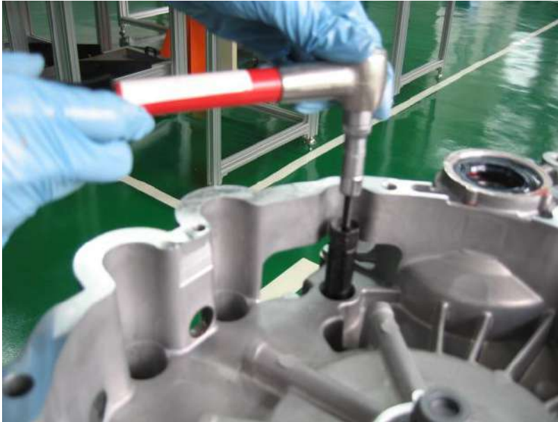
Fig. 4-3: Rotate screw to remove the seal
