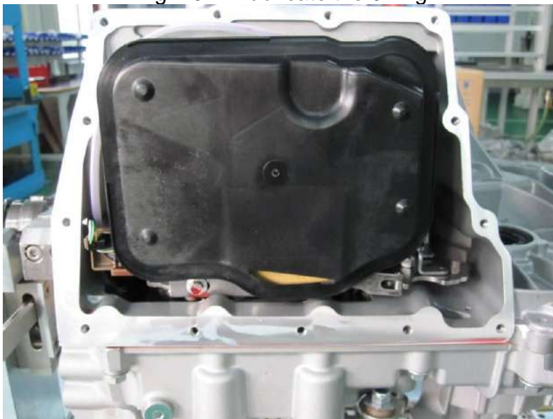
Fig. 10-2: Fix oil filter in position
