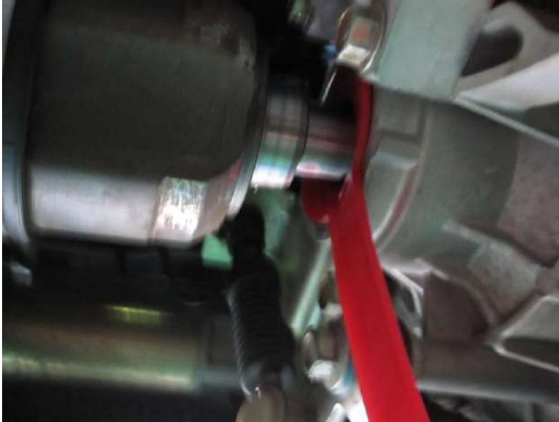
Fig. 1-3: Drive shaft inserted for 4cm
