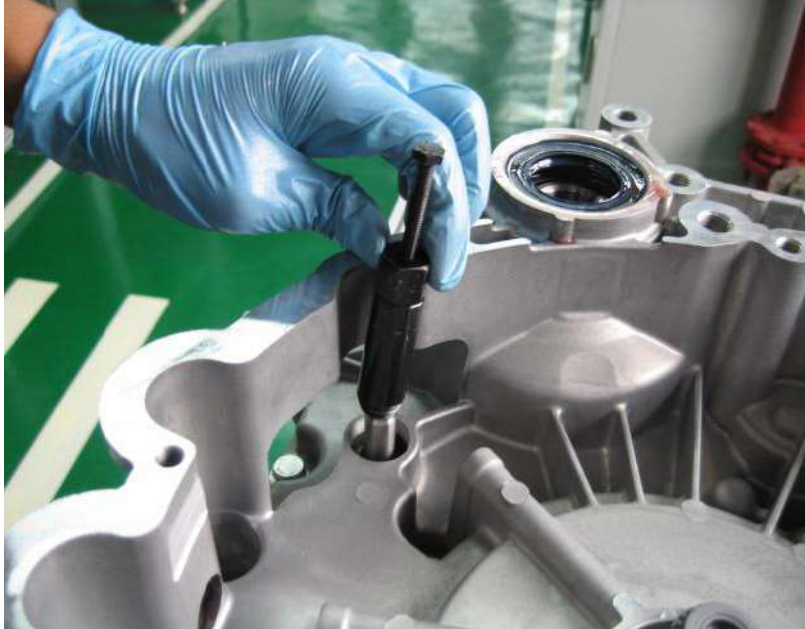
Fig. 4-1: Put special tool (480127) on shaft
