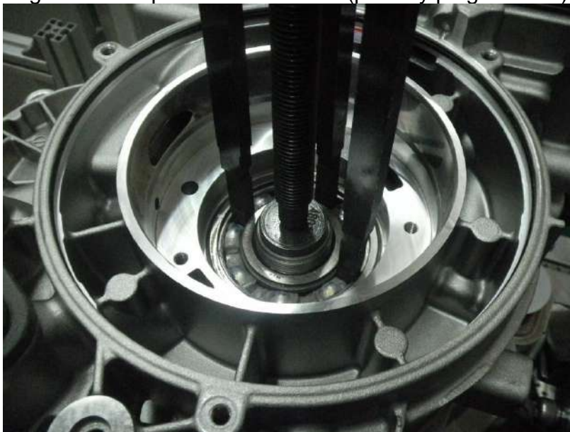
Fig. 7-4: Assemble bearing puller (480136)
