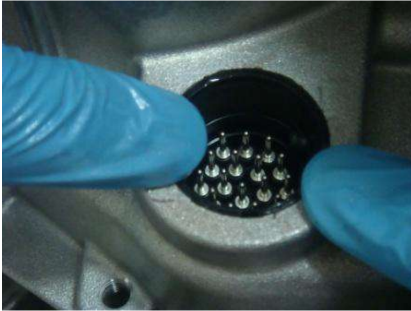
Fig. 15-2: Push main connector into the transmission
