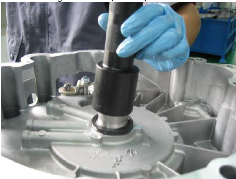
Fig. 3-4: Installing seal by special stamp (480130)
