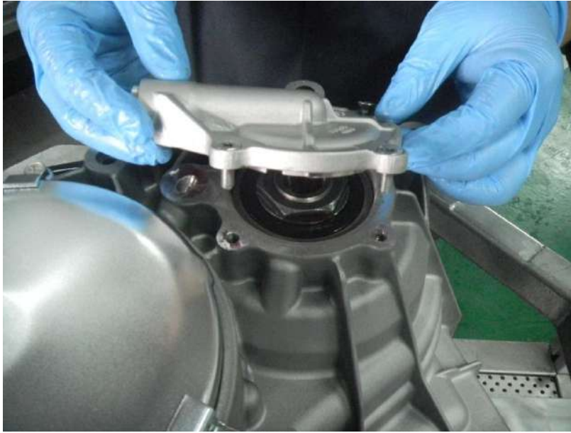
Fig.2 : remove secondary cover
