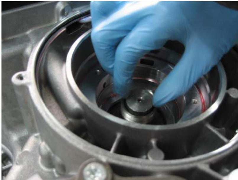
Fig. 7-3: Put special tool on shaft (primary plug 480139)
