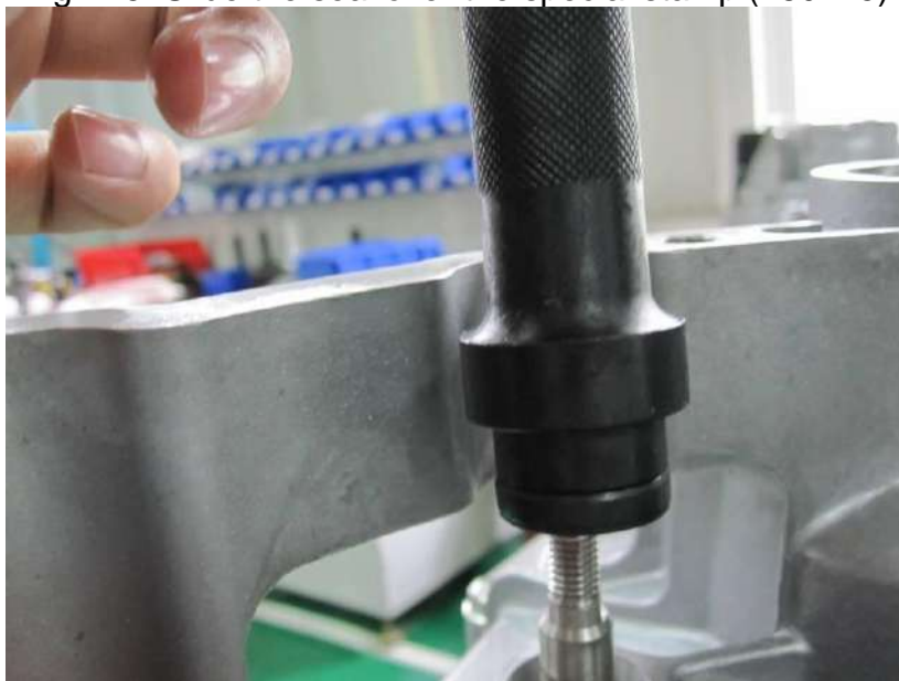
Fig. 4-6: Place special stamp (480125) with seal over the selector shaft
