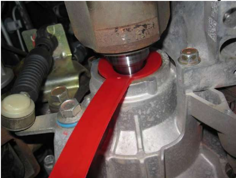
Fig. 1-4: 2 cm distance between drive shaft and tool 480145
