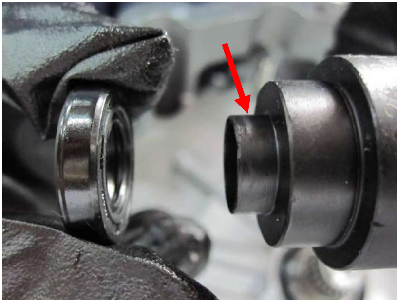
Fig. 4-5: Slide the seal over the special stamp (480125)
