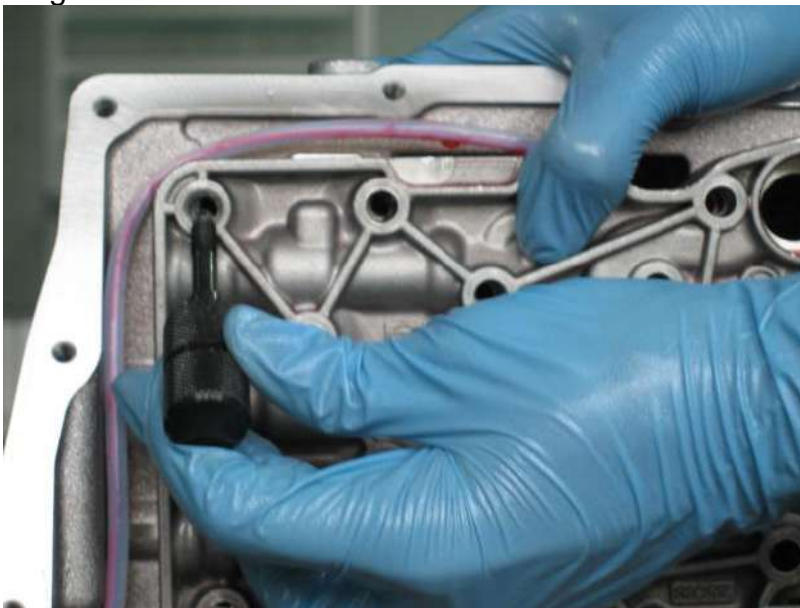
Fig. 12-6: Special alignment (480142) tool for hydr. unit
