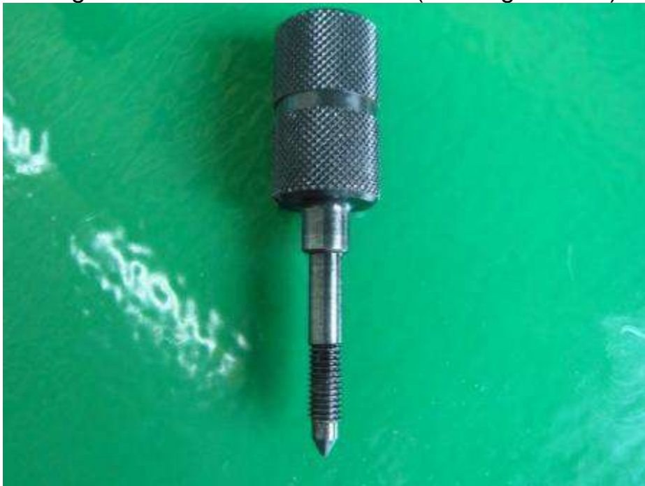
Centering pin – hydraulic unit (drawing 480142)
