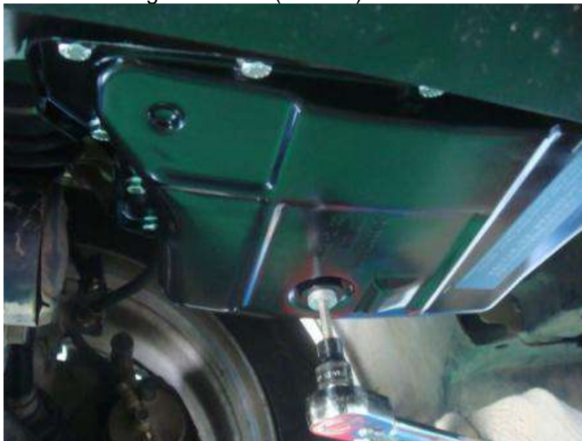
Fig. 9-1 Remove oil drain plug
