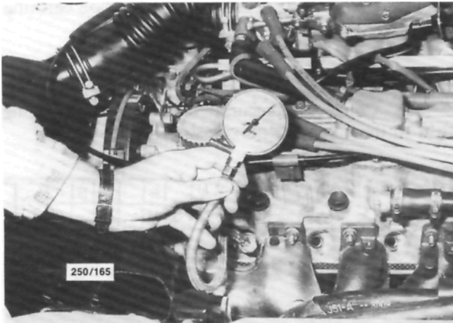
Check the cylinder compressions using a compression gauge.
