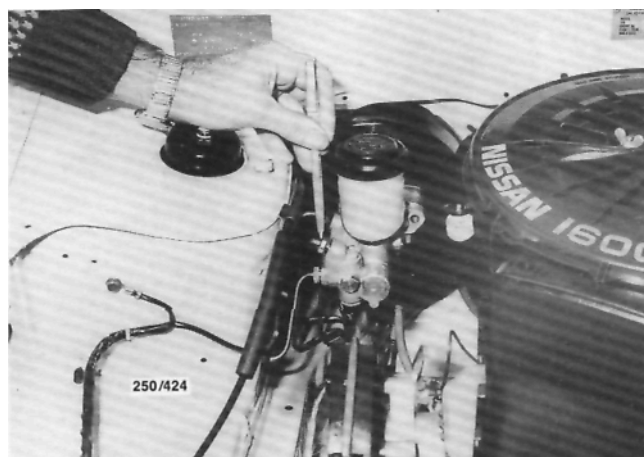
Check the brake pipe unions for leaks.
