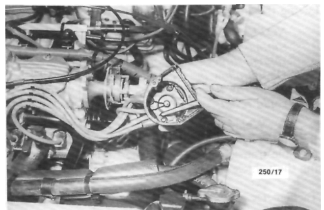
Check the distributor cap for cracks or tracking between the terminals.
