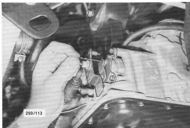
Using a 2.5 mm drill bit to adjust the neutral safety switch.
