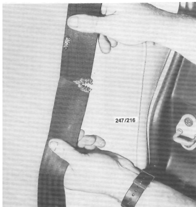
Check the seat belt webbing for fraying, cuts, burns or other damage.
