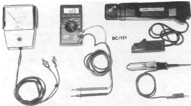
Assorted test equipment — dwell tachometer, digital multimeter, timing light and test lamp.
