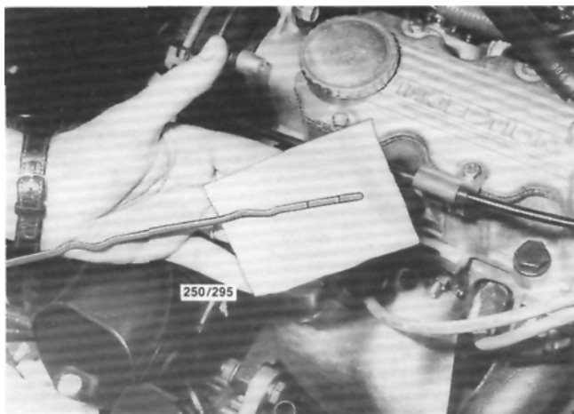
Check the engine oil for level and dilution on the dipstick.
