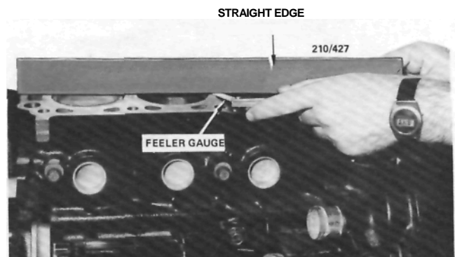
Checking the cylinder block face for distortion.
