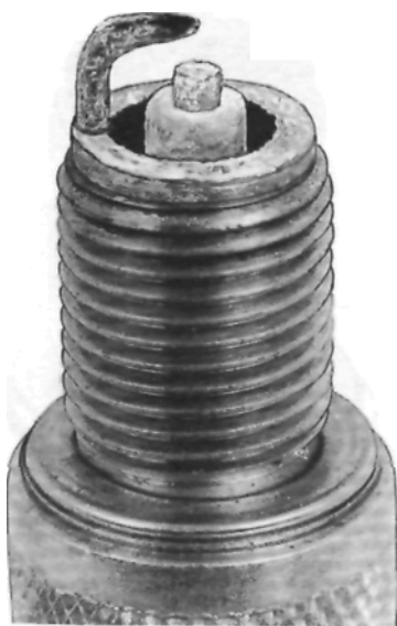
Spark plug with burnt electrodes and white blistered appearance, possibly due to incorrect plug type, loose plug or motor running too hot.
