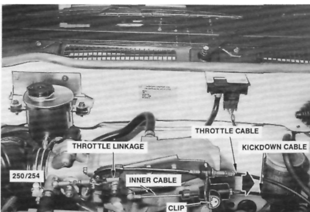
View of the kickdown cable adjustment point. The arrow indicates the direction in which the outer kickdown cable must be pulled to initiate the automatic adjustment. 1.8 liter engine.
