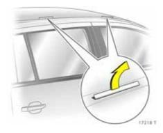
**Version without roof railing** Fold covers of installation openings up wards.
