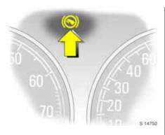
It is not necessary to select the neutral position before starting. If no gear is engaged, the transmission automatically shifts into neutral position (N) before starting the engine. This can lead to a slight delay when starting.
