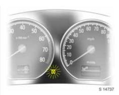
The self-cleaning function will automatically operate whilst driving after the engine has reached its normal operating temperature. The control indicator **W** will continue to flash until the self-cleaning operation is complete. This may take up to 20 minutes of driving. The time will be shorter at higher vehicle speeds. If the vehicle is not moving for more than a few minutes, then the selfcleaning function will not operate. Operation will continue when driving resumes.
