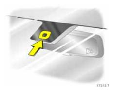
To ensure proper operation of the rain sensor \*, the sensor area must be free from dust, dirt and ice. The windscreen wash system must also be operated at regular intervals and the sensor area must be de-iced. Vehicles with rain sensor can be identified by the sensor area near the top of the windscreen. Service setting for front windscreen wiper (e.g. for changing or cleaning the front wiper blades).
