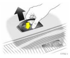
To open the loading floor, fold out release lever by pushing at the marked point and raise up the loading floor all the way.
