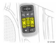
Vehicles with rear electric windows **\*** have a slide switch between the buttons in the driver's door
