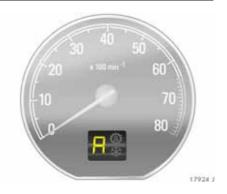
**Transmission display** Shows the mode or current gear.
