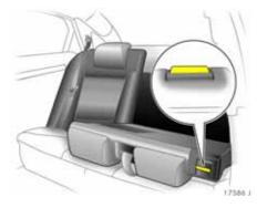
**Restoring backrest to an upright position** Audibly engage the rear seat backrests. There is a locking indicator on the release lever. If the rear seat backrests have been correctly locked the red indicator on the release levers must not be visible.
