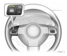
Selection using left-hand adjuster wheel on steering wheel:
