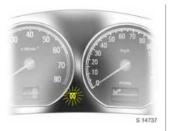
If the filter needs cleaning and recent driving situations did not allow the function to automatically operate, then control indicator **100** will flash. If this occurs, then you may continue to drive the vehicle normally. The vehicle will not be damaged and does not require service.
