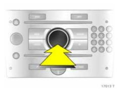
Selection using multi-function knob: Rotate and press multi-function knob.
