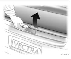
To unlock and open the luggage compartment: Press button ≥ on remote control, press button on boot lid/tailgate and for Estate, pull catch under handle
