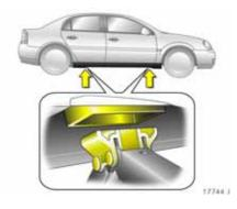
There are plastic retainers at the front and rear of the vehicle underbody for positioning the jack. The location of each retainer is indicated by a mark on the bottom edge of the vehicle.
