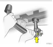
Inserting the coupling ball bar Insert the tensioned coupling ball bar in the coupling housing and push firmly upwards until you hear the coupling ball bar engaging.
