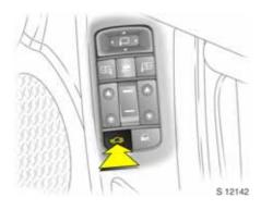
With the key in the starter switch and the handbrake applied, hold button 🖨 in the driver's door depressed for approx. 1 second; the tailgate opens electrically.
