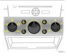
Vehicles without a n air conditioning system do not have buttons for cooling 森, air recirculation ☞ or demisting and defrosting ም.
