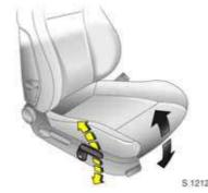
To adjust seat incline 🛠 Pump action of lever Upwards: Seat steeper Dow nwa rd s: Seat flatter
