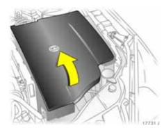
**Fusebox in engine compartment** The fusebox is in the box at the front of the engine compartment.
