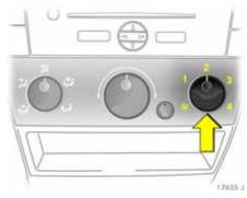
**Airflow** Setting with the right rotary knob.
