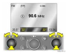
Common temperature setting Press the knob for the driver's side. The temperature for both the driver's and front passenger's side can be set together using the knob on the driver's side.
