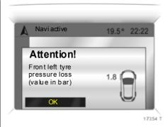
A diagram **\*** appears at the same time, marking the front left tyre and showing the current tyre pressure: Considerable pressure difference or direct loss of pressure. Exit flow of traffic as soon as possible without obstructing other vehicles, stop and check tyre and tyre pressure. Fit spare wheel if necessary see pages 236, 238.
