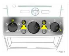
To demist or defrost windows: Set air distribution to **#i**, tum rotary knob for temperature and airflow clockwise;
