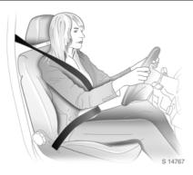
Adjust height such that the seat belt passes over the wearer's shoulder and rests against the shoulder. It must not pass over the neck or upper arm.
