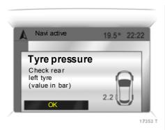
A graphic \* indicating the left rear tyre is shown together with the current tyre pressure: Slight pressure deviation. Reduce speed. Check pressure at next op portunity with appropriate gauge and correct if necessary.
