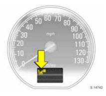
If control indicator ⊌<sup>\*</sup> does not illuminate whilst driving, the front and side airbags for the front passenger's seat are not deactivated and there is a risk of fatal injury to the child. Fit the child restraint systems on the rear seat. Have the cause of the fault eliminated by a workshop.
