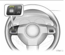
To select using the left adjuster wheel **\*** on the steering wheel Scroll upwards Previous menu item.
