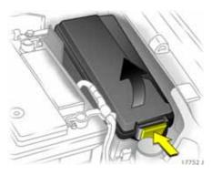
Disengage the bar at the front of the cover of fusebox and swing it upwards.
