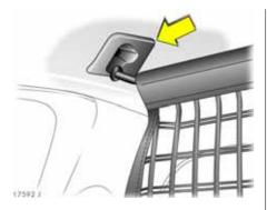
Extend the net from the cassette. The roof frame houses two installation openings. Fit the net rod in the installation opening on one side and then the other and engage by pushing forwards.
