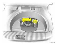
The tyre repair kit is in a compartment in the spare wheel well of the luggage compartment.
