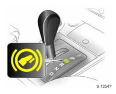
The engine can only be started with lever in position **P** or **N**. When position **N** is selected, depress footbrake or apply handbrake before starting.
