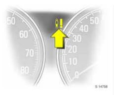
Control indicator I for Continuous Damping Control or SPORT mode fault Illuminates for a few seconds after the ignition is switched on. If the control indicator does not go out, or if it illuminates whilst driving, there is a fault in the Continuous Damping Control system or SPORT mode. The system is not ready for operation. Have the cause of the fault rectified by a workshop. The system's integrated self-diagnostics allows faults to be quickly remedied.
