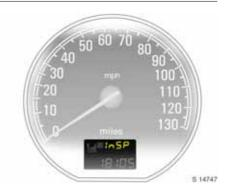
InSP Service interval display \* When InSP appears on the odometer display, make an appointment with a workshop for servicing as soon as possible. We recommend your Vauxhall Authorised Repairer.
