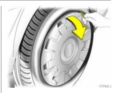
Prise off the wheel trim using the hook included with the vehicle tools \*. For vehicle tools - see page 238.
