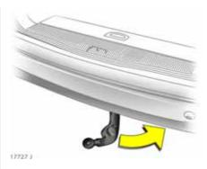
**Stowing the coupling ball bar** Open the stowage compartment – see page 222.
