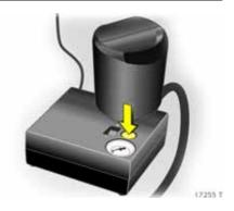
If the specified tyre pressure is not reached within 10 minutes, remove the tyre repairkit. Move the vehicle through one tyre rotation, approx. 2 metres, in either direction. Reconnect the tyre repair kit and continue the filling process for 10 minutes. If the specified tyre pressure is still not reached, the tyre is too badly damaged. Park the vehicle and contact a workshop. Drain excess tyre pressure with the button over the pressure indicator.
