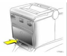
If it is correctly locked, the red mark must no longer be visible in the window, otherwise the procedure must be repeated.
