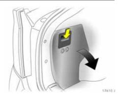
Tail lights Saloon / Hatch 1. To open the stowage compartment, press down bar and open the cover.
