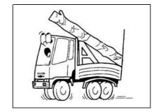
When long cargos are to be loaded, use rigid frames to minimize their protrusion from the rear end of the body.
