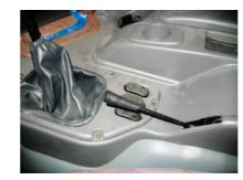
Loosen trailer brake hand brake valve handle to make handle return automatically.
