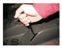
Tractor adopts separate trailer brake hand brake valve, its function is: auxiliary brake the trailer by controlling separately, especially for complete train running on ramp to lighten impulsion from trailer and make train decelerate calmly as well as increasing stabilization when braking.
