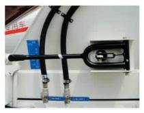
d. The stop of the agitating tank: pull the operation handle to "stop".
