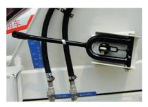
c. Stuff output of pre-agitating concrete: pull the operation handle to "low speed" or "high speed" position, meanwhile lock the stuff collecting trough in a specific position.
