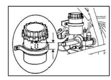
To Check the Fluid Level (If installed)
