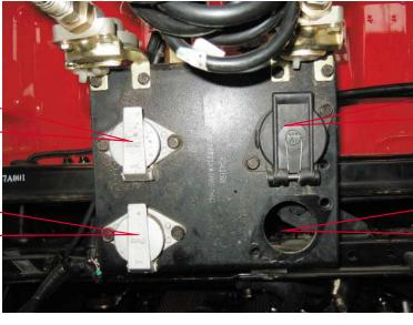
Interface for ABS cable on trailer
