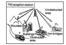
FM broadcasts are transmitted at high frequency and do not bend to follow the earth's surface. Because of this, FM broadcasts generally begin to fade at short distances from the station. Also, FM signals are easily affected by buildings, mountains, or other obstructions. These can result in certain listening conditions which might lead you to believe a problem exists with your radio. The following conditions are normal and do not indicate radio trouble:
