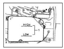
Check reservoir tank for the coolant level. The coolant level should be with in the range 1 shown in the illustration. If the level is low, add coolant by reference to "Replacement of coolant".
