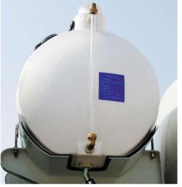
Water pump supply water tank
