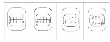
Your Manual Transmission vehicle has a fully synchro-meshed, 8-forward and 1-reverse or 5-forward and 1-reverse speed transmission controlled by a gear shift, lever located on the floor. This shift pattern is shown on the knob.
