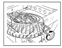
2. To install a tire, face the convex side of wheel upward, put the hanging plate in the disc wheel, and rotate the spare tire carrier handle clockwise to lift the tire.
