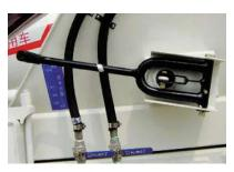
c. Stuff output of pre-agitating concrete: pull the operation handle to "low speed" or "high speed" position, meanwhile lock the stuff collecting trough in a specific position.
