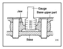
How to adjust inside diameter of jaw
