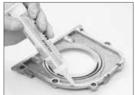
15.5 Apply RTV sealant to the sealing surface
