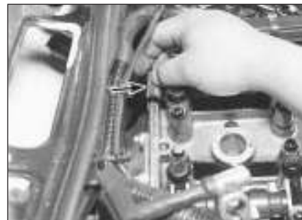
4.6 Apply RTV sealant to the half-circle rubber plugs and insert them into the cylinder head before refitting the valve cover
