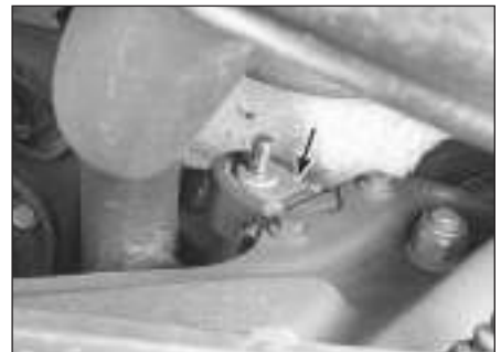
10.2 Check the exhaust system hangers (arrowed) for damage and cracks
