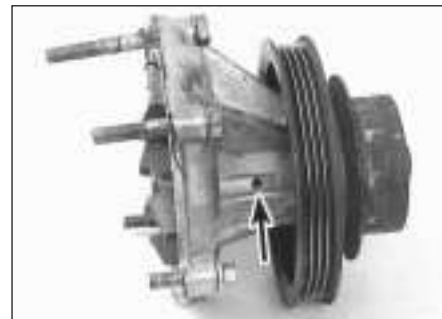
7.3 Check the weep hole (arrowed) for signs of leakage (pump removed for clarity) - grey discolouration is normal, large brown stains indicates seal failure
