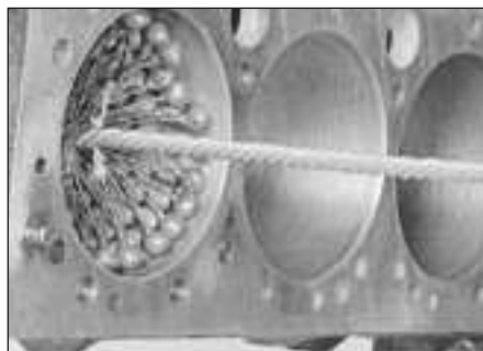
17.3a A "bottle brush" hone will produce better results if you have never done cylinder honing before
