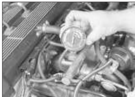
3.14 Connect a vacuum gauge to the vacuum line leading to the fuel pressure regulator and check the vacuum source
