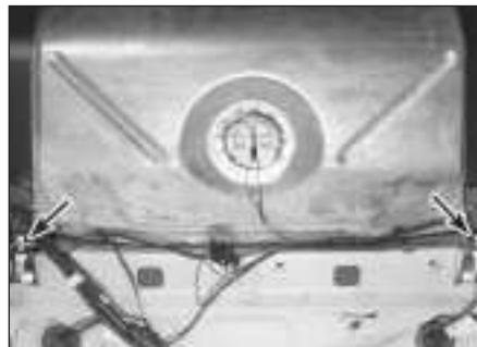
7.10 Remove the tank strap bolts (arrowed) from the body
