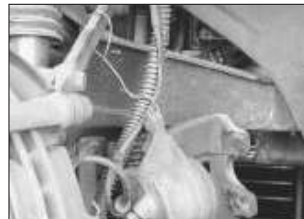
3.5e . . . and suspend it out of the way with a piece of wire
