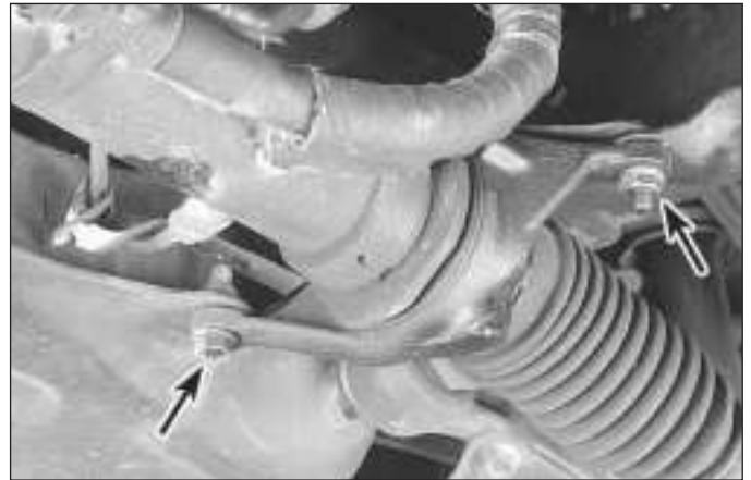
17.6 To detach the steering gear from the vehicle, remove these nuts and bolts (arrowed) from the mounting brackets (right bracket shown, left bracket similar)
