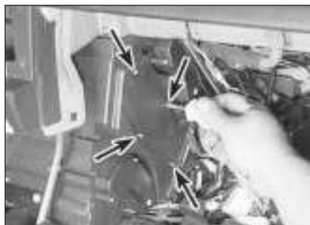
11.7 Remove the four screws (arrowed) and the heater core cover plate
