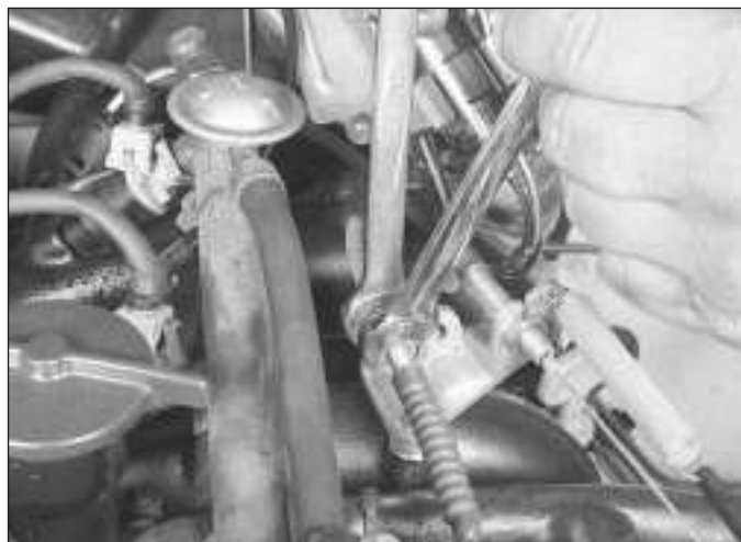
10.2 Loosen the locknuts on the accelerator cable
