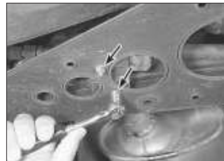
4.6 Remove the fuel pump mounting nuts (arrowed) and slide the fuel pump out of the rubber casing (1989 model shown)
