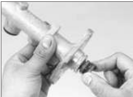
6.7g Remove the primary piston
