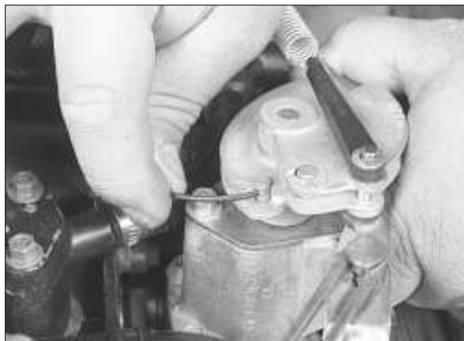
10.3 Rotate the bellcrank and remove the cable end from the slot
