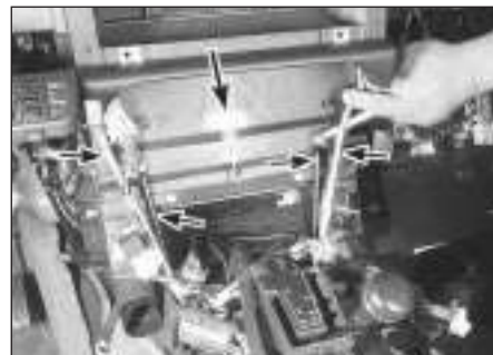
17.9a Unbolt the four support braces (small arrows) from the case (large arrow) and floor
