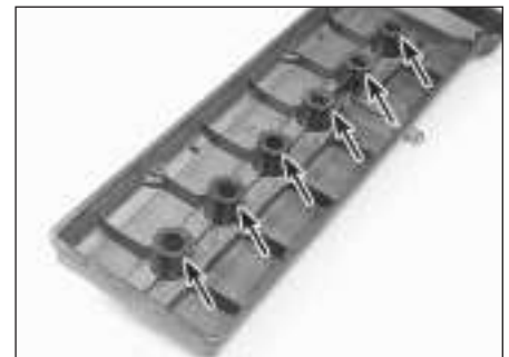
4.7 Press the valve cover gasket into the groove around the valve cover and fit a new set of spark plug tube seals (arrowed)
