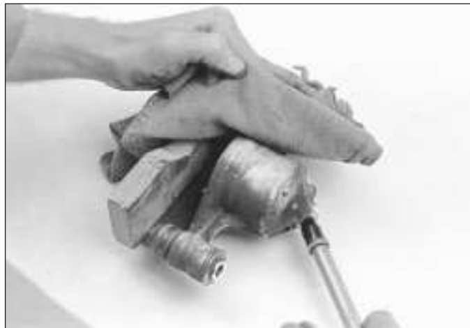
4.5 With the caliper padded to catch the piston, use compressed air to force the piston out of its bore - make sure your fingers are not between the piston and the caliper
