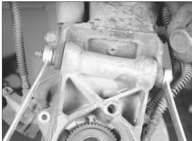
11.5 To detach the hub carrier from the rear control arm, remove the carrier-to-control arm nut and bolt
