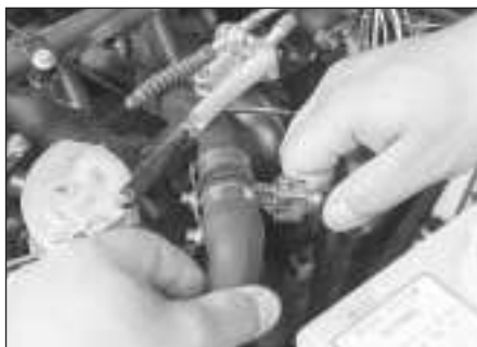
8.7 Disconnect the electrical connector from the electronic heating element
