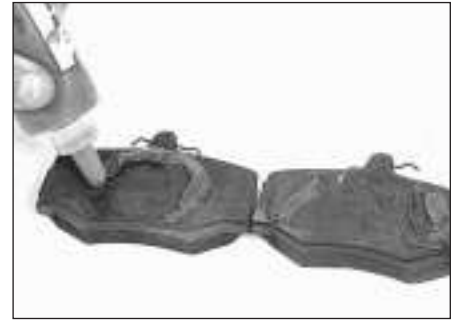
3.5k Apply anti-squeal compound to the new brake pads
