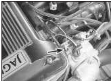
9.3 The coolant temperature sender unit (arrowed) is located in the top of the thermostat housing - it is the sender unit with the single wire
