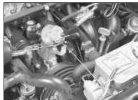
10.10 Attach a strong wire (coat hanger) to the master cylinder using a clamp and align it with the notch on the bellcrank
