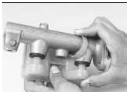
6.7s Align the reservoir pipes with the grommets as shown . . .
