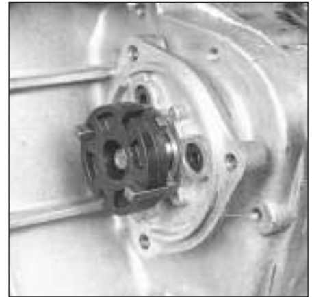
18.6c . . . and on the drive coupling on the auxiliary shaft side; note that the two lugs on each drive coupling fit into their corresponding slots in the coupling disc, 180° apart - all four lugs must be properly engaged or you won't be able to bolt the adapter to the auxiliary shaft housing
