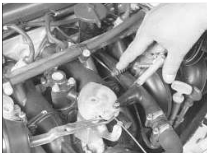
10.9 Make sure the throttle closes completely and there is a slight amount of flex in the cable
