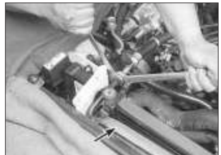
16.3 Disconnect the two lines, then pull up on the condenser (arrowed)
