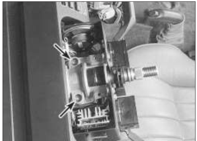
9.5 To remove the ignition switch/lock cylinder assembly, drill out the centre of the two retaining bolts (arrowed) and remove them with a screw extractor
