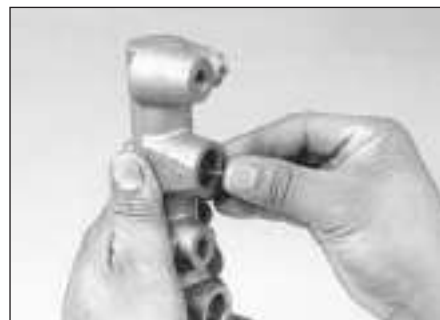
6.7o Using the same technique as in illustration 6.7f, depress the pistons and refit the stopper pin
