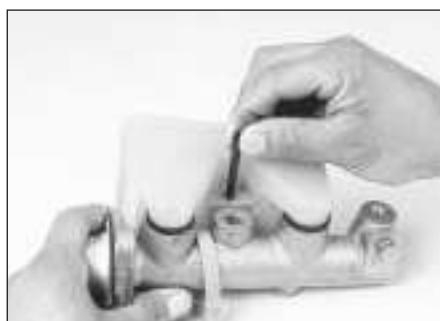
6.7u Refit the reservoir roll pin . . .
