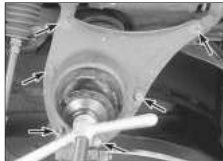
8.3 To detach the coil spring pan from the lower control arm, compress the spring and remove these six bolts (arrowed)
