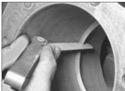
22.4 With the ring square in the cylinder, measure the end gap with a feeler gauge
