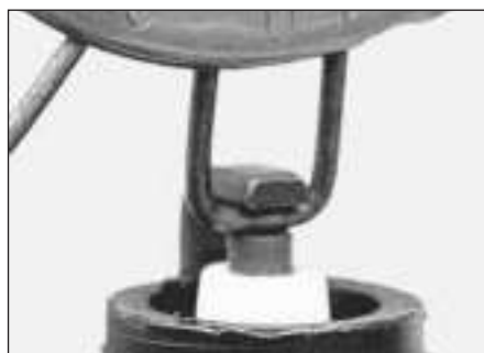
4.4a Spark plug manufacturers recommend using a wire-type gauge when checking the gap - if the wire does not slide between the electrodes with a slight drag, adjustment is required
