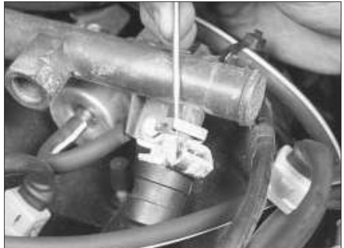
13.37 Remove the fuel injector retaining clips from the fuel rail using a small screwdriver
