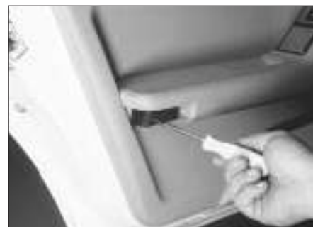
18.7b Remove the retaining screw from inside the lamp housing
