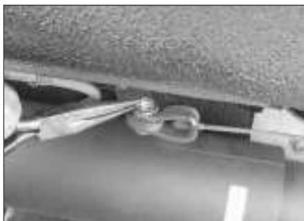
11.2 To disconnect the forward end of the front cable from the handbrake lever, remove this cotter pin, washer and clevis pin
