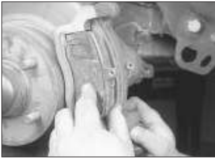
3.5f Remove the outer brake pad
