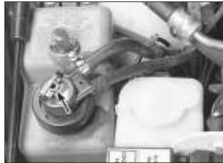
5.3 To add fluid, remove the filler hole dust cap (arrowed)
