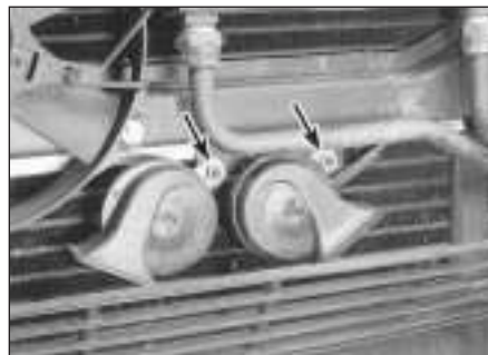
20.9 Disconnect the electrical connector, remove the retaining nuts (arrowed) - then detach the horn(s)
