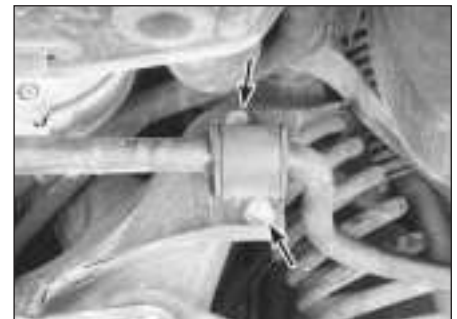
3.2 To detach the anti-roll bar from the suspension crossmember, remove these two bolts (arrowed) from each bushing bracket
