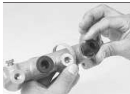
6.7r Refit the grommets
