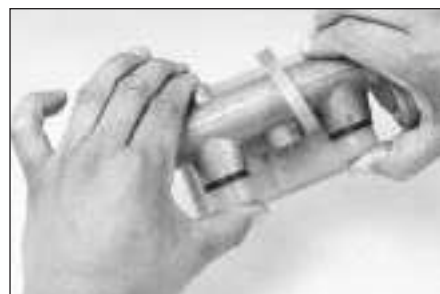
6.7t . . . and squeeze the reservoir and master cylinder together; make sure the reservoir is fully seated
