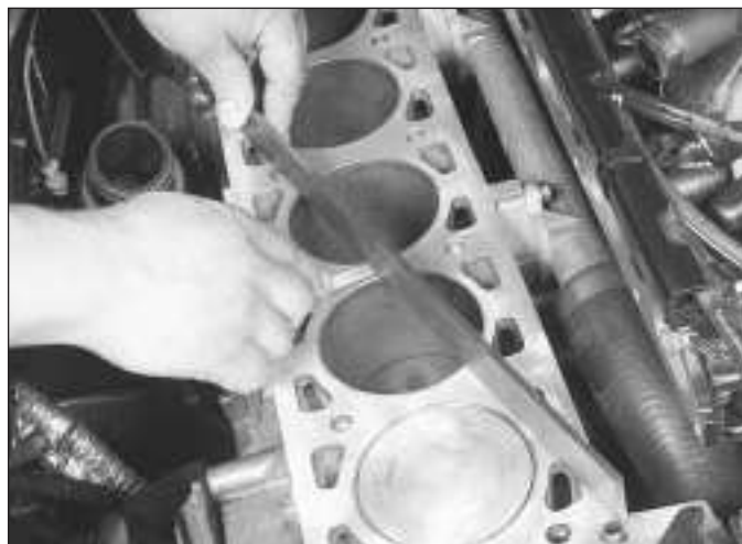
10.13 Check the cylinder head and engine block gasket surfaces for warpage by trying to slip a feeler gauge under a precision straightedge (see the Specifications for the maximum warpage allowed and use a feeler gauge of that thickness) - check both the cylinder head and engine block (shown)
