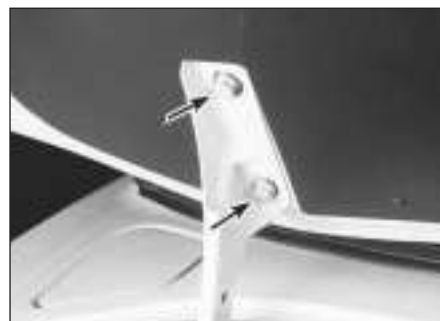
16.4 With the help of an assistant to hold the boot lid, remove the retaining bolts and lift off the boot lid
