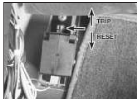
22.2 The inertia switch is located behind the passengers side kick panel - pull upward on the button to trip the switch - push downward on the button to reset the switch
