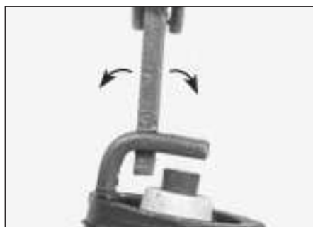
4.4b To change the gap, bend the side electrode only, as indicated by the arrows, and be very careful not to crack or chip the porcelain insulator surrounding the centre electrode
