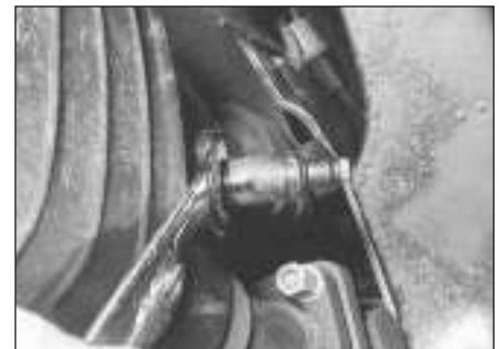
4.21 Unscrew the oxygen sensor from the exhaust system
