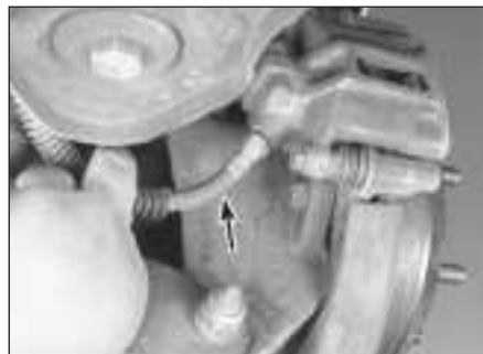
11.11 Check along the brake hoses and at each fitting (arrowed) for deterioration and cracks
