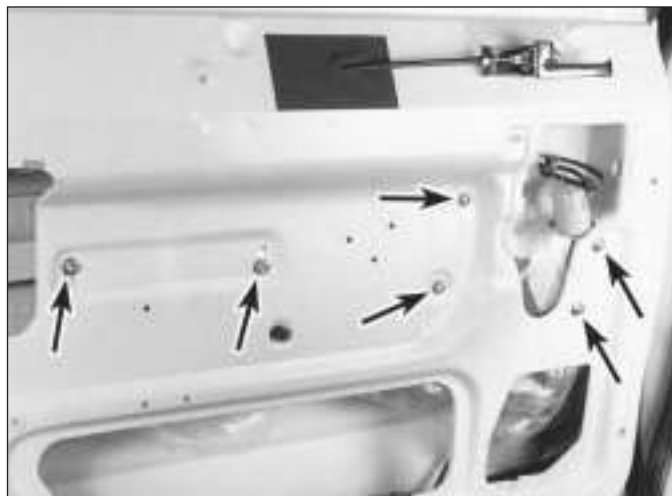
21.3 Detach the window regulator bolts (arrowed)
