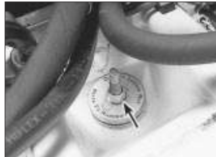
4.4 To disconnect the upper end of the shock absorber from the body, remove this nut (arrowed)
