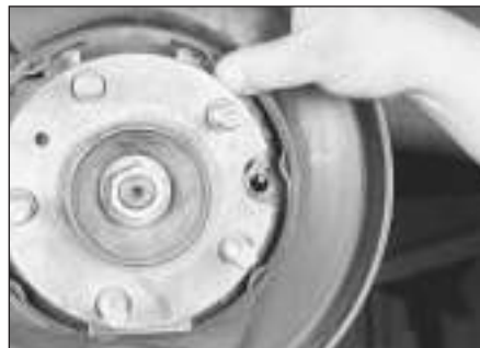
12.5o . . . place the rear shoe in position, insert the pin through the backing plate and the shoe and refit the rear washers and hold-down spring
