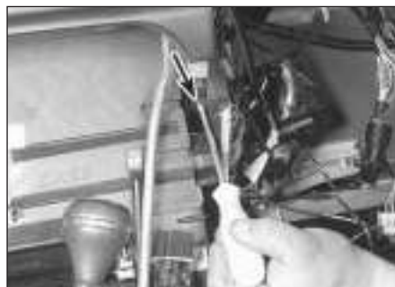
11.6a Remove three screws (one arrowed; one at the top-back and one below) to take out the climate-control computer on right side of heater/air conditioning assembly
