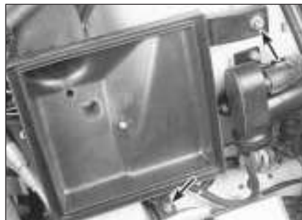
9.2a Remove the bolts (arrowed) from the air cleaner assembly
