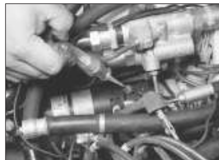
6.11 Refit the LED test light to the coil negative (-) terminal, crank the engine over and observe the light flash in response to the trigger signal from the computer
