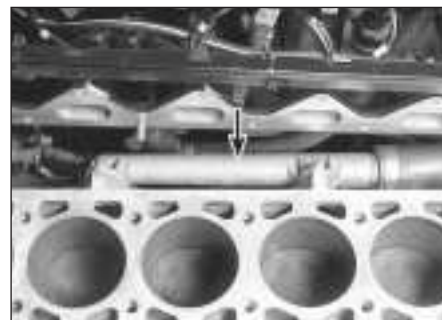
8.8b The water pipe (arrowed) may need new gaskets where it meets the block - the pipe is best accessed from below or with the intake manifold unbolted
