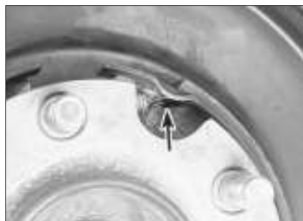
12.5q . . . and into the rear shoe
