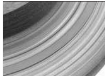
5.3 The brake pads on this vehicle were obviously neglected, as they wore down to the rivets and cut deep grooves into the disc - this disc must be replaced
