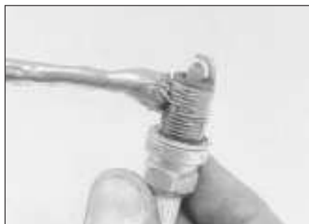
4.10 Apply a coat of anti-seize compound to the spark plug threads
