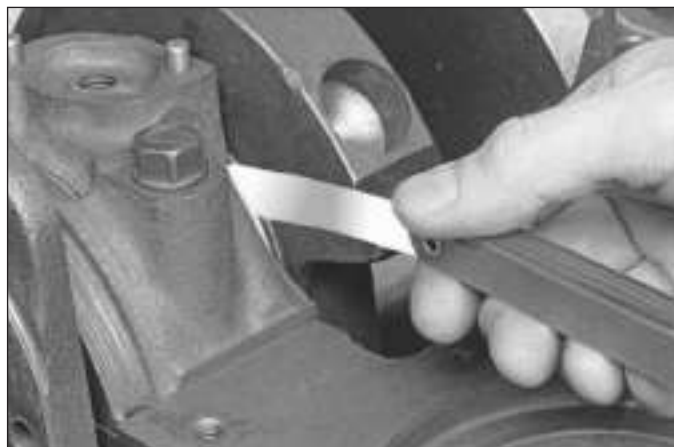
14.3 Checking crankshaft endplay with a feeler gauge
