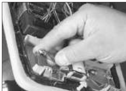
21.9 The interior light bulbs can be accessed after lowering the overhead console
