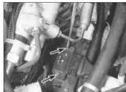
7.5 Remove the amplifier mountings screws (arrowed) and lift the unit from the engine compartment
