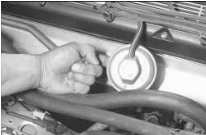
6.5 Use a fingertip to move the diaphragm inside the EGR valve
