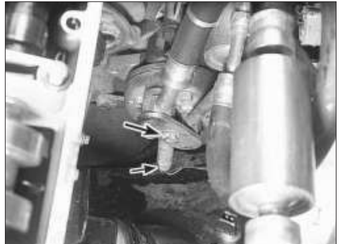
15.4 Disconnect the electrical connector (small arrow) at the compressor, then disconnect the bolt (large arrow) at the retaining plate that holds the two hoses in place
