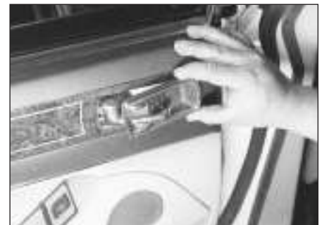
18.3b . . . then detach the inside handle retaining screw and bezel
