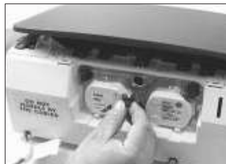
21.10 To remove an instrument cluster bulb, depress the bulbholder and rotate it anti-clockwise
