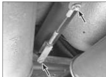
11.5 To disconnect the intermediate cable, remove the cotter pins, washers and clevis pins (arrowed) from the adjuster lever and the yoke
