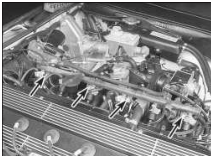
13.35 Remove the fuel rail mounting bolts (arrowed) . . .
