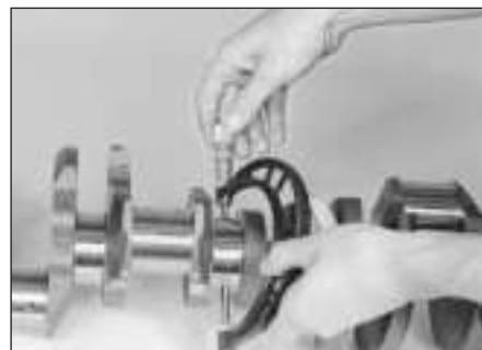
19.5 Measure the diameter of each crankshaft journal at several points to detect taper and out-of-round conditions
