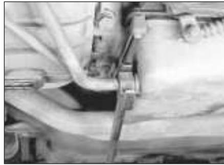
26.6a Unscrew the dipstick tube collar
