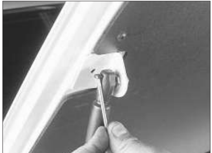
9.2b The boot lid support strut requires prising out a locking pin to detach it from the locating stud
