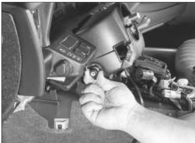
27.2 Pull off the knob from the instrument panel light rheostat
