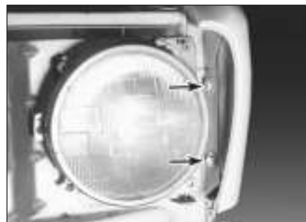
15.7a Detach the wing retaining bolts (arrowed) at the front of the wing
