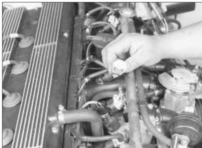
12.8 Refit the "noid" light into the fuel injector electrical connector and check to see that it blinks with the engine running
