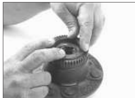
22.19 After refitting the inner wheel bearing into the hub - press the grease seal into place
