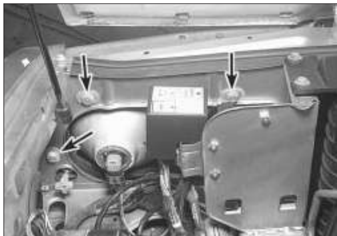
19.2 Remove the headlight housing retaining nuts (arrowed) from the backside of the radiator support
