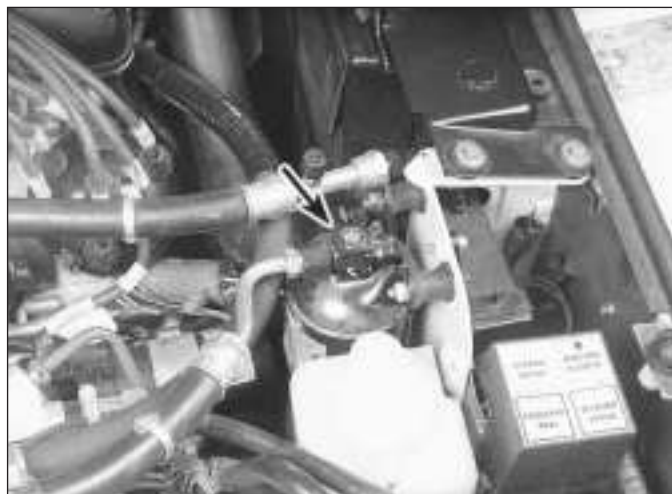
13.11 The sight glass (arrowed) is located on the top of the receiver/drier, to the right of the radiator
