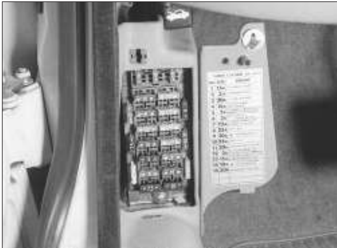
3.1a The left side fusebox is located in the passenger's side kick panel, behind the fuse panel cover
