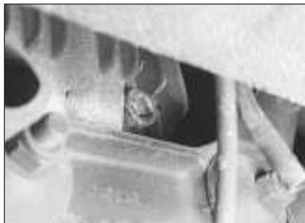
9.2 The differential check/fill plug is located on the rear of the differential housing - place your finger in the filler plug hole to make sure the lubricant level is even with the bottom of the hole
