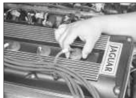
4.6 When removing the spark plug leads, grasp only the boot and use a twisting/pulling motion
