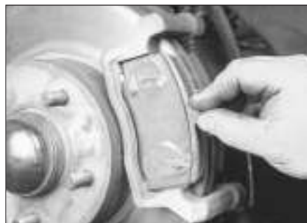
3.5n Refit the outer pad
