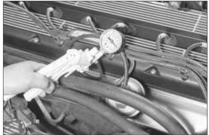
6.4 Apply vacuum to the EGR valve and confirm that the valve opens and allows exhaust gases to circulate. Once it is activated, the EGR valve should hold steady (no loss in vacuum)
