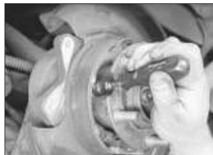
12.5c Remove the front hold-down spring, washers and pin; note that one washer goes below the spring and one above it
