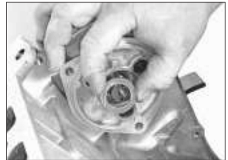
9.10 Refit the washer before replacing the snap-ring
