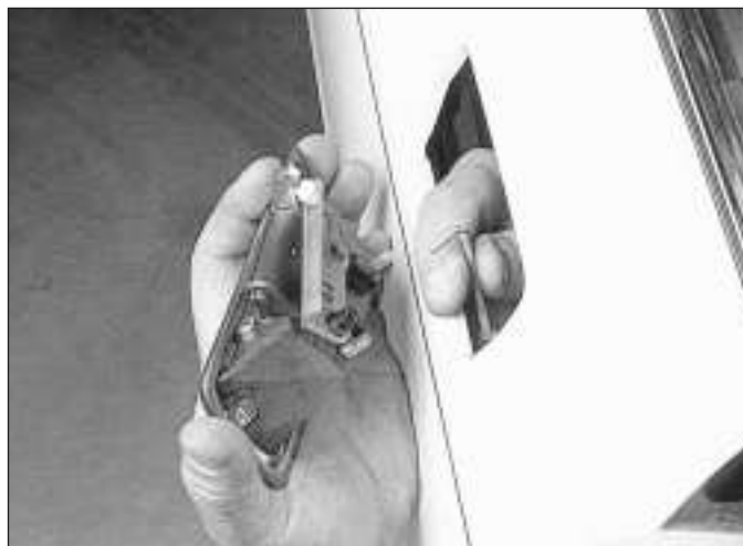
20.8 Detach the plastic clip securing the lock rod
