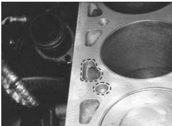
10.12 Place the new head gasket on the engine block, and trace around the water passages and bolt holes - make sure there is no erosion of the aluminium beyond these lines
