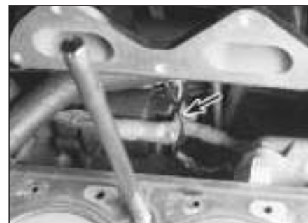
15.4b From underneath the vehicle, remove the battery terminal from the solenoid (cylinder head removed for clarity)
