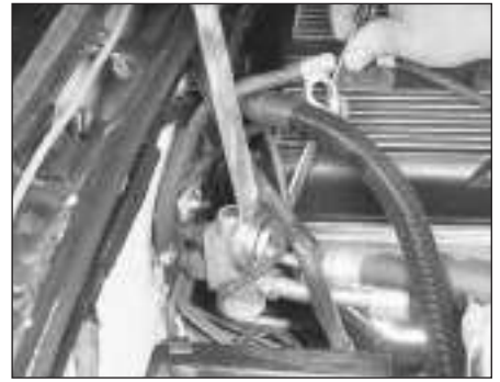
17.13 Disconnect the lines at the front of the expansion valve - always use two spanners to avoid twisting a line - one spanner holds the body of the valve
