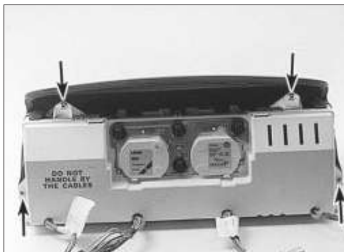
12.3 Remove the instrument cluster retaining screws (arrowed) then separate the instrument cluster from the cluster housing
