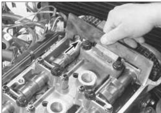
10.5 Position the camshaft alignment tool over each camshaft - the projection on the tool only fits into the slot on the camshafts when they are at TDC - flip the tool over to check the other camshaft
