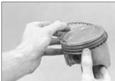
22.9a Refit the spacer/expander in the oil control ring groove
