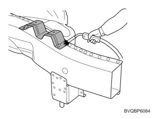
10. Apply the two-part epoxy primer to the interior of the front side member.
