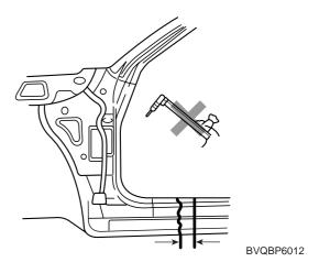
Removing paint from an area to be spot welded Using a torch and wire brush, remove paint completely before beginning welding.
