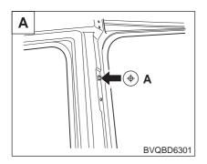
Rear door stopper mounting hole (ø10)
