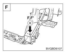
Front bumper bracket mounting hole (ø9)
