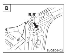
Curtain airbag mounting hole (ø6.6)
