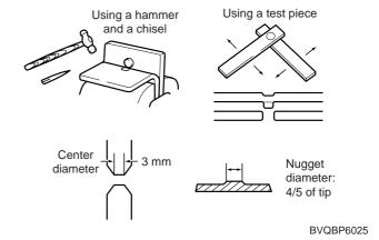
c) The tip of the spot welding machine should be maintained to a minimum tolerance of 3 mm. Also let area cool after 5 or 6 welds to minimize problems caused by excessive heat.
