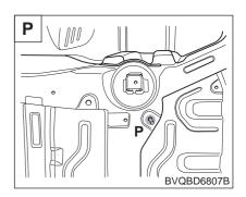
Brake pipe bolt mounting hole (Ø16)
