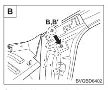
Curtain airbag mounting hole (ø6.6)
