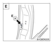
Front door switch mounting hole (R9.2X9.2)
