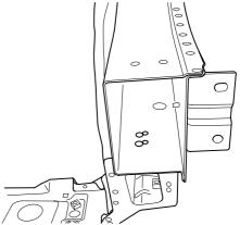
2. Drill out all the spotwelds to separate radiator support panel from front side member(7 points).
