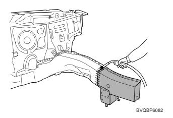
8. Clean MIG welds with a disc grinder.
