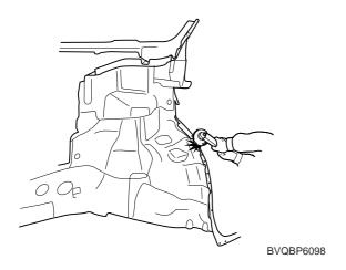
15. Apply the two-part epoxy primer to the interior of the front side member
