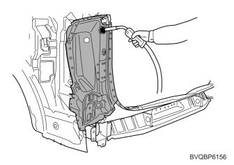
4. Clean and prepare all surfaces to be welded and remove all residue.
