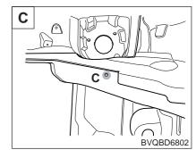
Brake pipe mounting hole (ø7)
