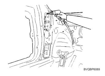
Before cutting front pillar, be sure to support roof panel.
