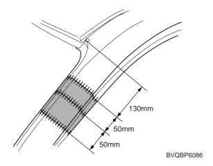
2. Measure and mark the cut line on front side sill outer panel as shown in the illustration.
