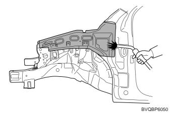
5. Clean MIG welds with a disc grinder.
