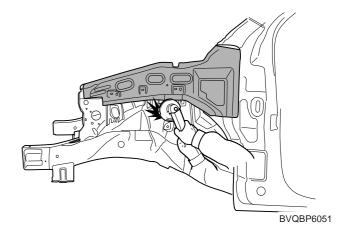
After welding the cowl side outer panel, apply the epoxy primer and anti corrosion to the cowl side outer panel.
