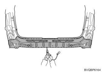
Clean and prepare all surfaces to be welded and remove all residue.
