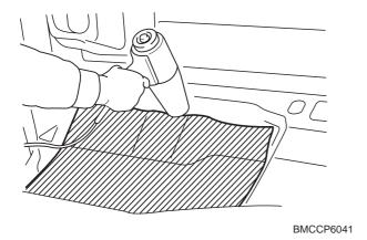
2. Align the antivibration pad layer in the position where it is to be installed, and then press it down with a roller or a block of wood so that it adheres well.
