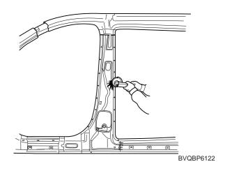
7. Apply the epoxy primer to the side inner reinforcement.
