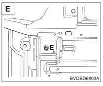
Sub frame rear mounting hole (Ø18)
