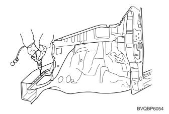
2. Clean MIG welds with a disc grinder.
