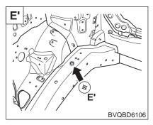
Engine bracket mounting hole (ø18)
