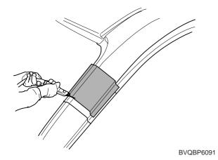
Cut the front pillar through each cut line, taking care not to damage the other panel as illustration.
