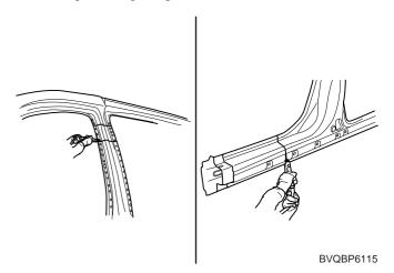
6. After cutting side outer panel (center pillar outer & side sill), cut the center pillar outer reinforcement and center pillar inner panel.
