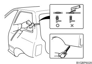
b) Finish areas that have been brazed by applying body filler then smooth the area with a flexible file and sander.
