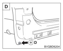
Front fender mounting hole (ø10)
