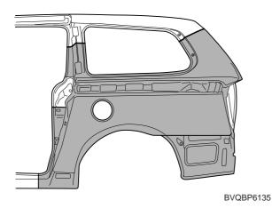
Apply body filler to the welded seam. Sand and finish.
