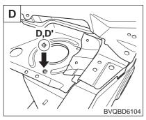
Front strut mounting hole (ø14)
