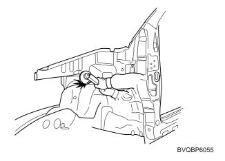
3. Before welding the fender apron inner lower panel, apply the epoxy primer to the interior of the fender apron inner lower panel.
