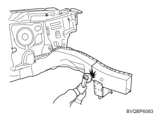
MIG plug weld engine mounting bracket from front side member.
