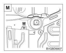
Sub frame mounting hole (Ø18)
