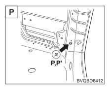
Wire harness earth mounting hole (ø9)
