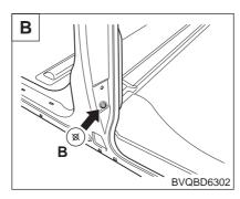
Rear door stopper mounting hole (ø10)
