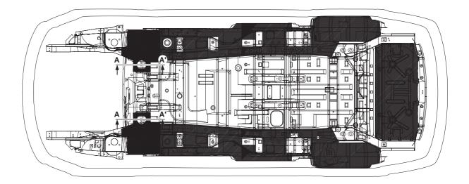
Under body coating (Thickness : 0.8 mm, :1.5 mm)
