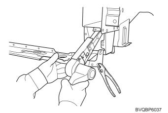
4. Clean MIG welds with a disc grinder.
