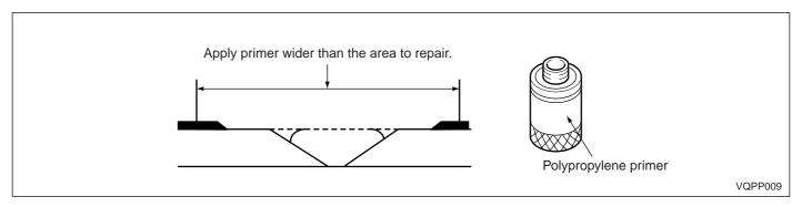
6. Mix main filler material and hardener at a ratio depending on paint specifications. Mix filler material and apply over the damaged area.
