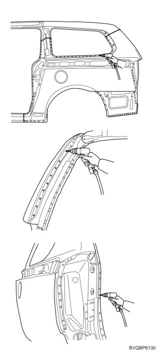
3. Cut the quarter outer panel at cutlines and remove the quarter outer panel as illustration.
