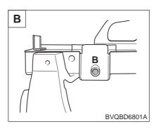
Sub frame front mounting hole (Ø16)
