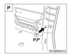
Wire harness earth mounting hole (Ø9)
