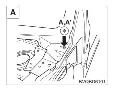
Hood hinge mounting hole (ø12)
