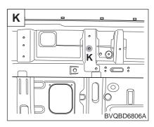
Traling arm mounting front hole (ø14
