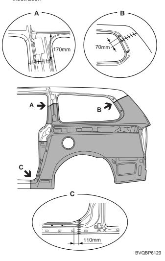
Drill out all attaching spdtwelds the quarter outer panel.
