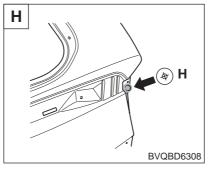
Center rail cover mounting hole (Ø10)
