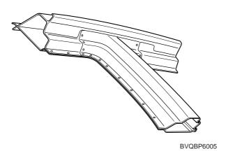
2. When spot welding, weld in the middle of the joint.
