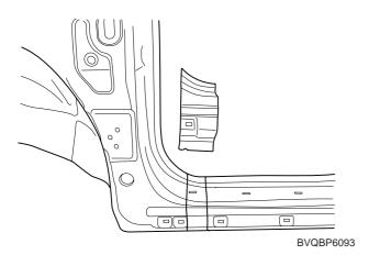
13. Straighten all flanges as necessary, prepare all surfaces to be welded.
