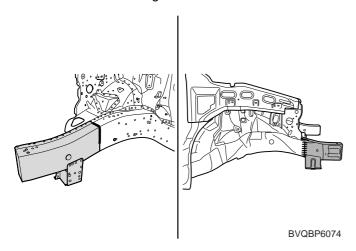
Drill out the spotwelds to separate front side member from engine mounting bracket.(6points)
