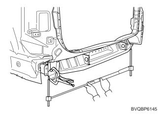
3. MIG plug weld at the holes and MIG butt weld the seam in the side member.
