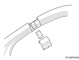
12. Cut the side sill inner panel vertical cutting line and remove the front pillar.
