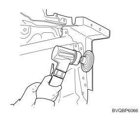
5. Apply the epoxy primer to interior of the fender aproninner upper panel.
