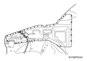
2. Using a disc grinder, remove the cowl side outer panel by drilling out the MIG lap welds.(5 points)
