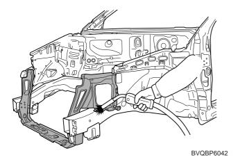
6. Clean MIG welds with a disc grinder.
