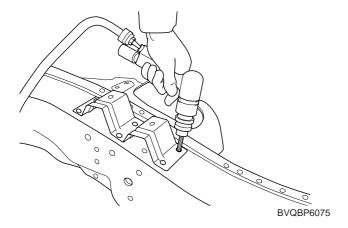
Drill out all the spotwelds to separate fender apron inner panel from front side member.
