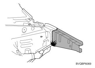
After welding the fender apron inner upper panel, measure each measurement point(refer to the BODY DIMENSIONS) and correct the installation position.
