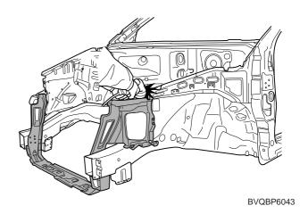
After welding the radiator support panel, apply the epoxy primer and anti-corrosion to the radiator support panel
