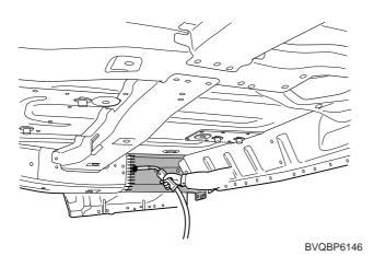
4. Clean and prepare all surfaces to be welded and remove all residue.
