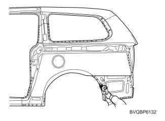
6. Apply the two-part epoxy primer to the quarter inner panel.
