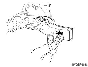
5. Before welding the radiator support panel, apply the epoxy primer to the interior of the radiator support panel
