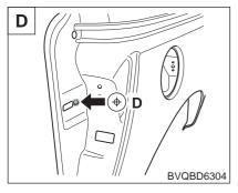
Rear door switch mounting hole (Ø8)
