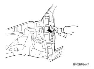
Before welding the cowl side outer panel, apply the epoxy primer to the interior of the cowl side outer panel.
