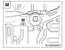
Sub frame mounting hole (ø18)
