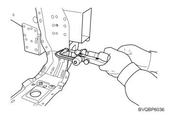
3. Using a belt sander, remove the front side member by drilling out the spotwelds(4points).
