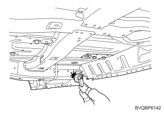
7. Apply the two-part epoxy primer to the rear floor side member.
