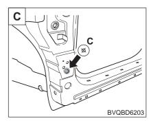
Front door hinge mounting hole (ø13)
