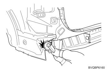
3. Apply the two-part epoxy primer to the interior of the rear floor side member.
