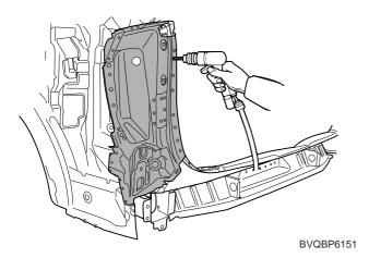
2. Clean MIG welds with s disc grinder.
