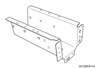
Fit and clamp the new rear floor side member in place for welding.
