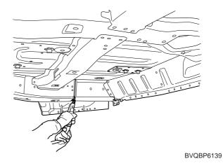
Remove the rear floor side member by drilling out all attaching spotwelds.
