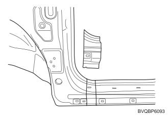
10. Drill out all the spotwelds to separate side outer panel from side inner panel (82points).
