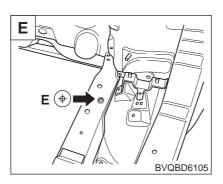
Transaxle bracket mounting hole (ø12)
