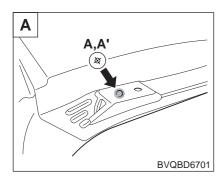
Tail gate hinge mounting hole (ø12)
