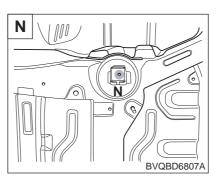
Rear bumper stopper mounting hole (Ø11)
