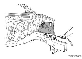
5. Clean MIG welds with a disc grinder.
