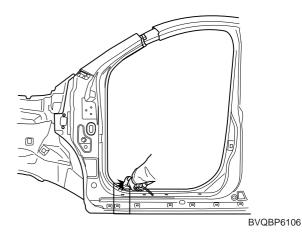
18. Before welding the cowl side upper outer panel, apply the two-part epoxy primer and anti-corrosion agent to the interior of the cowl side upper outer panel.
