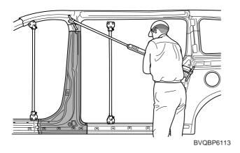
4. Drill out all spotwelds and cut all laser welds attaching the center outer pillar to the body to remove center outer pillar.
