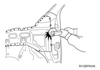
3. Clean MIG welds with a disc grinder.
