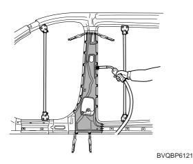
6. Clean MIG welds with a disc grinder.
