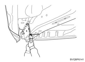
6. Clean MIG welds with a disc grinder.
