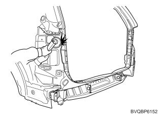
3. Apply the two-part epoxy primer to the interior of the rear floor side member.
