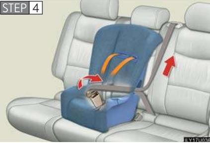
While pushing the child seat into the seat, allow the shoulder belt to retract until the child seat is securely in place.
