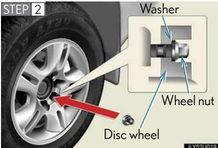
Install the spare tire and loosely tighten each nut by hand to approximately the same amount.
