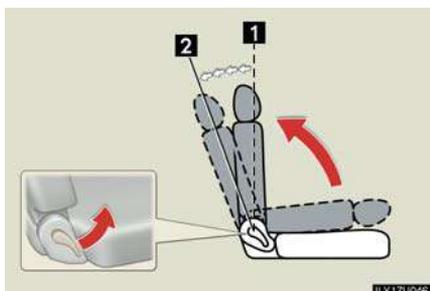
Fold the seatback forward and then back to the 1st lock position (most upright position) until it locks into place. Adjust the seatback to the 5th lock position.
