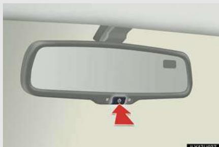
Press the button for longer than 3 seconds to turn auto mode on/off.
