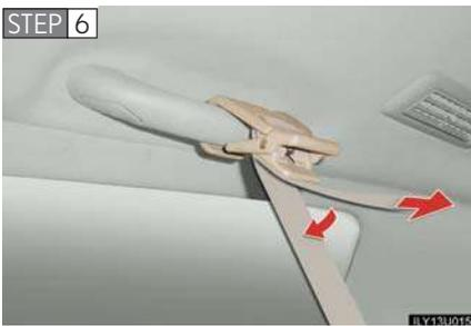
Pull the free end of the straps to the secure the seats.
