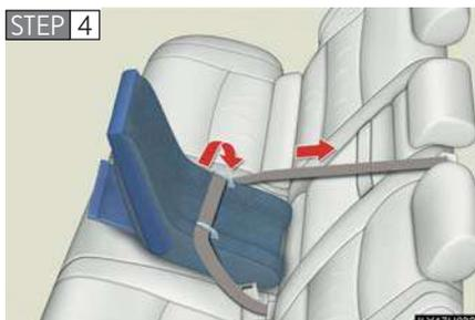
While pushing the child seat down into the seat, allow the shoulder belt to retract until the child seat is securely in place.
