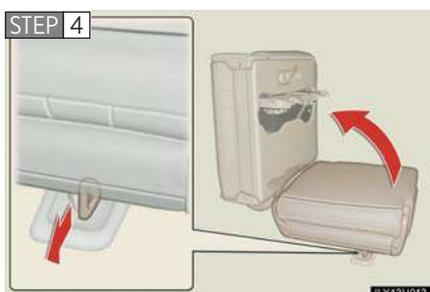
Unlock the seat legs by pulling the seat leg lock release handles, and lift the seats sideward.
