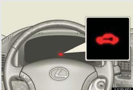
To arm the alarm, exit the vehicle, make sure that the doors and hood are closed, and lock all the doors.
