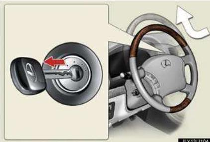
When the ignition key is removed, the steering wheel returns to its stowed position by moving up and away to enable easier driver entry and exit.
