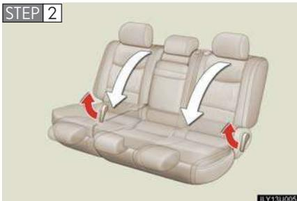
Fold down the seatbacks while pulling the lock release levers.
