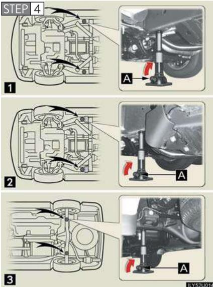
Turn the tire jack portion "A" by hand until the head of the jack is in contact with the appropriate jack point.
