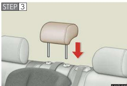
Reinstall the head restraint.
