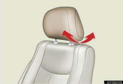
Grip the head restraint and twist to tilt forward or backward.
