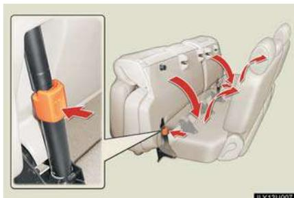
Push the red knobs and swing the seat down, then raise the seat-backs.
