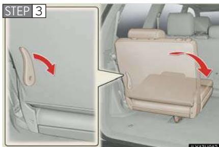
Unlock the seatbacks by pushing the lock release levers forward, and fold them down.
