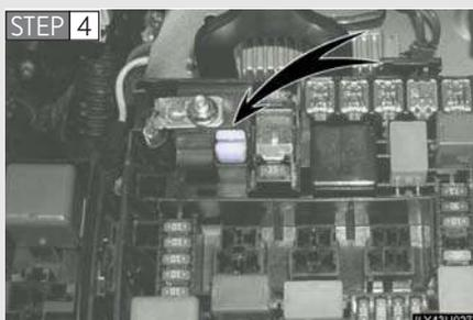
Remove the fuse with the pull-out tool.
