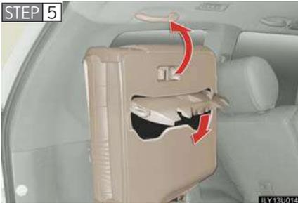
Retract the seat legs, then take the holding straps out and attach the straps to the assist grips.
