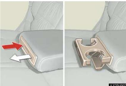
To open, press in and release the rear cup holder on the armrest.
