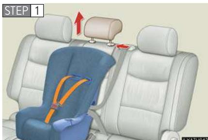
Secure the child restraint using a seat belt or lower anchors, and remove the head restraint.
