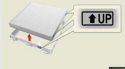
Remove the air conditioning filter from the filter case and replace it with a new one.
