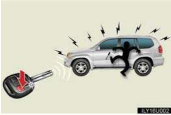
When the “PANIC” button is pushed for longer than about 1 second, the headlights/tail lights/emergency flashers will flash, the interior lights will come on, and an alarm will sound for about 60 seconds to deter any person from trying to break into or damage your vehicle.
