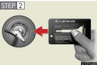
Bring the key case close to the engine switch within 10 seconds as indicated by an arrow.
