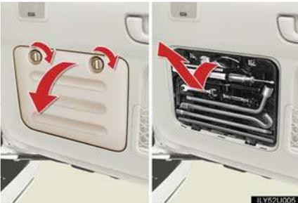
Remove the tool tray compartment cover and take out the tool tray.
