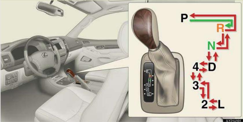
← While the engine switch is in the “ON” position, depress the brake pedal and move the shift lever.
