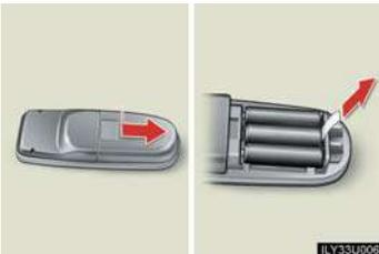
An insulating sheet is set to prevent the batteries from being discharged. Remove the insulating sheet before using the remote control.
