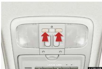
Press and hold down the 2 outside buttons for 20 seconds until the indicator light flashes.
