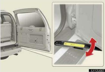
You can hold the back door in this position using the back door stopper.
