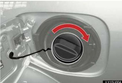
When installing the cap, turn it clockwise until one click is heard, in order to fully close it.
