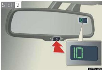
**STEP 2** Press the button until a number (1 to 15) appears on the compass display.
