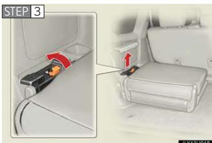
Remove the seat lock cover and push the red seat lock release knobs outward, then lift the seats free.
