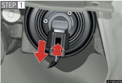
Unplug the connector while pushing the lock release.
