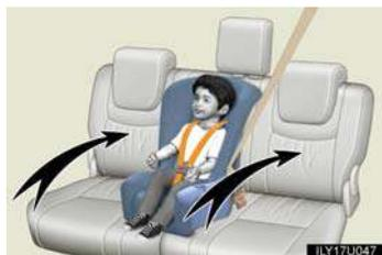
● When installing a child restraint system in the third center position, set the both seat-backs to the same angle. Otherwise, the child restraint system cannot be properly secured.
