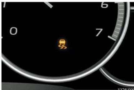
If the vehicle is in danger of slipping, rolling backwards when starting on an incline, or if the rear wheels spin, the slip indicator light flashes to indicate that the VSC/TRAC/hill-start assist control systems have been engaged.
