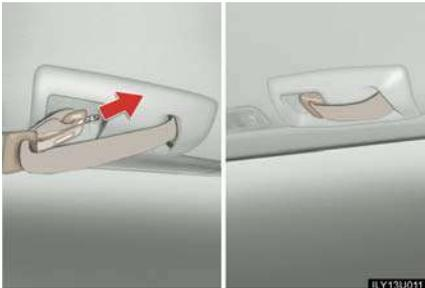
For the center seat belt, stow the seat belt tabs in the cover set in the roof as shown.
