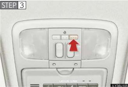
Test the operation of the HomeLink<sup>®</sup> by pressing the newly programmed button.
