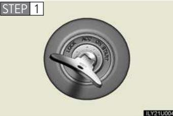
Remove the flat key from its case. Insert the key into the engine switch.
