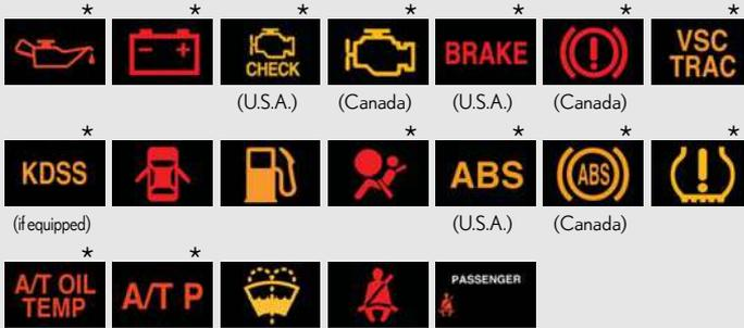
\*: These lights turn on when the engine switch is turned to the "ON" position to indicate that a system check is being performed. They will turn off after the engine is running, or after a few seconds. There may be a malfunction in a system if the lights do not come on, or turn off. Have the vehicle inspected by your Lexus dealer.
