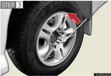
Slightly loosen the wheel nuts (one turn).
