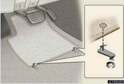
Secure the floor mat using the hooks provided.
