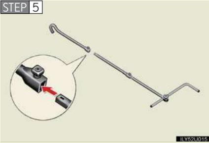
Attach the hooked jack handle end to the jack handle extension as shown.
