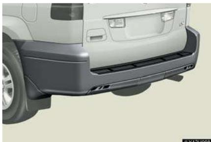
For rear end protection and easier step-up loading.
