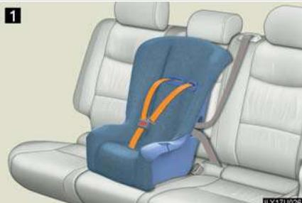
**1** Seat belts equipped with a child restraint locking mechanism (ALR/ELR belts except driver's seat belt) (→P. 52)
