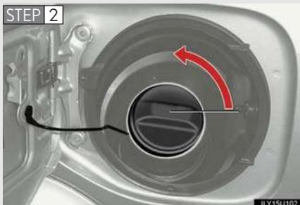
To remove the fuel tank cap, turn the cap slowly counter-clockwise, then pause slightly before removing it.
