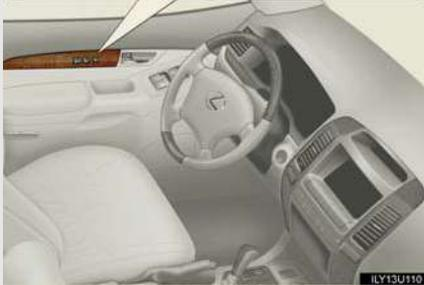
While pushing the "SET" button, push button "1" or "2" until the signal beeps.
