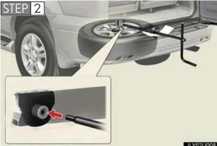
Insert the jack handle extension into the lowering socket.
