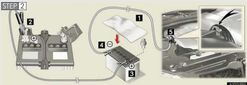
Connecting the jumper cables.
