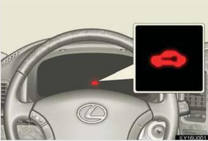
The indicator light flashes after the engine switch has been turned to the "LOCK" position to indicate that the system is operating.
