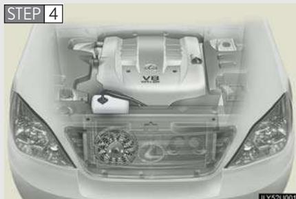
After the engine has cooled down sufficiently, check the coolant level and inspect the radiator for any leaks.
