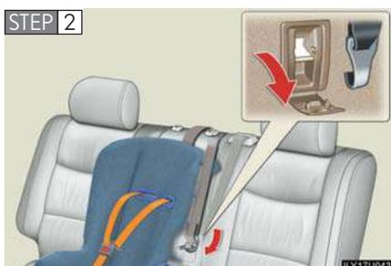
Open the anchor bracket cover, latch the hook onto the anchor bracket and tighten the top strap.
