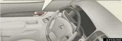
The front doors can be opened by pulling the inside handles even if the lock buttons are in the lock position.
