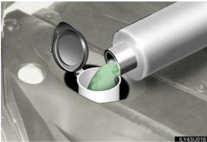
If a washer does not work, the washer tank may be empty. Add washer fluid.
