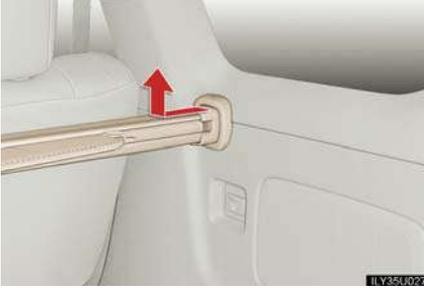
Retract the cover and release both ends, then lift it out.
