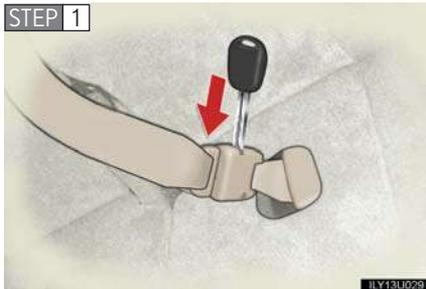
To release the hooked tab, insert the vehicle's key into the hole on the buckle with the light gray buckle release button.
