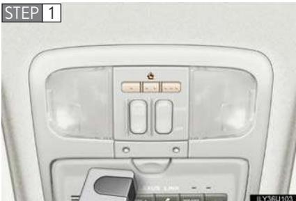
Point the remote control for the device 1 to 3 in. (25 to 75 mm) from the HomeLink® control buttons.
