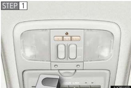
Point the remote control for the device 1 to 3 in. (25 to 75 mm) from the HomeLink<sup>®</sup> control buttons.
