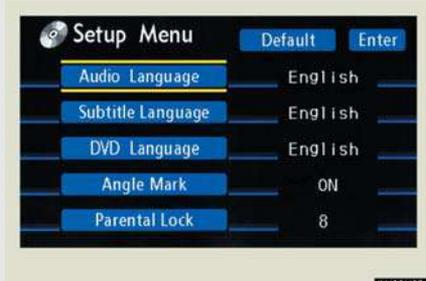
Press **SET UP** or select **Set Up** to display the initial settings screen.
