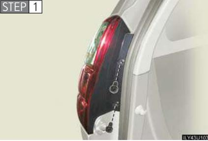
Open the back door and remove the screws.
