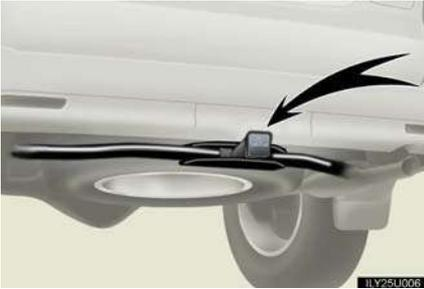
A tow hitch receiver installed under the rear bumper is rated for weight that does not exceed the vehicle's total towing weight.
