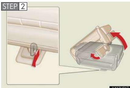
Unlock the seat legs by pulling the seat leg lock release handles, and lift the seats. Retract the seat legs, then place the seats on the floor.
