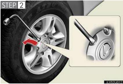
Remove the wheel ornament using the wheel nut wrench as shown.
