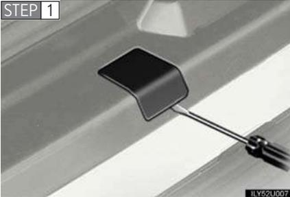
Remove the spare tire carrier lid using a flathead screwdriver.
