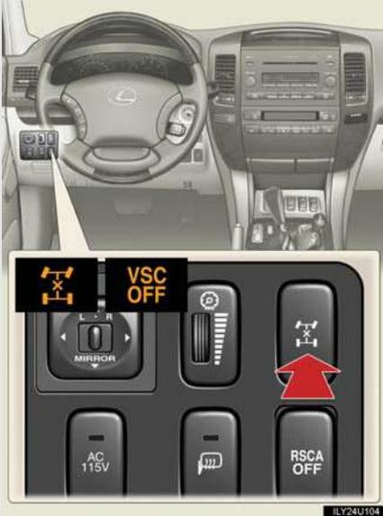
Use this button when your vehicle's wheel gets stuck in a ditch or when you are driving on a loose or bumpy surface.
