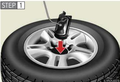
Lay down the tire with the outer side facing up, and install the holding bracket.
