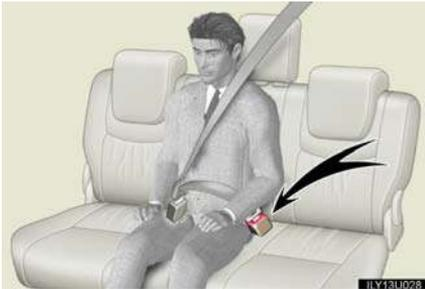
Make sure that the buckle with the light gray buckle release button is securely latched for ready use of the center seat belt.
