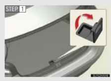
Lift up the hook and remove the panel.
