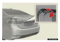
Turn the mechanical key clockwise to open.
