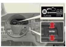
Toggle the "ENTER" switch on the steering wheel upward or downward through several items to select the energy monitor display.
