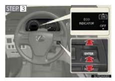
Press the "ENTER" switch upwards or downwards to select the desired setting for the item being customized and press the "ENTER" switch to confirm.
