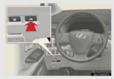
Press the opener switch to release the trunk lid.
