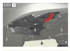
Remove the fender liner bolts, clip and remove the fender liner.
