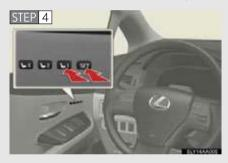
While pressing and holding the "SET" button, or within 3 seconds of pressing the "SET" button, press button 1, 2 or 3 until the signal beeps.
