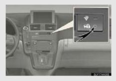
Close the doors, trunk and hood, and lock all the doors using the entry function or wireless remote control. The system will be set automatically after 30 seconds.
