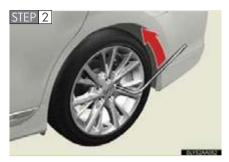
Slightly loosen the wheel nuts (one turn).
