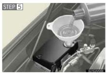
Add engine coolant if necessary.
