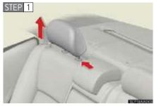
Remove the head restraint.
