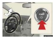
When the "POWFR" switch is turned off, the steering wheel returns to its stowed position by moving up and away to enable easier driver entry and exit.
