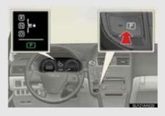
Fully stop the vehicle and keep depressing the brake pedal, and then press the P position switch.
