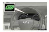
During Eco-friendly acceleration (Eco driving), Eco Driving Indicator Light will turn on. When the accelerator pedal is depressed excessively, and when the vehicle is stopped, the light turns off.
