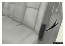
There is an air intake vent on the side of the rear left seatback for the purpose of cooling the hybrid battery (traction battery). If the vent become blocked, the hybrid battery may overheat, leading to a reduction in hybrid battery output.
