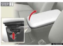
Pull up the knob to release the lock and lift the armrest.
