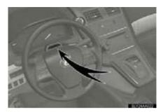
The driver monitor sensor detects the direction the driver is facing. The system determines whether the driver is facing forward.
