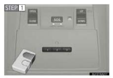
Point the remote control transmitter for the device 1 to 3 in. (25 to 75 mm) from the HomeLink  $^{\circledR}$  buttons.
