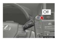
Set the wiper switch to the off position. If the wiper switch is in "AUTO", the wipers may operate and the wiper blades may be damaged.
