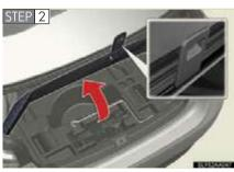
Secure the panel using the hook provided.
