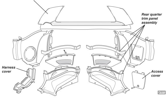
First remove the rear seat cushion or shelf, rear seat backrest or bulkhead insulation, and the rear window surround. Then:
