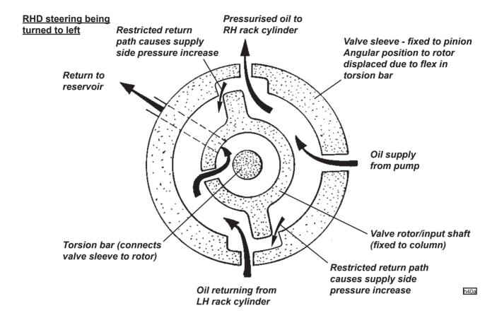
The engine driven pump supplies oil at a controlled rate. A progressive restriction of this oil flow will cause the pressure to increase whilst the flow rate is maintained. Eventually, when the flow is completely restricted, the pressure will rise to the relief valve setting in the pump, causing oil to flow through the relief valve and recirculate within the pump.
