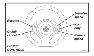
*To enable cruise control:* The system will always default to 'off' whenever the ignition is turned off. To enable cruise control, turn on the ignition, and press the on/off switch; the tell tale in the instrument panel will light to confirm that the system is enabled (although no speed has yet been set). Alternatively, this operation may be combined with that for activation, by pressing the on button followed by the set button (see below).
