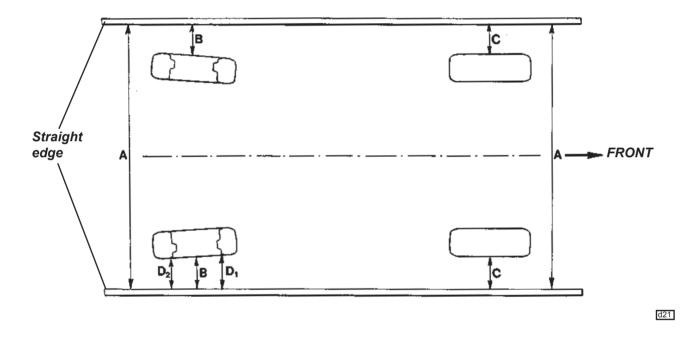
Measure the distance from the bar to the rim of the wheel concerned at the front and rear of the centre line of the wheel  $(D_1, D_2)$ . If the front dimension,  $D_1$ , is greater than the rear dimension,  $D_2$ , the wheel has TOE-IN. If the rear dimension is greater than the front dimension, the wheel has TOE-OUT. The difference between the two measurements is the amount the wheel has toe-in or toe-out.
