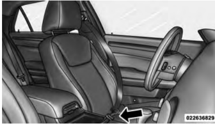
Inserting Latch Plate Into Buckle
