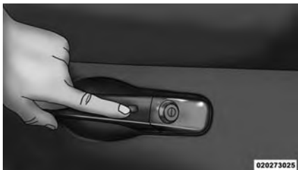
Press The Door Handle Button To Lock
