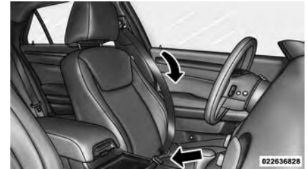
Pulling Out The Lap/Shoulder Belt Latch Plate
