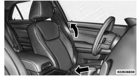
Removing Slack From Belt
