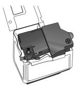
To access the battery, release the fixings and move the top of the battery cover aside as shown in illustration.
