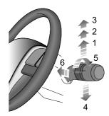
The wipers and washers will operate with the ignition in position I, i.e. Auxiliary. Push the lever up to select different wiper speeds.
