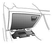
Note: The closing panel below the glove box should be removed to gain access to the fuses.
