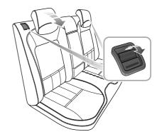
To increase luggage space, fully lower all head restraints, press either of the release catches and fold the seat backrest forward.
