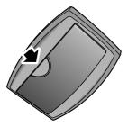
Press the switch (arrowed) to illuminate the courtesy light, press again to switch off.
