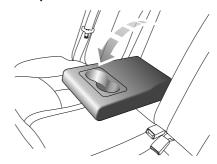
Pull the rear armrest forwards and lower into position. Raise armrest to close.
