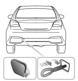
Your car is equipped with a removable towing eye, that can be used at the front or the rear of your vehicle. The towing eye is stored in the tool kit beneath the loadspace floor when not in use.
