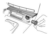
When the ignition is in position I or II, open the front ashtray cover, and pull out the socket lid to use the power socket.
