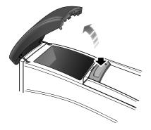
Press the release catch (arrowed) to open the lid. Push down to close.
