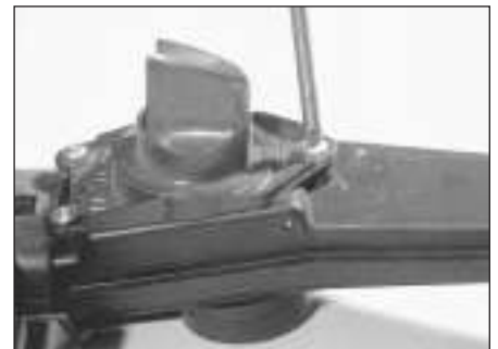
3.12 Removing the air cleaner intake duct adapter
