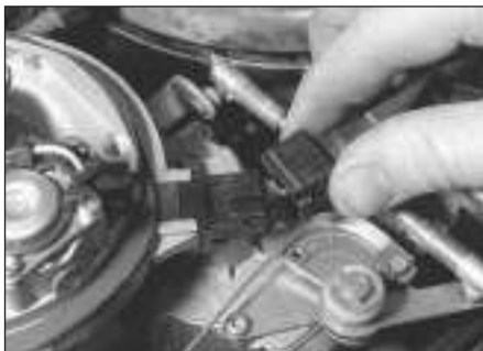
13.12 Disconnecting the injector housing wiring connector
