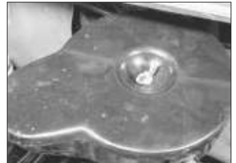
2.1a Remove the single wing nut on early models . .
