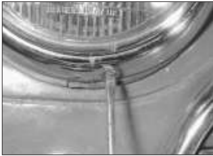
5.2b On non-Clubman models, undo the outer rim securing screw . . .
