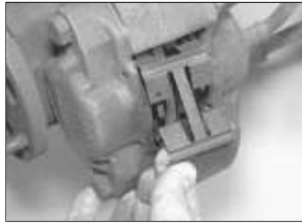
7.3a Lift away the pad retaining spring plate . . .
