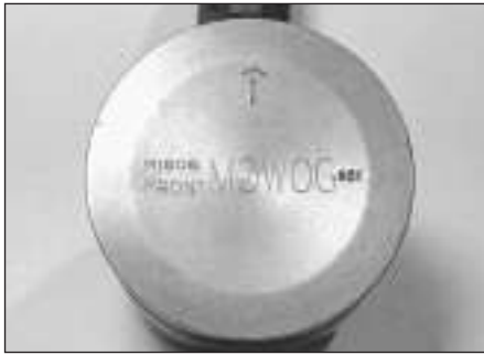
11.19 Identification markings on the piston crown
