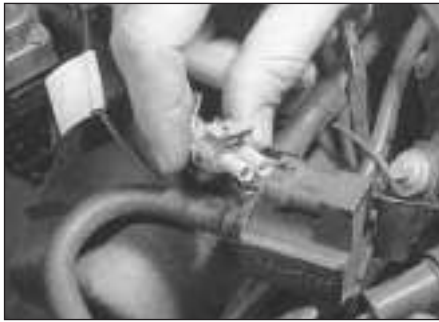
6.28 Disconnecting the purge valve wiring connector
