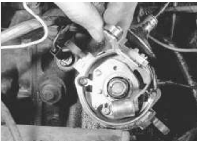
6.10a . . . and with the retaining screw removed, lift the contact assembly off the baseplate
