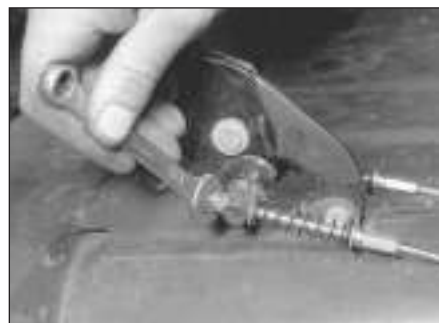
21.3 Remove the handbrake cable adjusting nuts
