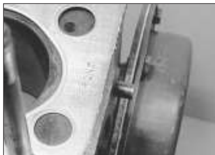
7.25a The cylinder head gasket is marked FRONT . . .
