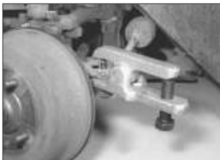
3.5 Remove the steering tie-rod balljoint with a universal separator
