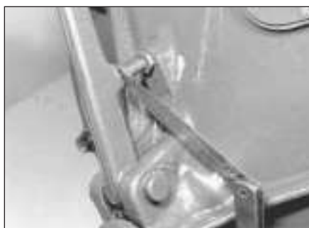
22.3 Using feeler blades to measure the clutch return stop clearance
