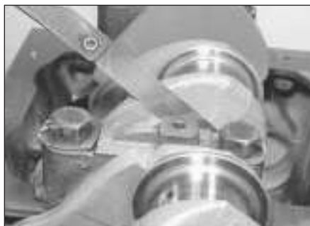
12.3 Checking crankshaft endfloat using feeler blades
