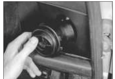
13.2 Turn the air vent anti-clockwise to remove
