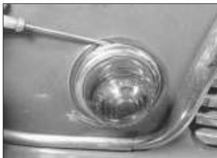
5.27a Fold back the rubber flange and remove the rim . . .
