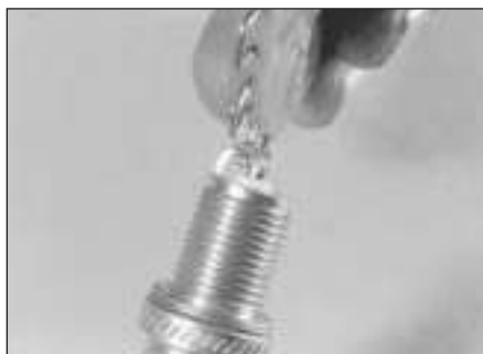
33.11 Adjusting a spark plug electrode gap
