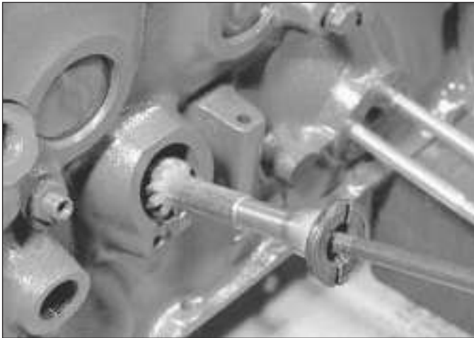
13.5 Using a 5/16 in UNF bolt to remove the distributor driveshaft
