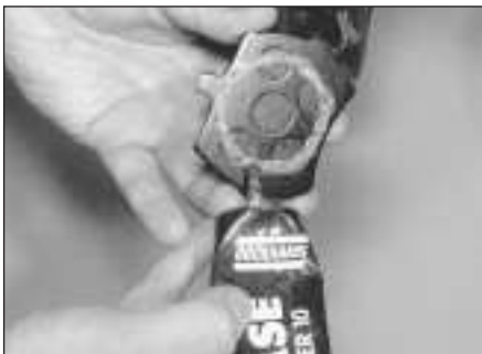
7.8 Smear high-temperature anti-seize grease to the pad backing plates
