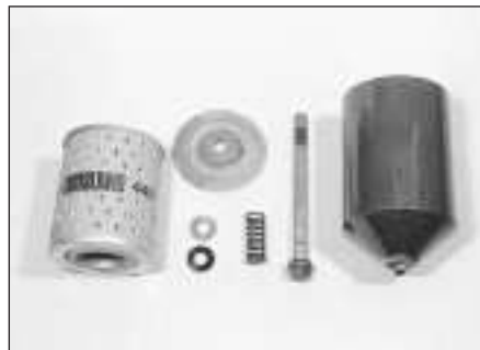
13.9 Components of the cartridge type oil filter
