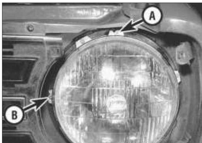
7.1 Headlight vertical position A and horizontal position B adjusting screws
