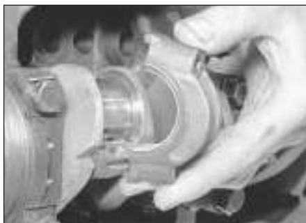
11.3 Removing a connecting rod big-end cap
