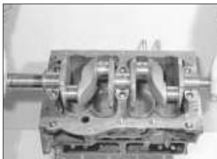
12.10 Carefully lift out the crankshaft
