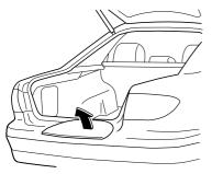
2. Turn the tire wing bolt counterclockwise.
