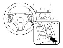
Your vehicle has a tap-down feature that allows you to decrease your current speed in decrements of 1.6 km/h (1 mph) by a momentary tap of the SET/COAST button. Multiple taps will decrease your vehicle speed 1.6 km/h (1 mph) for each tap.
