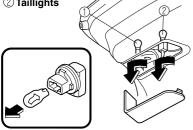
4. Install the new bulb in the reverse order of removal.
