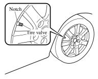
Damage could occur during installation if the wheel cover is not properly aligned.
