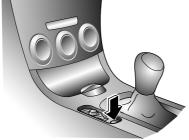
When placing the remote control back in the cradle, press it until you hear it engage.
