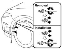
4. Turn the socket and bulb assembly counterclockwise, and carefully pull it backward.
