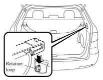
3. Slowly pull out the cover towards you and insert the cover ends into the hook retainers at the rear of the vehicle.
