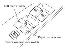
To open the power window to the desired position, hold down the switch. To close the power window to the desired position, pull up the switch.
