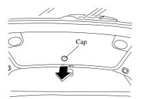
2. Turn the lever to the right to unlock the liftgate.
