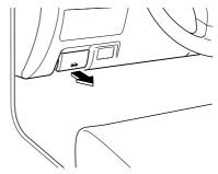
2. Insert your hand into the hood opening and slide the hood latch lever to the right and lift the hood.
