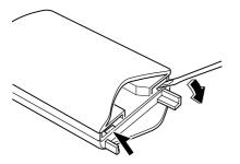
4. Press the portion of the battery indicated by A and remove the battery.
