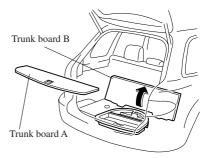
2. For vehicles equipped with a cargo sub-compartment, remove the cargo sub-compartment.
