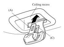
To pull out the seat belt, slide tongue (A) with your finger while moving it downward, and slowly pull out the seat belt from the ceiling recess.
