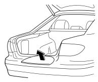
3. For vehicles equipped with a subwoofer, loosen the wing bolt and remove the woofer and spare tire.
