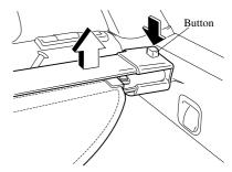
3. Remove the left end of the retainer bar from the notch.
