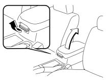
Small items can be placed in the tray of the center console lid. To open it, pull the upper release latch.
