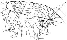
The side and curtain air bag will deploy only on the side the vehicle receives the force of the impact.
