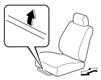
Make sure the lever returns to its original position and the seat is locked in place by attempting to push it forward and backward.
