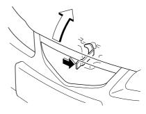
3. Grasp the support rod and secure it in the stay hole indicated by the arrow to hold the hood open.
