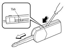
3. Insert a small screwdriver into the slot and gently pry open the transmitter.
