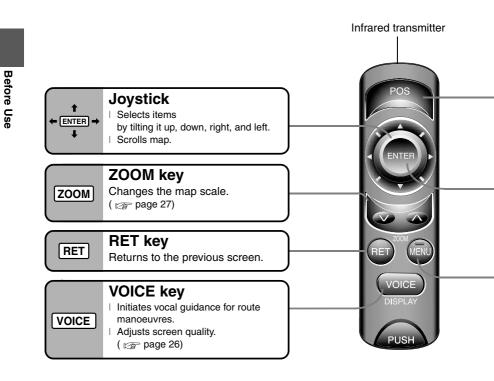
To remove the remote control from the cradle press **PUSH**
