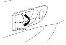
To lock any door with the door-lock knob from the outside, push the door-lock knob to the lock position and close the door. This does not operate the other door locks.
