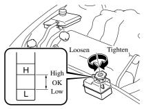
The level must be kept between the H and L marks.
