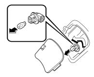
4. Install the new bulb in the reverse order of removal.
