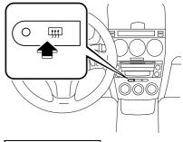
Don't use sharp instruments or window cleaners with abrasives to clean the inside of the rear window surface. They may damage the defroster grid inside the window.
