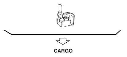
**Cargo Weight** includes all weight added to the Base Curb Weight, including cargo and optional equipment. When towing, trailer tongue load or king pin weight is also part of cargo weight.
