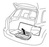
For vehicles equipped with a subwoofer, loosen the wing bolt and remove the woofer and spare tire.
