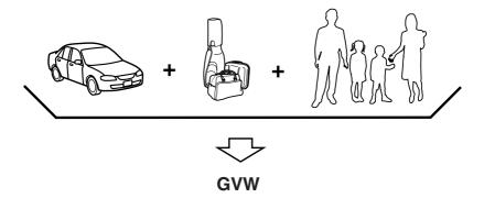
GVW (Gross Vehicle Weight) is the Vehicle Curb Weight + cargo + passengers.
