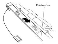
Slowly pull out the net in the upward direction, insert the left and right net anchors into the ceiling retainers, and slide them to the position indicated in the figure.
