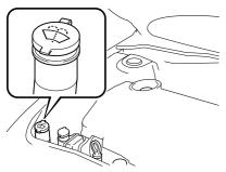
Use plain water if washer fluid is unavailable. But use only washer fluid in cold weather
