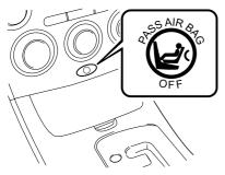
If the front passenger weight sensors are working properly, the indicator light illuminates when the ignition switch is turned to the ON position. After a specified period of time it goes out.
