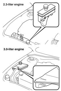
If it's at or near LOW or L, add enough coolant to the coolant reservoir to provide freezing and corrosion protection and to bring the level to FULL or F.
