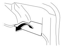
3. Turn the wing bolt and jack screw counterclockwise.
