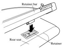
Slide the retainer bar in the direction indicated in the figure, and engage the anchors into the seatback retainers.
