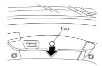
2. Turn the lever to the right to unlock the hatch.
