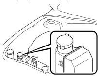
The level must be kept between MIN and MAX.
