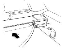
2. Press and hold the button on the right side of the retainer bar and lift the bar.
