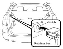
2. Set the right side of the retainer bar onto the retainer loop on the right side of the luggage compartment.
