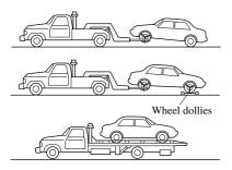
When towing with the rear wheels on the ground, release the parking brake.
