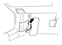
Pulling the cover off sideways may break the retaining tabs off.
