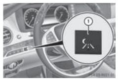
Press button ①. If Night View Assist Plus is activated, the Night View Assist Plus display is shown in the multifunction display.
