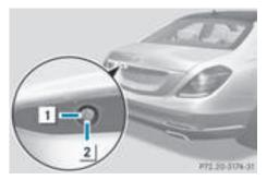
▶ Turn the mechanical key from position 1 counter-clockwise as far as it will go to position 2.
