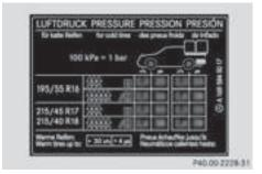
The load conditions "partially laden" and "fully laden" are defined in the table for different numbers of occupants and amounts of luggage. The actual number of seats may differ.
