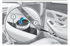
The ashtray is located in the stowage compartment in the rear door. To use it, you can place it in a cup holder or hold it in your hand.
