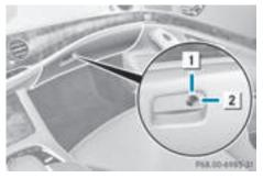
The glove box can only be locked and unlocked using the mechanical key ( $\triangleright$  page 79).
