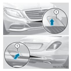
The brackets for the screw-in towing eye are located in the bumpers. They are at the rear and at the front, under covers (1).
