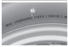
Maximum tire load ① is the maximum permissible weight for which the tire is approved. Do not overload the tires by exceeding the specified load limit. The maximum permissible load can be found on the vehicle's Tire and Loading Information placard on the B-pillar on the driver's side ( $\triangleright$  page 353).
