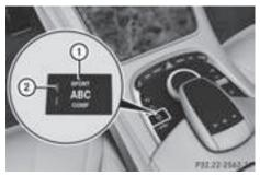
The firmer setting of the suspension tuning in SPORT mode ensures even better contact with the road. The steering response behavior is sporty. Select this mode when employing a sporty driving style on flat roads, e.g. on highways.
