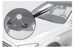
The ROAD SURFACE SCAN function monitors the road in front of the vehicle using multifunction camera (1) at the top of the windshield. This function is automatically active if you select comfort suspension tuning. The system is operational at speeds of up to 81 mph (130 km/h).
