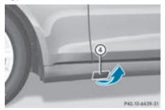
Mercedes-AMG vehicles and vehicles with AMG equipment: fold cover (4) upwards.
