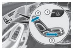
The head restraint must be installed, in order for the front-passenger seat to be moved into the normal position ( $\triangleright$  page 108).
