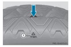
Marking ① shows where the bar indicator (arrow) for tread wear is integrated into the tire tread.
