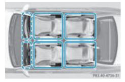
You can set the temperature separately for the following areas on vehicles with rear-compartment climate control:
