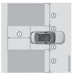
At a distance of approximately 1.6 ft (0.5 m) (2) from the vehicle, Active Blind Spot Assist monitors the area up to 10 ft (3 m) next to (3) and behind (1) your vehicle, as shown in the picture. The detection of obstacles can be impaired in the case of:
