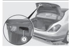
▶ Pull the trunk lid down using recess ①.
