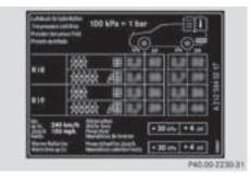
Some tire pressure tables show only the rim diameters instead of the full tire size, e.g. **R18**. Rim diameter is part of the tire size and can be found on the tire sidewall ( $\triangleright$  page 357).
