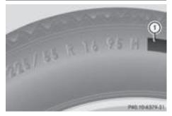
In addition to the load-bearing index, load index () may also be imprinted on the sidewall of the tire. You will find this after the letter that identifies the speed rating ( $\triangleright$  page 357).
