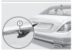
Rear view camera ① is in the trunk lid handle. Rear view camera ① is an optical parking and maneuvering aid. It shows the area behind the vehicle with guide lines in the multimedia system.
