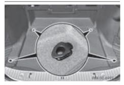
There are up to four parcel net hooks in the trunk depending on the equipment installed.
