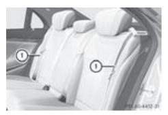
When triggered, belt bags ① open, increasing the protected area of the occupants' ribcages. The beltbags are triggered depending on the type and severity of the accident.
