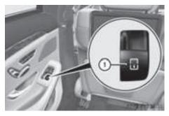
► To open/close manually: press or pull switch ① to the point of resistance and hold it until the rear roller sunblind has reached the desired position.
