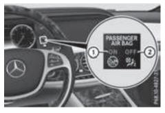
PASSENGER AIR BAG ON indicator lamp (1) and PASSENGER AIR BAG OFF indicator lamp (2) are part of the Occupant Classification System (OCS).
