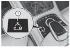
Mercedes-AMG vehicles: press program selector button (1) repeatedly until the letter for the desired drive program appears in the multifunction display.
