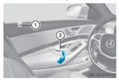
To unlock and open a front door: pull door handle (2). If the door is locked, locking knob (1) pops up.
