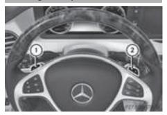
You can activate manual drive program **M** in the **E** (**C** in AMG vehicles) and **S** automatic drive programs using steering wheel paddle shifters (1) and (2) ( $\triangleright$  page 157). In manual drive program **M**, you can briefly change gear yourself by using the steering wheel paddle shifters.
