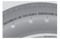
Uniform Tire Quality Grading Standards are U.S. government specifications. Their purpose is to provide drivers with uniform reliable information on tire performance data. Tire manufacturers have to grade tires using three performance factors: (1) tread wear grade, (2) traction grade and (3) temperature grade. These regulations do not apply to Canada. Nevertheless, all tires sold in North America are provided with the corresponding quality grading markings on the sidewall of the tire.
