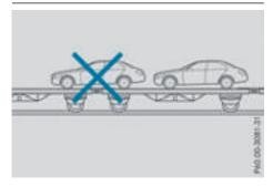
When the vehicle is loaded for transport, the front and rear axles must be stationary and on the same transportation vehicle. Positioning over the connection point of the transport vehicle is not permitted. The drive train may otherwise be damaged.
