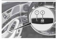
▶ To activate/deactivate:press button ②. If indicator lamp ① is lit, operation of the rear side windows is disabled. Operation is only possible using the switches in the driver's door. If indicator lamp ① is off, operation is possible using the switches in the rear compartment. When the override feature is activated, the controls in the rear compartment are disabled for:
