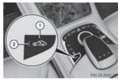
It is possible to choose between the "Normal" and "Raised" vehicle levels. Select the "Normal" setting for normal road surfaces and "Raised" for driving with snow chains or on particularly poor road surfaces. Your selection remains stored even if you remove the SmartKey from the ignition lock.
