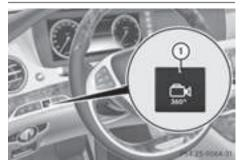
► To switch on: press button ①. Depending on whether position D or R is engaged, the following is shown:
