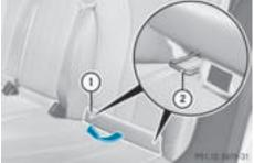
LATCH-type (ISOFIX) securing rings ② on the rear seats are covered by a Velcro-fastened upholstered lining ①.
