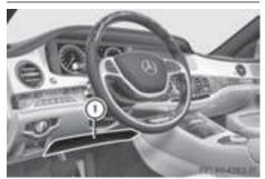
Driver's knee bag ① deploys under the steering column. The driver's knee bag is always deployed along with the driver's front air bag. The driver's knee bag offers additional thigh, knee and lower leg protection for the occupant in the driver's seat.
