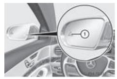
Active Blind Spot Assist is not operational at speeds below approximately 20 mph (30 km/h). Vehicles in the monitoring range are then not indicated.
