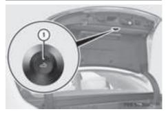
You can unlock the trunk lid from the inside using emergency release button (1).
