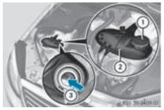
Example: checking the coolant level
