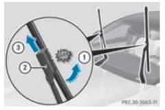
► To bring the wiper blade into the removal position: hold onto the wiper arm with one hand. With the other hand, turn the wiper blade in the direction of arrow ① beyond the point of resistance.
