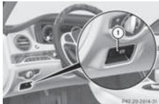
► To engage: push handle ①. When the electric parking brake is applied, the red PARK (USA only) or (②) (Canada only) indicator lamp lights up in the instrument cluster.
