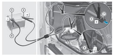
Position number (3) identifies the charged battery of the other vehicle or an equivalent jump-starting device.
