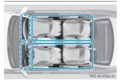
You can set the temperature separately for the following areas on vehicles without rear-compartment climate control:
