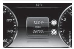
Press and hold the <u>button</u> button on the steering wheel until the Trip menu with trip odometer (1) and odometer (2) appears.
