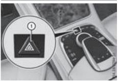
► To switch the hazard warning lamps on or off: press button ①.
