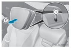
The supplementary cushion is in the vehicle. The supplementary cushion is attached to the head restraint by three press studs.
