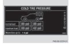
The tire pressure table contains the recommended pressures for cold tires for various operating conditions, i.e. differing load and speed conditions.
