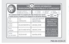
Specification for maximum gross vehicle weight ① is listed in the Tire and Loading Information placard: "The combined weight of occupants and cargo should never exceed XXX kilograms or XXX lbs."
