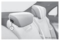
Press and hold button ① until the head restraint has fully extended or retracted.
