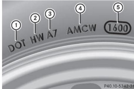
The TIN is a unique identification number. The TIN enables the tire manufacturers to inform purchasers of recalls and other safety-relevant matters. It makes it possible for the purchaser to easily identify the affected tires. The TIN is made up of manufacturer identification code ②, tire size ③, tire type code ④ and manufacturing date ⑤.
