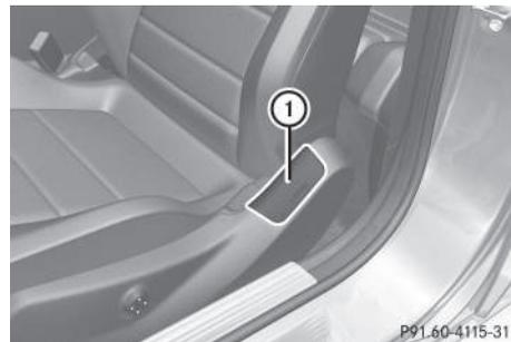
Pelvis air bags ① deploy next to and below the outer seat cushions. They are deployed:
