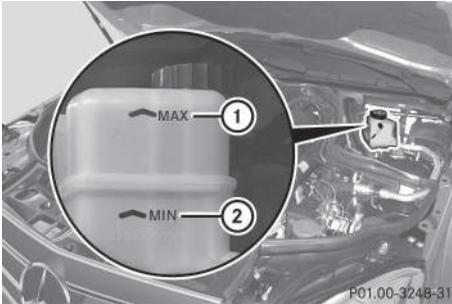
If the brake fluid level is between MIN marking ② and MAX marking ① on the brake fluid reservoir, it is correct.
