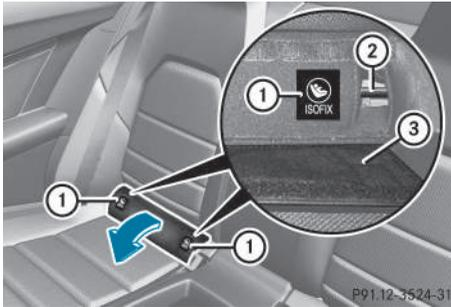
Installation instructions ① indicate the installation location of securing rings ②.
