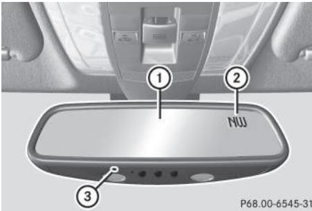
To obtain a correct display in rear-view mirror ①, the compass must be calibrated and the magnetic field zone must be set.
