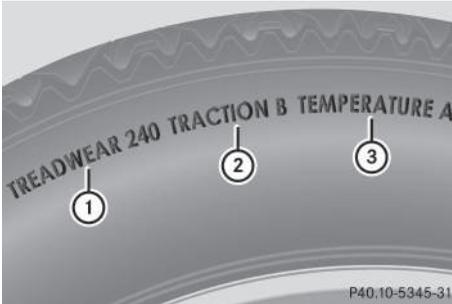
Uniform Tire Quality Grading Standards are U.S. government specifications. Their purpose is to provide drivers with uniform reliable information on tire performance data. Tire manufacturers have to grade tires using three performance factors: tread wear ①, tire traction ②, and heat resistance ③. All tires sold in North America are provided with the corresponding quality class mark on the sidewall of the tire, even though these regulations do not apply to Canada.
