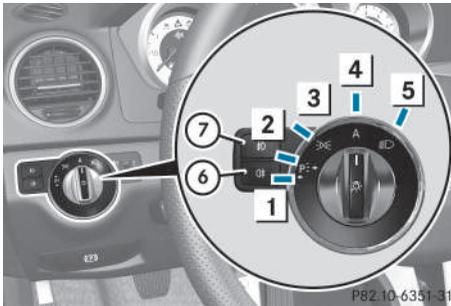
Illustration: light switch with the **A** symbol for the automatic headlamp mode/daytime running lamps
