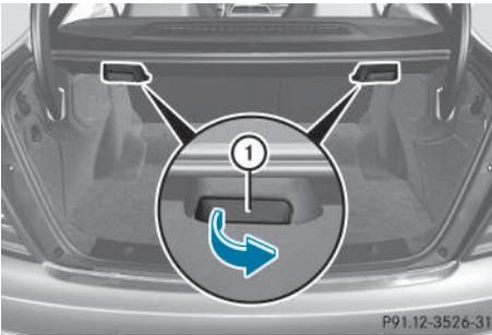
**i** Vehicles with memory function: when you fold one or both parts of the rear seat backrest forwards, the respective front seat moves forward slightly, when necessary, in order to avoid contact.
