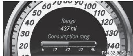
The approximate range that can be covered depends on the fuel level and your current driving style. If there is only a small amount of fuel left in the fuel tank, the display shows a vehicle being refueled instead of the range.
