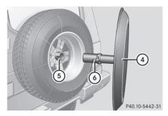
(1) When refitting cover panel (4), make sure that retainer (6) engages in recess (5).
