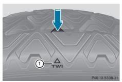
Indicator (1) for tread wear is integrated into the tire tread.
