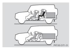
The gross vehicle weight (GVW) is the vehicle weight including fuel, vehicle tool kit, spare wheel, installed accessories, vehicle occupants and luggage/cargo.
