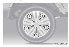
▶ Tighten the wheel bolts evenly in a crosswise pattern in the sequence indicated (1) to (5). The tightening torque must be 96 lb-ft (130 Nm).
