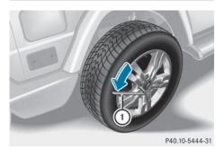
► Using lug wrench ①, loosen the bolts on the wheel you wish to change by about one full turn. Do not unscrew the wheel bolts completely.
