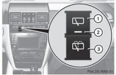
The rear window wiper comes on automatically if you shift the selector lever to **R** while the windshield wipers are on.
