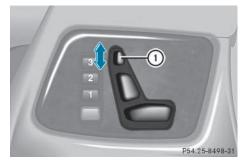
▶ Slide head restraint adjustment button ① up or down in the direction of the arrow.
