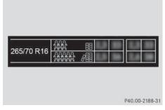
Tire pressure table with tire dimensions (example) Some tire pressure tables only show the rim diameter instead of the complete tire size, e.g. **R16**. The rim diameter is part of the tire size and can be found on the tire sidewall (⊳ page 259).
