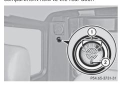
The warning display is divided into four yellow and two red segments ①. The ultrasonic backing up aid is ready for use when you hear a warning tone and segment ② lights up briefly.
