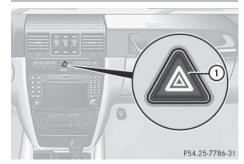
The hazard warning lamps switch on automatically if an air bag or the Emergency Tensioning Devices are triggered and the SmartKey is in position 1 in the ignition lock.
