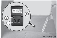
115 V power socket ① provides an alternating voltage of 115 V, so that small electronic devices can be connected. These devices, such as game consoles, chargers and laptops, should not consume more than a maximum of 150 W altogether.
