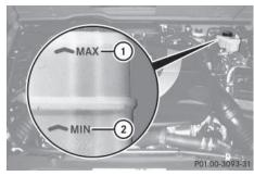
The brake fluid level is correct if it is between MIN marking ② and MAX marking ① on the brake fluid reservoir.
