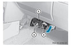
To make it easier to change the fuse, you can fold fuse box (5) down slightly:
