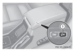
▶ Press and hold Roadside Assistance button ① for more than two seconds. A call to a Mercedes-Benz Roadside Assistance Representative is initiated. The indicator lamp in Roadside Assistance button ① flashes while the call is active. The Connecting call message appears on the multifunction display and the COMAND system is muted.
