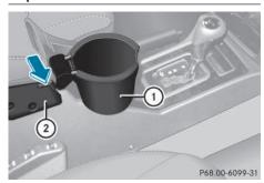
▶ Insert cup holder (1) as shown with the arrow into the fixture of carrier bar (2).
