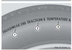
The Uniform Tire Quality Grading Standards are U.S. government specifications. Their purpose is to provide drivers with uniform reliable information on tire performance data. Tire manufacturers have to grade tires using three performance factors: tread wear (1), tire traction (2), and heat resistance (3). All tires sold in North America are provided with the corresponding quality grading markings
