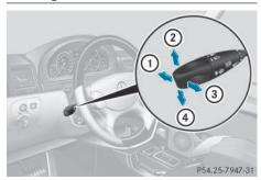
➤ To indicate briefly: press the combination switch briefly to the pressure point in the direction of arrow ② or ④.
