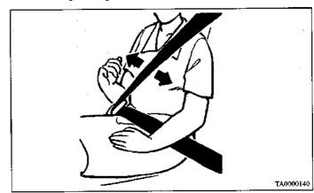
6. To release the belt, push the button on the buckle. The belt retracts automatically, so hold the tongue when the belt is released and while it retracts. If the belt does not fully return to its stowed position, pull the shoulder belt down slightly, then release it quickly.
