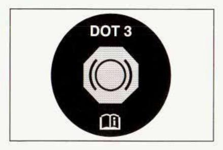
Your master cylinder reservoir is on the driver's side of the engine compartment. It is filled with DOT-3 brake fluid. See Engine Compartment Overview on page 5-14.
