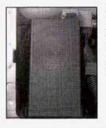
The engine compartment fuse block is located near the front on the passenger's side of the vehicle. See Engine Compartment Overview on page 5-14 for more information on location.
