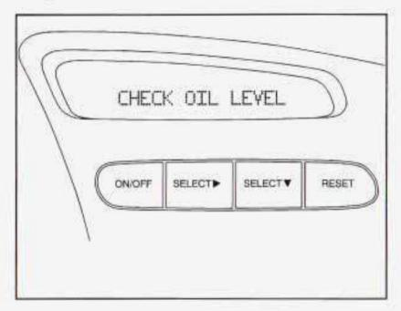
If the CHECK OIL LEVEL message appears on the instrument cluster, it means you need to check your engine oil level right away. For more information, see *DIC Warnings and Messages on page 3-50*.
