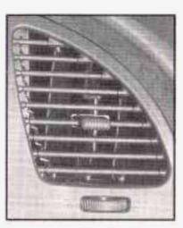
Use the lever located in the center of each front outlet to change the direction of the airflow. Use the thumbwheel located below each front outlet to turn the outlets on and off.
