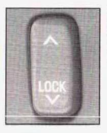
With power door locks, you can lock or unlock all the doors on your vehicle using the driver's or the front passenger's door lock switch.
