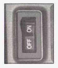
The trunk release lockout switch in the glove box allows you to secure items in the trunk, and disable the fuel door release and the HomeLink<sup>®</sup> Transmitter.
