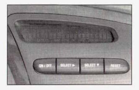
The DIC has different display modes which can be accessed by pressing the four buttons on the DIC. These buttons are labeled ON/OFF, SELECT right arrow, SELECT down arrow and RESET. The functions of these buttons is explained in the following sections.
