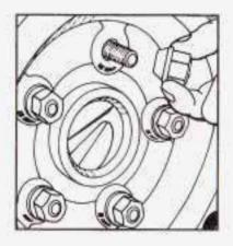
Put the wheel nuts back on with the rounded end of the nuts toward the wheel. Tighten each nut by hand until the wheel is held against the hub.
