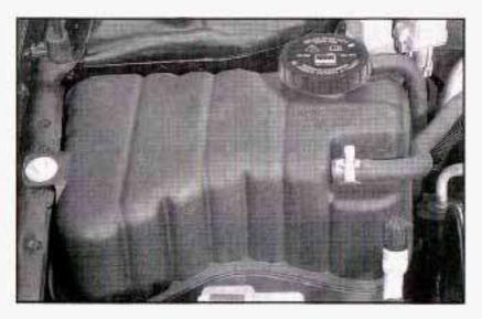
A low coolant level should be indicated by a LOW ENGINE COOLANT message on the Driver Information Center. If it is, you may have a leak at the pressure cap or in the radiator hoses, heater hoses, radiator, water pump or somewhere else in the cooling system.
