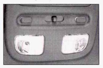
These lamps and the interior courtesy lamps will come on when you open a door. They will turn off when you turn on the ignition. If a door is left open, they will turn off after about 10 minutes.
