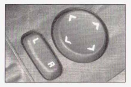
The controls for the outside power mirrors are located on the driver's door armrest.
