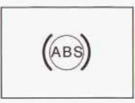
With the anti-lock brake system, the light(s) will come on when your engine is started and may stay on for several seconds. That's normal.
