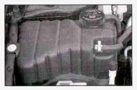
The engine coolant surge tank is located in the engine compartment on the passenger's side of the vehicle, near the windshield. See Engine Compartment Overview on page 5-14 for more information on location.
