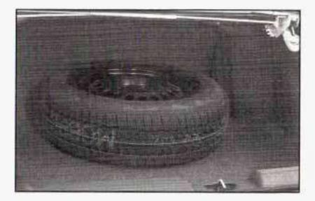
Store the flat tire as far forward in the trunk as possible. Store the jack and wheel wrench in their compartment in the trunk. For storage, the jack must be raised until the screw end is flush with the edge of the jack.
