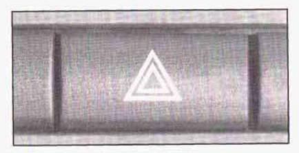
The hazard warning flasher button is located in the center of the instrument panel.
