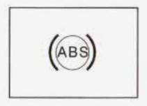
If there's a problem with the anti-lock brake system, this warning light will stay on. See Anti-Lock Brake System Warning Light on page 3-36.
