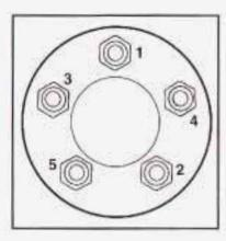
Using the wheel wrench, tighten the wheel nuts firmly in a crisscross sequence as shown.
