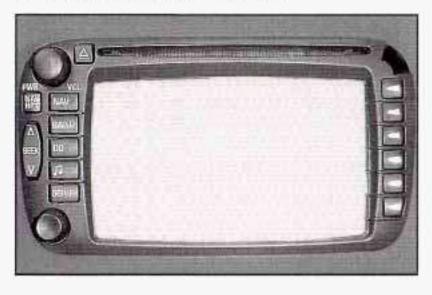
Your vehicle may have the optional navigation radio system that includes Radio Data System (RDS) which will seek out the kind of music you want to listen to. The radio system can also communicate with your navigation system to broadcast announcements on traffic and emergency alert communications. For information on how to use this system, see the "Navigation/Radio System" supplement.
