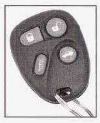
(Unlock): The driver's door will unlock and the exterior lights will flash twice when this button is pressed.
