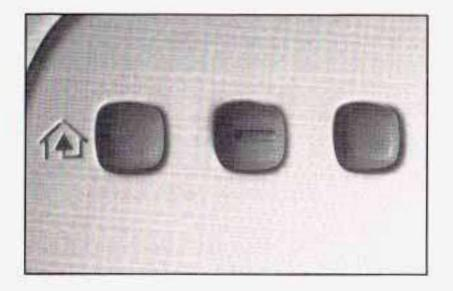
HomeLink<sup>®</sup>, a combined universal transmitter and receiver, provides a way to replace up to three hand-held transmitters used to activate devices such as gate operators, garage door openers, entry door locks, security systems and home lighting. Additional HomeLink<sup>®</sup> information can be found on the internet at www.homelink.com or by calling 1-800-355-3515.
