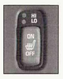
If your vehicle has this option, the heated seat switch is located next to the console shifter.
