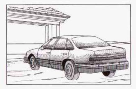
Turn on the low-beam headlamps and place a piece of cardboard or equivalent in front of the headlamp not being aimed. This should allow only the beam of light from the headlamp being aimed to be seen on the flat surface.
