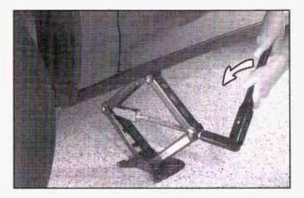
Turn the wheel wrench counterclockwise by hand to lower the jack head until it fits under the vehicle.
