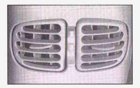
Move the control between the rear outlets up to direct airflow through the upper outlets. Move the control down to direct airflow through the floor outlets. Adjust the direction of the airflow with the levers located in the center of each rear outlet.
