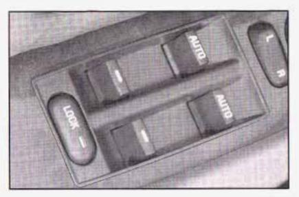
Switches on the driver's door armrest control each of the windows while the ignition is on or when Retained Accessory Power (RAP) is active. In addition, each passenger's door armrest has a separate window switch.
