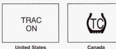
When your traction control system is limiting wheel spin, this light will come on. Slippery road conditions may exist if the traction control system active light comes on, so adjust your driving accordingly.
