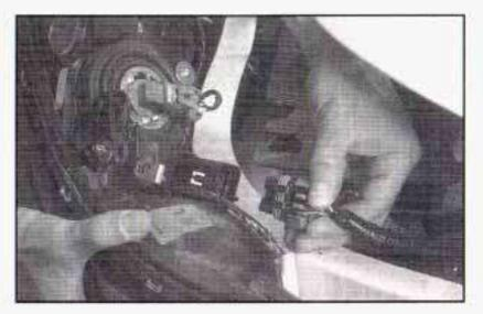
Disconnect the wiring harness from the headlamp assembly.
