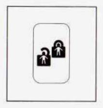
Your vehicle is equipped with rear door security locks that prevent passengers from opening the rear doors of your vehicle from the inside.
