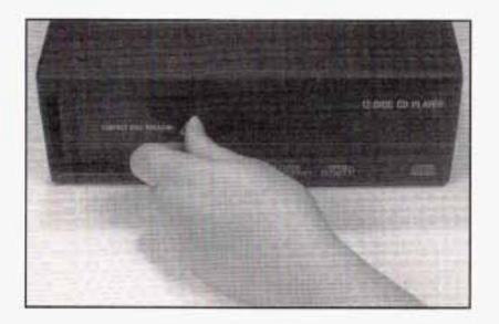
Close the door by sliding it all the way to the right. If the door is left partially open, the changer will not operate and an error will occur. When the door is closed, the changer will begin checking for discs in the magazine. This will continue for up to two minutes depending on the number of discs loaded.
