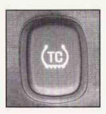
To turn the system off, press the TC button on the center console.
