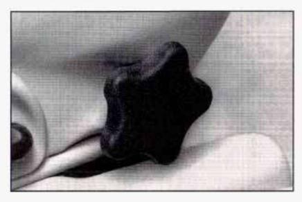
If your vehicle has this feature, the knob that controls it is located on the outboard side of the driver's seat. Turn the knob toward the front of the vehicle to increase lumbar support. Turn the knob toward the rear of the vehicle to decrease lumbar support.
