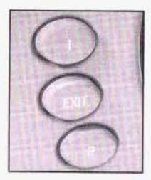
If your vehicle has this feature, the controls are located on the driver's door panel, and are used to program and recall memory settings for the driver's seating, outside mirror positions and climate controls. See Automatic Climate Control System on page 3-23 for more information.
