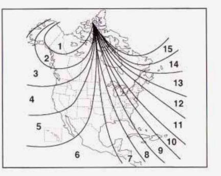
3. Once a zone number appears in the display, press the COMPASS button (or the on/off button for mirrors equipped with OnStar<sup>®</sup> controls) quickly until the correct zone number appears in the display. Stop pressing the button and the mirror will return to normal operation. If C appears in the compass window, the compass may need calibration. See "Compass Calibration" explained previously.
