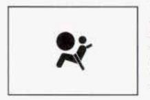
This light will come on when you start your vehicle, and it will flash for several seconds. Then the light should go out. This means the system is ready.
