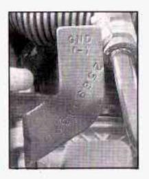
Connect the other end of the negative (-) cable at least 18 inches (45 cm) away from the dead battery, but not near engine parts that move.
