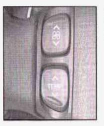
With this feature some heating and cooling controls can be adjusted at the steering wheel.  $\land \Re \lor$  (Fan): Press the up or down arrow on the fan button to override the automatic fan control and increase or decrease the fan speed.
