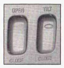
If your vehicle has this option, the switches are located on the headliner between the sun visors.
