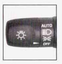
The lever on the left side of the steering column operates the exterior lamps.
