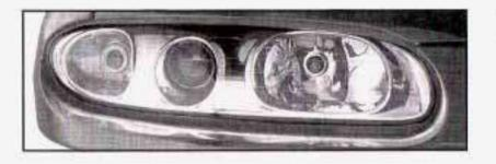
Your vehicle has a visual optical headlamp aiming system equipped with horizontal aim indicators. The aim has been preset at the factory and should need no further adjustment. This is true even though your horizontal aim indicators may not fall exactly on the "0" (zero) marks on their scales.
