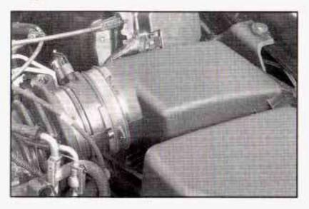
The engine air cleaner/filter is in the engine compartment on the driver's side of the vehicle. See Engine Compartment Overview on page 5-14 for more information on location.
