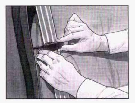
Slide the guide under and past the belt. The elastic cord must be under the belt. Then, place the guide over the belt, and insert the two edges of the belt into the slots of the guide.
