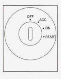
With the ignition key in the ignition switch, you can turn the switch to four different positions.
