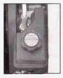
The power steering fluid reservoir is near the center of the engine compartment on the passenger's side of the vehicle. See Engine Compartment Overview on page 5-14 for more information on location.
