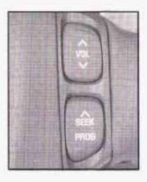
With this feature, you can control certain radio functions using the buttons on your steering wheel.
