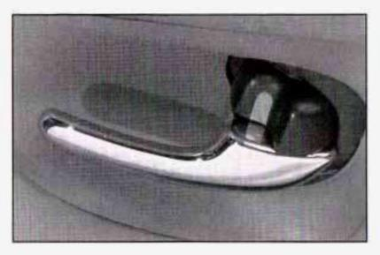
To unlock a door from the inside, move the manual door lock control, located above the door handle, rearward. To lock the door, move the manual door lock control forward.
