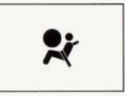
There is an air bag readiness light on the instrument panel, which shows the air bag symbol.
