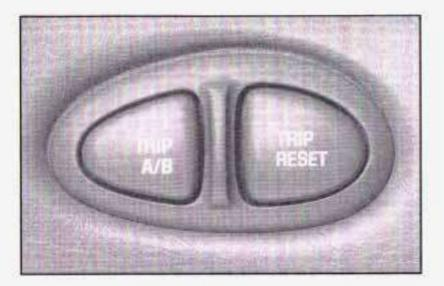
Press and hold the TRIP RESET button to reset the trip odometer that is currently being displayed.
