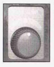
The knob for this feature is located on the passenger's door. Turn the knob clockwise or counterclockwise to a warmer or cooler setting.
