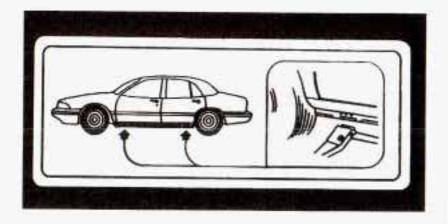
4. Near each wheel well is a notch in the frame to position the jack head. Position the jack under the vehicle and raise the jack head until it fits firmly against the sheet metal. Do not raise the vehicle yet. Put the compact spare tire near you.
