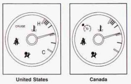
This gage shows the engine coolant temperature. If the gage pointer moves into the shaded warning zone, your engine is hot.
