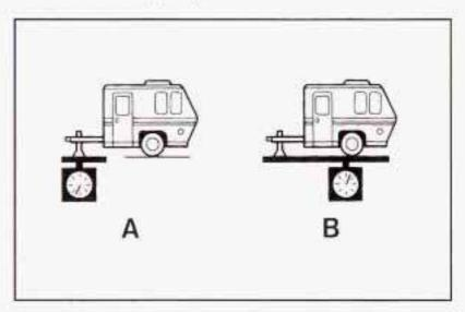
If you're using a weight-carrying hitch or a weight-distributing hitch, the trailer tongue (A) should weigh 10–15 percent of the total loaded trailer weight (B). After you've loaded your trailer, weigh the trailer and then the tongue, separately, to see if the weights are proper. If they aren't, you may be able to get them right simply by moving some items around in the trailer.
