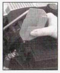
To access the remote positive (+) terminal, remove the cover. You will not see the battery of your vehicle under the hood. It is located under the rear passenger seat. You will not need to access the battery for jump starting. The remote positive (+) terminal is for that purpose.
