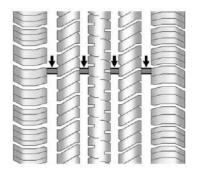
Treadwear indicators are one way to tell when it is time for new tires. Treadwear indicators appear when the tires have only 1.6 mm (1/16 in) or less of tread remaining. See *Tire Inspection*
