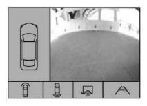
If equipped, a view of the area in front of the vehicle displays. The view displays after shifting from R (Reverse) to a forward gear, or by touching CAMERA in the infotainment display, and when the vehicle is moving forward slower than 8 km/h (5 mph). If equipped, the Front Vision Camera also displays when the Parking Assist system detects an object within 30 cm (12 in).
