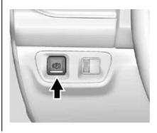
The Electric Parking Brake (EPB) switch is on the instrument panel, to the left of the steering wheel. The EPB can always be activated, even if the ignition is off. To prevent draining the battery, avoid repeated cycles of the EPB when the engine is not running.
