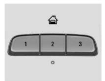
If equipped, the Universal Home Remote System allows for garage door openers, security systems, and home automation devices to be programmed to work with these buttons in the vehicle.
