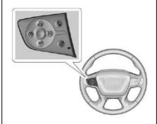
(S): Press to turn the system on or off. The indicator turns white on the instrument cluster when ACC is turned on.
