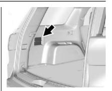
The second row seatbacks can also be folded forward by pulling the levers located on the drivers side of the rear cargo area. The top lever folds the drivers side seatback and the bottom lever folds the passenger side seatback.
