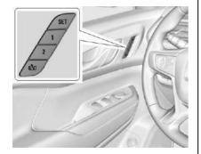
If equipped, the SET, 1, 2, and (Exit) buttons on the driver door are used to manually store and recall memory settings for the driver seat. The driver memory buttons also store outside mirror, and power tilt and telescoping steering wheel positions (if equipped).
