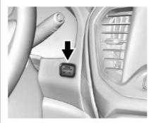
Vehicles with Keyless Access have pushbutton starting.
