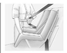
4. Pull the shoulder belt all the way out of the retractor to set the lock. When the retractor lock is set, the shoulder belt can be tightened but not pulled out of the retractor.
