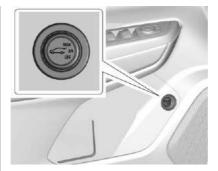
If equipped with a power liftgate, the switch is on the driver door. The vehicle must be in P (Park).
