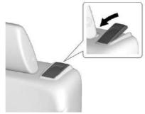
The second row seat can be folded to access the third row. Pull the handle located on top of the seat and slide the seat forward.
