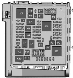
**Engine Compartment Fuse Block**
