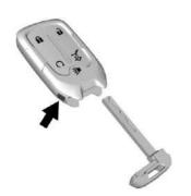
To remove the key, press the button near the bottom of the transmitter, and pull the key out. Never pull the key out without pressing the button.
