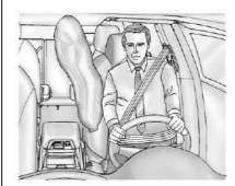
The front center airbag is in the inboard side of the driver seatback.
