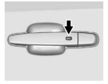
If equipped, press the button on the driver door handle when the RKE transmitter is within 1 m (3 ft) of the driver door handle. When unlocking from the driver door, the first press unlocks that door; press again within five seconds to unlock all passenger doors. See Remote Keyless Entry (RKE) System Operation ⇒ 29.
