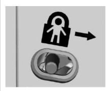
If equipped, the safety lock is on the inside edge of the rear doors. To use the safety lock:
