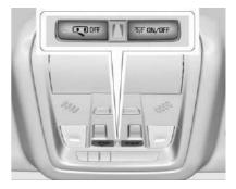
The dome lamp is in the overhead console.
