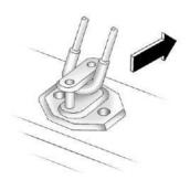
Make sure the metal tube is centered at the striker. Push the tube toward the front of the vehicle.
