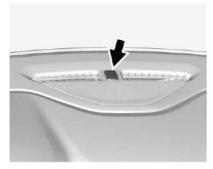
The solar sensor, located in the defrost grille in the middle of the instrument panel, monitors the solar heat. Do not cover the solar sensor or the system will not work properly.
