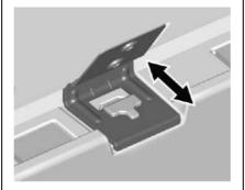
4. Unsnap the hinges on the load floor from the cargo management system.
