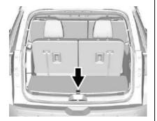
There is storage in the floor of the rear cargo area. Lift the handle to access the removable cargo management system.
