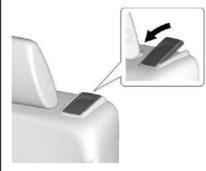
3. Pull the handle on top of the seat forward and pull the seat forward.
