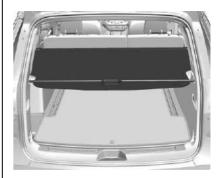
For vehicles with a cargo cover, it can be used to cover items in the rear of the vehicle. Unroll the cover toward the rear of the vehicle. Insert the cover pins into the channels on both sides. To store, carefully remove the cover from the channels and let it roll back up. The cover should be stored securely when not in use.
