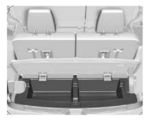
Lift the load floor to access the cargo management system, if equipped with the tray option.
