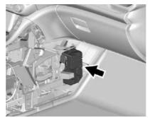
Remove the bolt cap and the screw that attaches the console side trim. Then remove the console side trim to access the fuse block.
