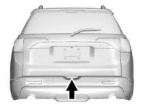
To unlock the liftgate, press on the power door lock switch or press on the RKE transmitter twice to unlock all doors. Press the touch pad on the bottom of the liftgate and lift up.
