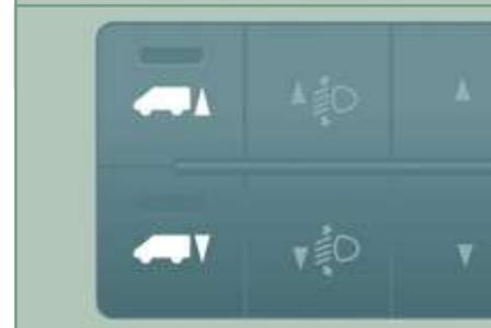
This equipment allows you to alter the rear height of the load floor to make loading or unloading easier.
