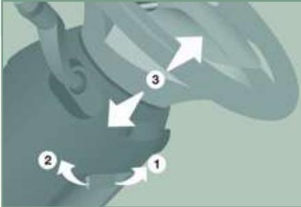
1. Unlocking the adjustment mechanism.
