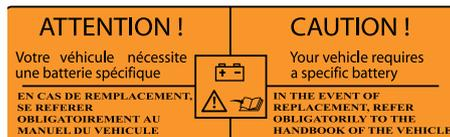
The presence of this label, in particular with the Stop & Start system, indicates the use of a specific 12 V lead-acid battery with special technology and specification. The involvement of a PEUGEOT dealer or a qualified workshop is essential when replacing or disconnecting the battery.
