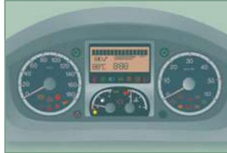
With the ignition on, the orange and red warning lamps come on.
