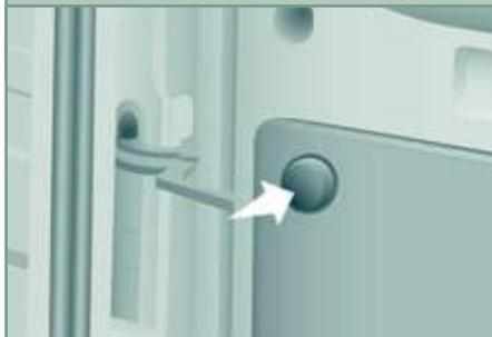
Press the button, located on the door trim panel, to widen the angle of opening of the door.
