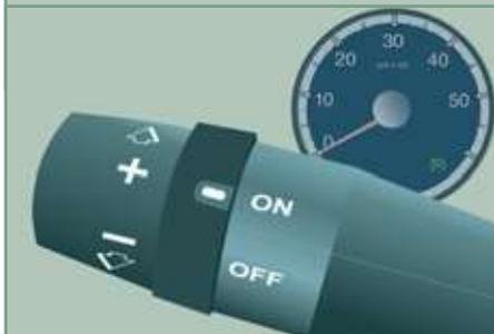
The state of the cruise control system is given on the instrument panel by a warning lamp located in the rev counter.
