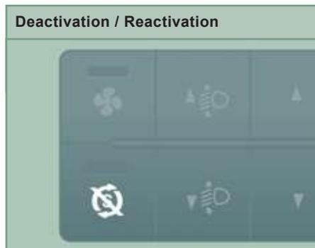
You can deactivate the system at any time by pressing the "S - OFF" control; the lamp in the button comes on, accompanied by a message in the instrument panel screen. The system is reactivated automatically at every new start with the key.
