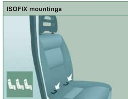
Two front rings, located between the seat back and the seat cushion are used to secure an ISOFIX child seat.
