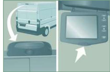
The camera comes on when you engage reverse gear and remains active up to approximately 9 mph (15 km/h). It is deactivated above 11 mph (18 km/h).
