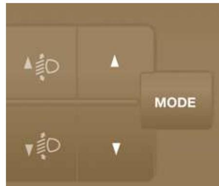
If your vehicle is fitted with this function, the passenger airbag must be deactivated using the trip computer MODE button.
