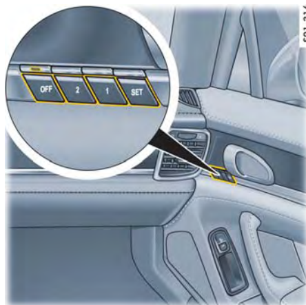
Passenger's door memory buttons (comfort memory)
