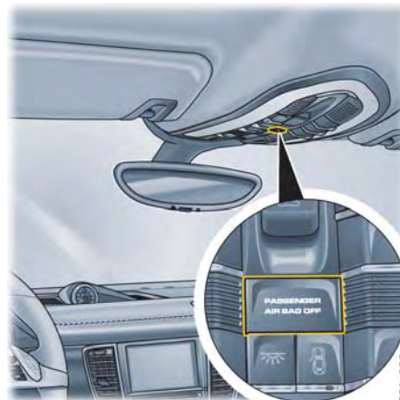
PASSENGER AIR BAG OFF indicator lamp
