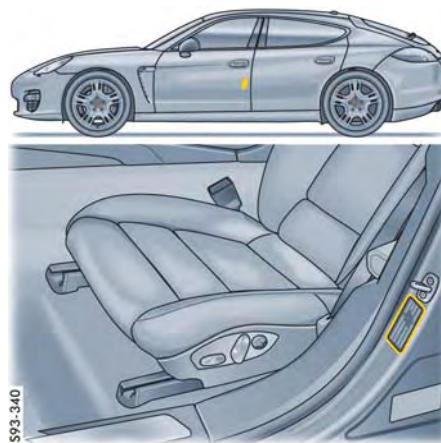
Safety compliance sticker
