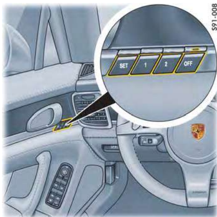
Driver's door memory buttons (driver memory or comfort memory)
