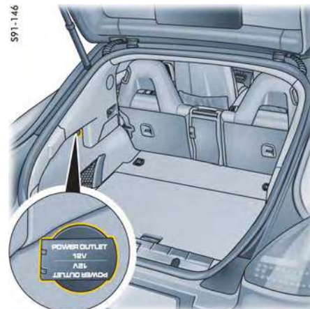
Plug socket in the luggage compartment
