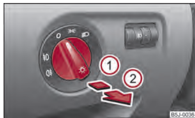
Fig. 23 Dash panel: Light switch
