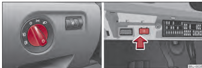
Fig. 22 Dash panel: Light switch/fuse box: Switch for daylight driving lights
