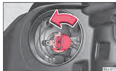
Fig. 160 Removing the light bulb for the main beam light
