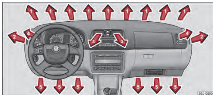
Fig. 77 Air outlet vents
