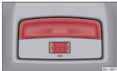
Fig. 28 Interior lighting - version 2
