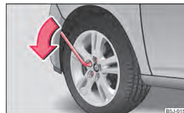
Fig. 142 Changing a wheel: Loosening the wheel bolts
