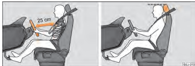
Fig. 96 The correct distance of the driver from the steering wheel/The correct head restraint adjustment for the driver
