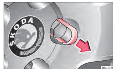
Fig. 141 Changing a wheel: Pull off cap from the wheel bolt
