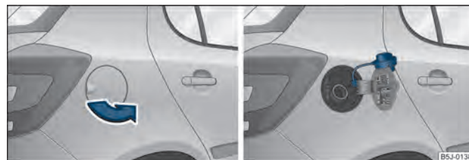
Fig. 125 Right rear side of the vehicle: Fuel filler flap/fuel filler cap with cap unscrewed
