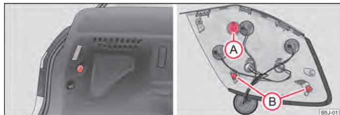
Fig. 165 Remove the rear light unit/install the rear light unit
