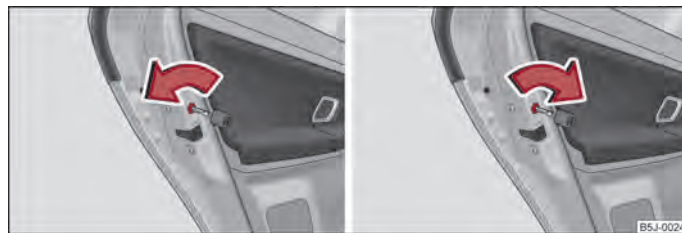
Fig. 11 Switching child safety lock on: for vehicles without or with central locking system
