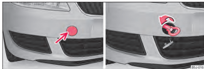
Fig. 149 Front bumper: Cover/installing the towing eye
