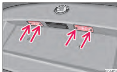
Fig. 164 Remove the licence plate light
