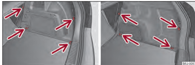
Fig. 44 Luggage compartment: Lashing eyes and fastening elements (Fabia)/(Combi)
