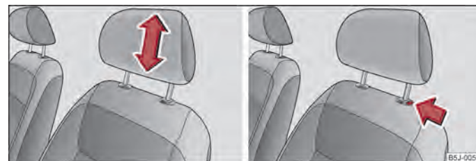
Fig. 39 Head restraint: Adjusting/pulling out
