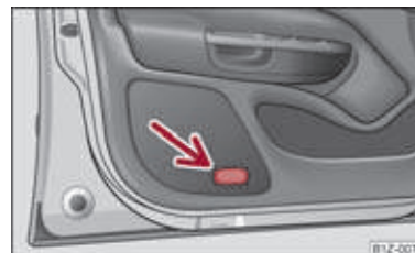
Fig. 33 Front door: Warning light
