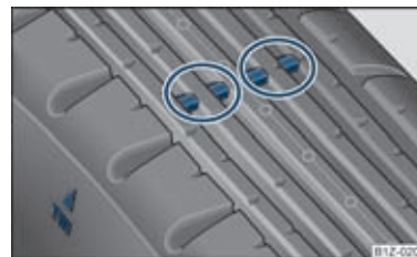
Fig. 158 Tyre tread with wear indicators
