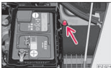
Fig. 172 Jump-starting on vehicles with the START-STOP system
