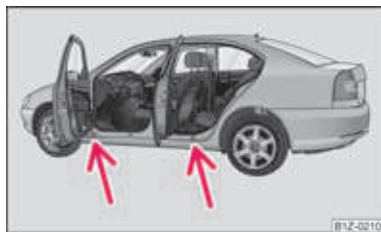
Fig. 167 Changing a wheel: Jacking points for positioning lifting jack
