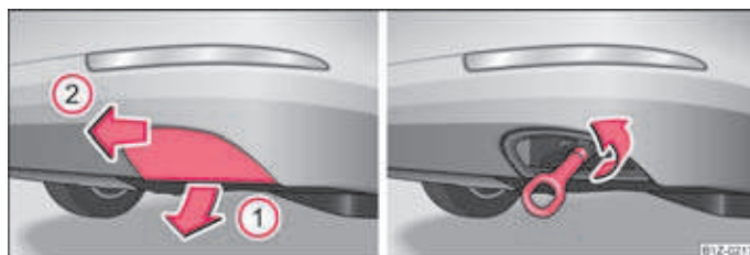
Fig. 175 Rear bumper: Remove cover/rear bumper: Installing the towing eye
