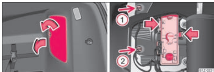
Fig. 189 Luggage compartment: Cover for the lamp holder/removing the lamp holder
