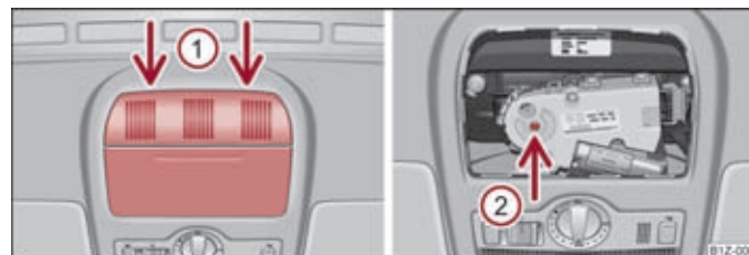
Fig. 23 Detail of the headliner: Points for positioning screwdriver/opening for positioning the key
