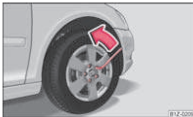
Fig. 166 Changing a wheel: Slackening wheel bolts
