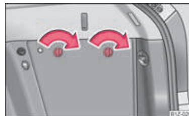
Fig. 161 Placing of the warning triangle (Estate car)
