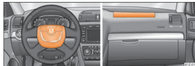
Fig. 122 Driver airbag in the steering wheel/front passenger airbag in the dash panel
