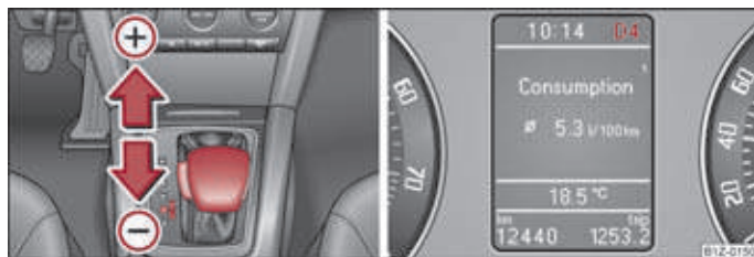
Fig. 107 Selector lever: manual shifting/information display: Manual shifting of gears
