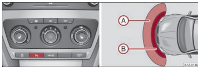
Fig. 103 Activating the parking aid/detection range of the front sensors
