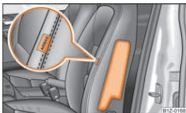
Fig. 125 Driver seat: Installation position of airbag
