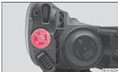
Fig. 182 Removing the light bulb for the turn signal light
