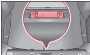
Fig. 160 Placing of the warning triangle (Laura)
