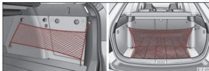
Fig. 54 Fixing net: Vertical pocket/division of the luggage compartment
