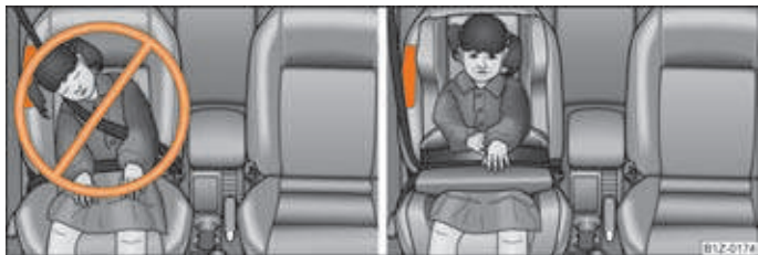
Fig. 131 Seated position of an unprotected child at risk from side airbag/Child properly protected by safety seat
