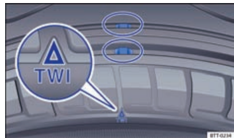
Fig. 94 Tread: Wear indicator.
