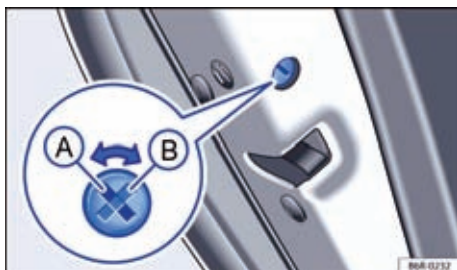
Fig. 17 In the rear left door: Child safety lock Ⓐ is on, Ⓑ is off.
