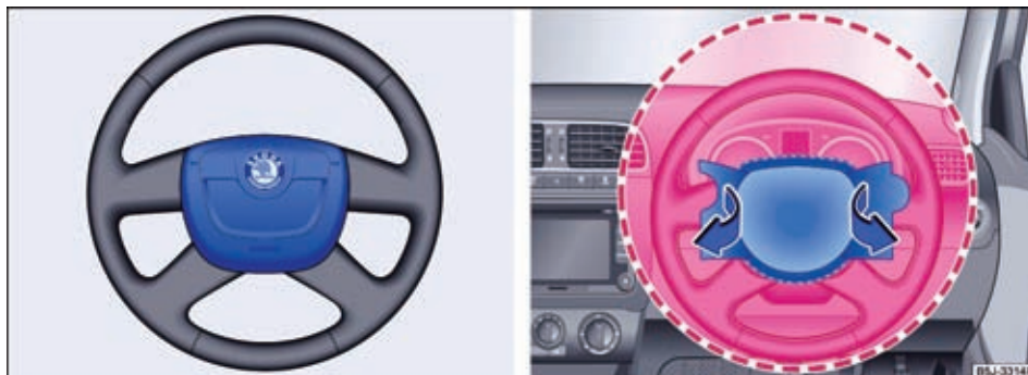
Fig. 41 Installation position and deployment area of the driver's front airbag.
