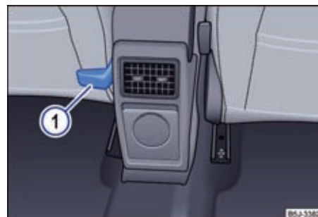
Fig. 26 Control lever on the back of the front passenger seat
