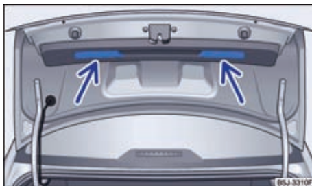
Fig. 21 Open boot lid: Recesses for closing.
