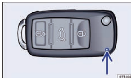
Fig. 13 Indicator light in the vehicle key.
