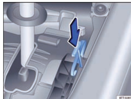
Fig. 104 Emergency unlock the release lever lock.
