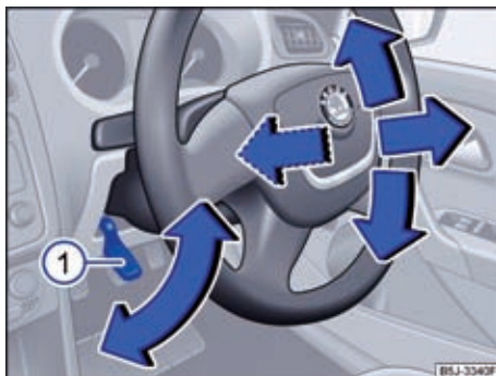
Fig. 28 Mechanical adjustment of the steering wheel position.
