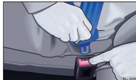
Fig. 37 Release the lock tongue from the belt buckle.
