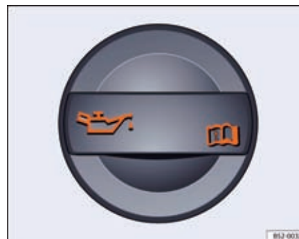
Fig. 85 In the engine compartment: Cap of the engine oil filler opening.
