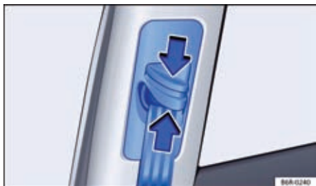
Fig. 40 At the side of the front seats: Seat belt height adjusters.
