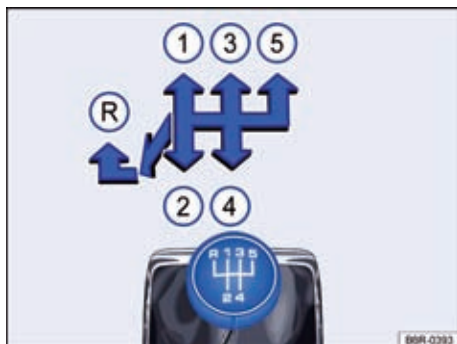
Fig. 69 Shift pattern of the 5-speed manual gearbox.
