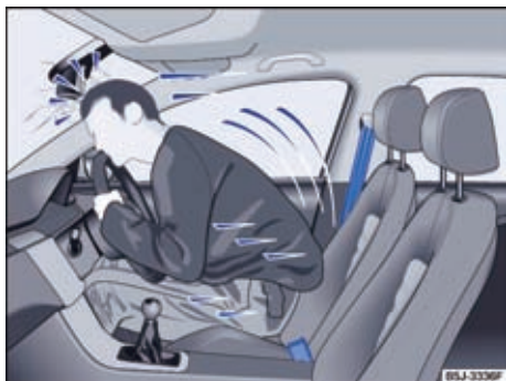
Fig. 33 The driver not wearing a seat belt is catapulted forward.
