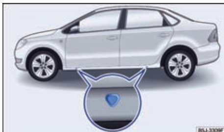
Fig. 111 Jacking points for positioning the jack.
