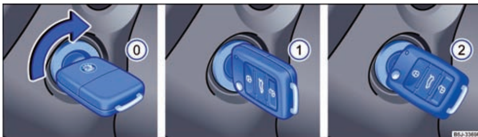
Fig. 66 Positions of the vehicle key in the ignition lock.
