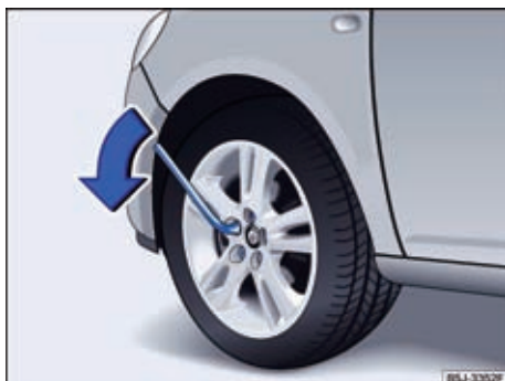
Fig. 109 Changing a wheel: Slackening the wheel bolts.
