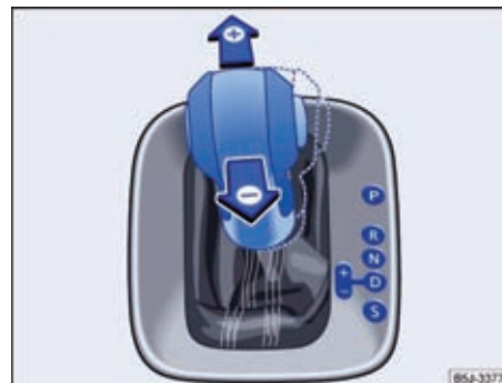
Fig. 71 Selector lever in Tiptronic position.
