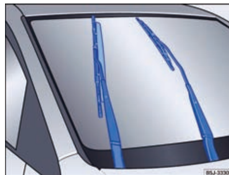
Fig. 89 Windscreen wiper in service position.
