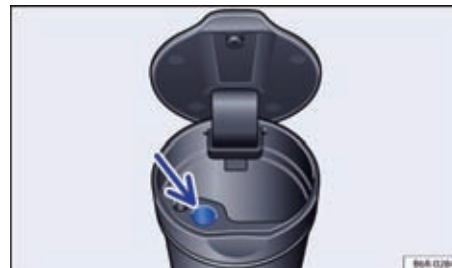
Fig. 91 Removed and opened ashtray with cigarette extinguisher.
