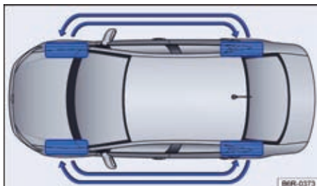
Fig. 92 Pattern for the exchange of the wheels.
