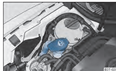
Fig. 178 Engine compartment: Windshield washer fluid reservoir
