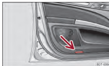
Fig. 45 Front door: Warning light
