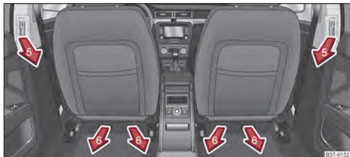
Fig. 109 Air vents at the rear
