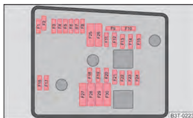
Fig. 201 Schematic representation of fuse box in engine compartment - version 2
