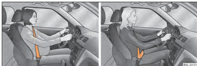
Fig. 118 Routing of belt webbing for an expectant mother/routing of belt webbing over the shoulders and the lap belt
