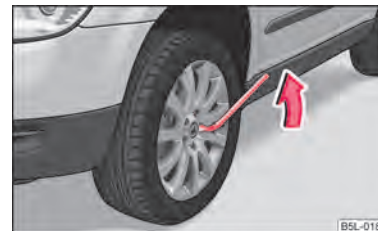
Fig. 168 Changing a wheel: Loosening the wheel bolts
