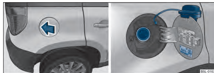
Fig. 150 Right rear side of the vehicle: Open fuel filler flap/fuel filler flap with cap unscrewed
