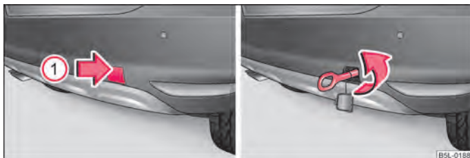
Fig. 176 Rear bumper: Removing the cover/installing the towing eye
