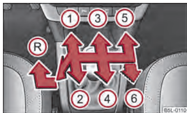
Fig. 97 The shift pattern: 5-speed or 6-speed manual gearbox
