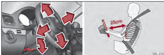
Fig. 95 Adjustable steering wheel: Lever next to the steering column/safe distance to the steering wheel
