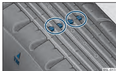
Fig. 161 Tyre tread with wear indicators
