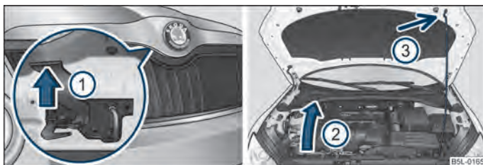
Fig. 152 Radiator grille: Locking lever/securing the bonnet with the bonnet support
