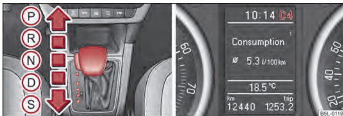
Fig. 106 Selector lever/information display: Selector lever positions
