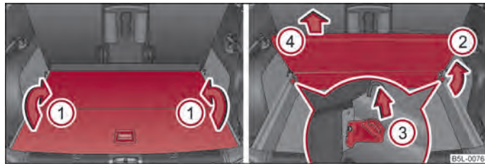
Fig. 63 Luggage compartment: Fold up variable loading floor/remove
