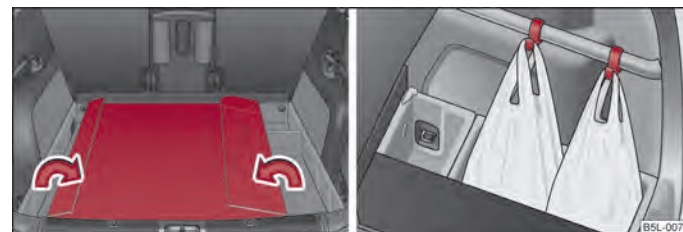
Fig. 65 Luggage compartment: Fold the side parts of the loading floor/example for using the variable loading floor
