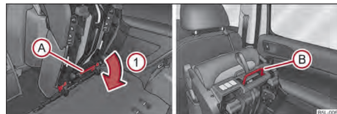
Fig. 52 Unlocking the folded forward seat/carrying handles on the seat cushion
