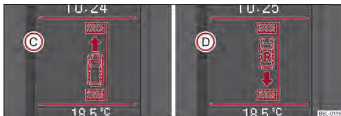
Fig. 103 Information display: Information for engaging the forward gear (C) or the reverse gear (D)
