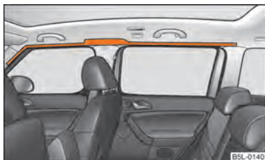
Fig. 127 Installation position of the head airbags
