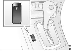
Switch for operation of central locking
