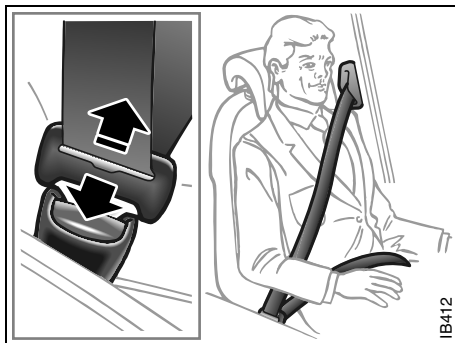
Press the red button to release the belt
