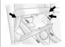
Lower the loosened glove box housing.
