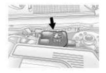
The surge tank is located on the driver side of the engine compartment. See *Engine Compartment Overview on page 10-6* for more information on location.
