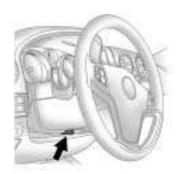
The lever is located on the left side of the steering column.
