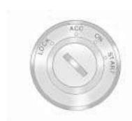
The ignition switch has four different positions.
