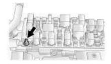
Your vehicle is equipped with a remote positive (+) terminal. This is located in the engine compartment on the driver side
