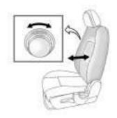
If the vehicle has this feature, the knob is located on the inboard side of the driver seatback.
