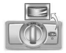
Turn the thumbwheel to the right or left to brighten or dim the instrument panel lights.
