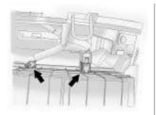
3. Unplug both wire cables and remove the glove box.
