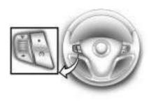
The cruise control buttons are on the left side of the steering wheel.
