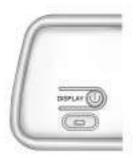
The video display will default back to on when the ignition is cycled, or the vehicle is put back in R (Reverse).
