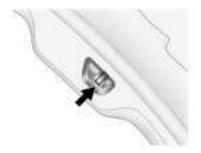
To open the liftgate if the vehicle's battery is disconnected or the voltage is low, access the release lever. Remove the interior trim cover on the inside of the liftgate. Use a tool to push the lever on the latch until the liftgate releases.
