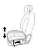
On vehicles with this feature, move the lever upward repeatedly to raise the seat.
