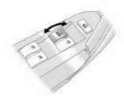
The window switches for all doors are located on the driver door. Each passenger door has a switch that controls only that window.
