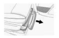
For vehicles with a storage area located under the front passenger seat, lift up on the end of the tray and pull it forward to access it.
