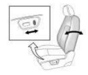
If the seats have power reclining seatbacks, the control used to recline them is located on the outboard side of the seat.
