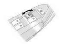
All window switches are located on the driver door. Each passenger door has a switch that controls only that window. Press the front of the switch to open the window. Pull the switch up to close it.
