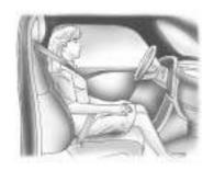
If a person of adult-size is sitting in the right front passenger seat, but the off indicator is lit, it could be because that person is not sitting properly in the seat. If this happens, use the following steps to allow the system to detect that person and enable the right front passenger frontal airbag and seat-mounted side impact airbag:
