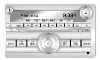
(Power/Volume): Press to turn the system on and off.
