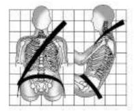
Sit up straight and always keep your feet on the floor in front of you. The lap part of the belt should be worn low and snug on the hips, just touching the thighs. In a crash, this
