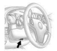
The lever is located on the left side of the steering column.
