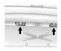
Turn and pull the license plate lamp forward through the fascia opening.
