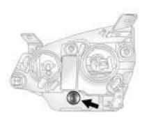
Turn the bulb to be replaced counterclockwise to remove it from the headlamp assembly.
