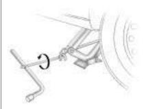
Lower the vehicle by turning the jack handle counterclockwise.
