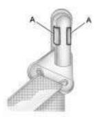
Squeeze the release buttons (A) together and move the height adjuster up or down to the desired position.
