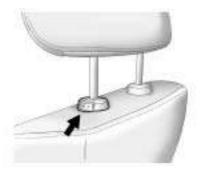
Pull the head restraint up to raise it. To lower the head restraint, press the button, located on the top of the seatback, and push the restraint down.
