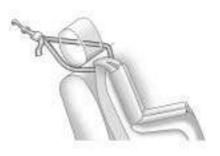
If the position you are using has an adjustable headrest or head restraint and you are using a dual tether, route the tether around the headrest or head restraint.
