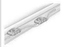
If the level of the shoulder is only slightly below the pavement, recovery should be fairly easy. Ease off the accelerator and then, if there is nothing in the way, steer so that the vehicle straddles the edge of the pavement. Turn the steering wheel 8 to 13 cm (3 to 5 inches), about one-eighth turn, until the right front
