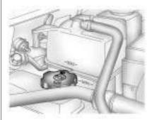
Fill the coolant surge tank with the proper DEX-COOL® coolant mixture, to between the MIN and MAX lines.
