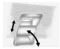
Slide and release the switch rearward to express open the sunroof. Slide the switch forward or rearward to stop movement.
