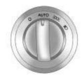
The exterior lamp control is on the instrument panel to the left of the steering wheel.
