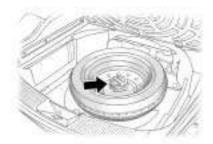
Place the wheel retainer bolt onto the wheel stow rod and tighten by turning it clockwise. The compact spare is for temporary use only. Replace the compact spare tire with a full-size tire as soon as possible.
