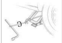
Raise the vehicle by turning the jack handle clockwise. Raise the vehicle far enough off the ground so there is enough room for the road tire to be removed.
