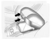
Your vehicle has a center console with an upper, lower and rear storage area. To access the upper storage area, lift up on the top lever. To access the lower storage area, lift up on the bottom lever. The top of the center console can extend forward. To adjust, hold the top of the lever up and pull the top of the center console forward.
