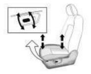
To raise or lower the front or rear part of the seat cushion, move the front or rear of the control up or down.
