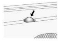
Do not cover the light sensor on top of the instrument panel or the headlamps will come on when they are not needed.
