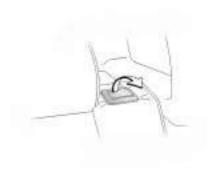
Lift the lever located on the top of the seatback to release the seatback and fold the seatback forward.
