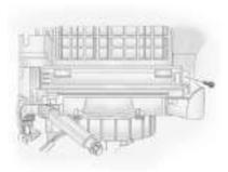
4. Remove the air filter cover screw.
