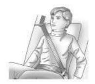
Buckle, position, and release the safety belt as described previously in this section. Make sure that the shoulder belt crosses the shoulder.
