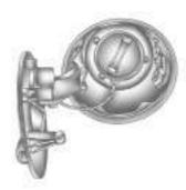
The tethered fuel cap is located behind a hinged fuel door on the driver side of the vehicle.
