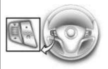
The cruise control buttons are on the left side of the steering wheel.
