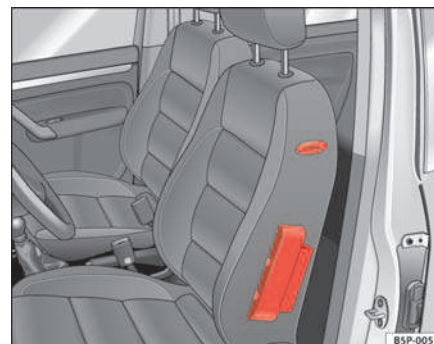
Fig. 22 Side airbag in driver seat
