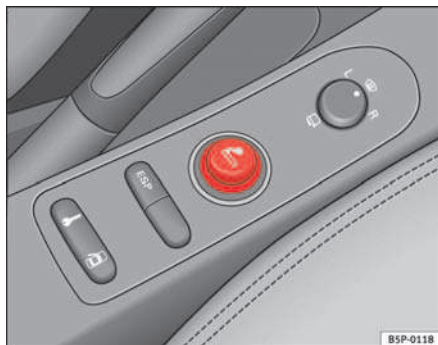
Fig. 114 The cigarette lighter is located in the electric socket on the front of the centre console
