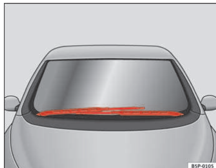
Fig. 158 Windscreen wipers in the service position
