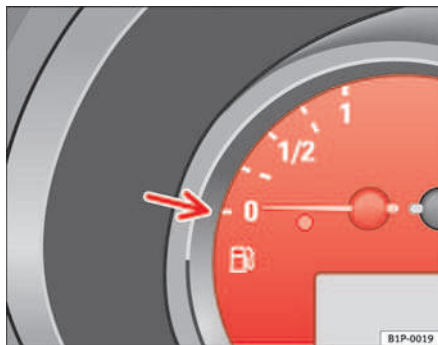
Fig. 34 Details of the instrument panel: Fuel gauge
