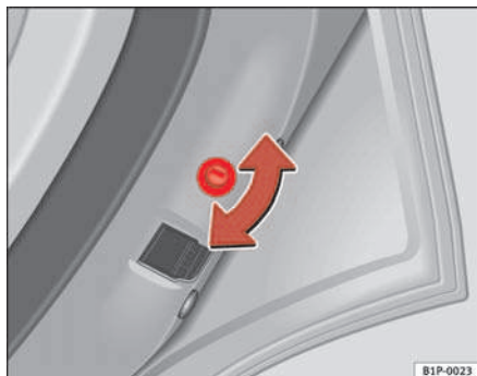
Fig. 62 Child safety lock on the right hand side door
