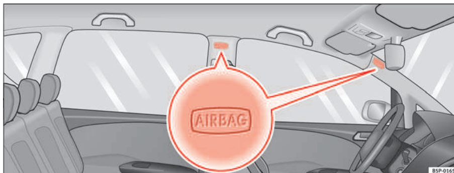
Fig. 24 Location of left curtain airbag
