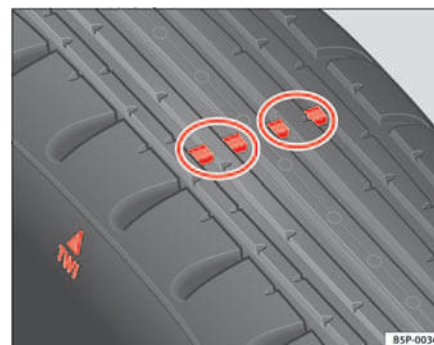
Fig. 162 Tyre tread wear indicators
