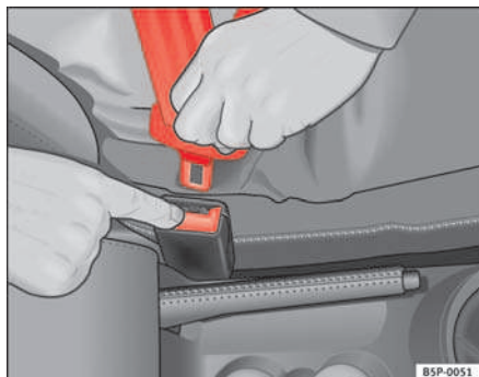
Fig. 16 Removing latch plate from buckle
