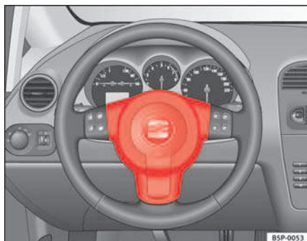
Fig. 18 Driver airbag located in steering wheel
