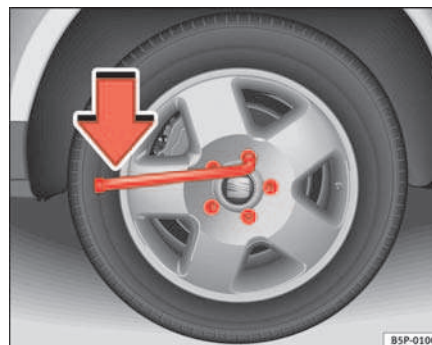
Fig. 166 Changing the wheel: Loosening the wheel bolts
