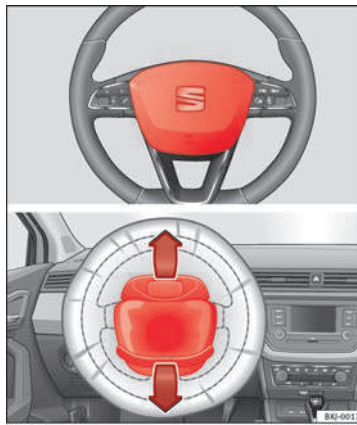
Fig. 17 Driver airbag located in steering wheel.
