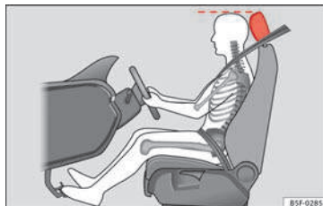
Fig. 78 Correct head restraint position for the driver.
