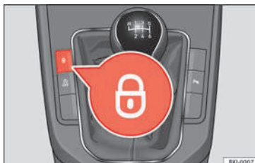
Fig. 2 Centre console: Central lock buttons.
