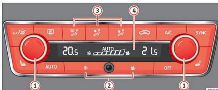
Fig. 49 In the centre console: Climatronic controls
