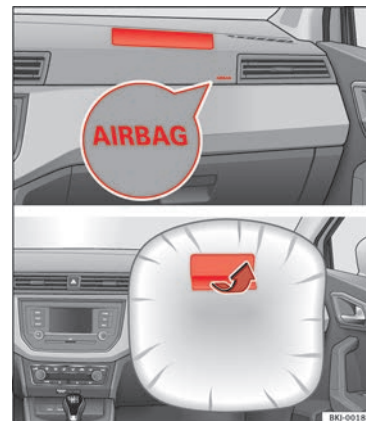
Fig. 18 Front passenger airbag located in dash panel.
