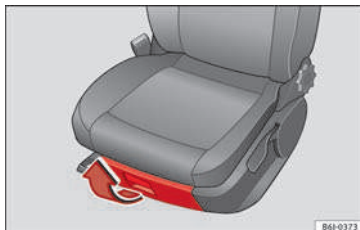
Fig. 134 Storage compartment under the right front passenger seat.
