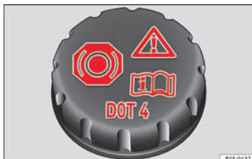
Fig. 56 Engine compartment: brake fluid reservoir cap.
