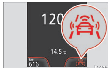
Fig. 159 On the instrument panel display: Front Assist switched off message.
