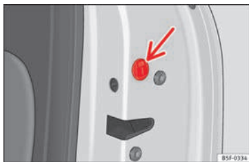
Fig. 4 Locking the door manually.
