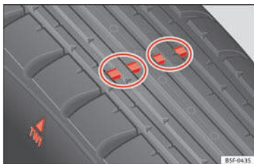
Fig. 195 Tyre tread wear indicators.
