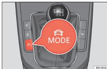
Fig. 170 Next to the gear lever. MODE button.
