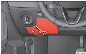
Fig. 58 On the driver-side dash panel: fuse box cover.
