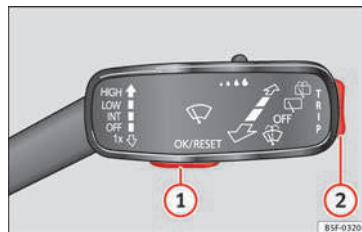
Fig. 39 Windscreen wiper lever: control buttons.
