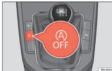
Fig. 152 Centre console: Start-Stop system button.
