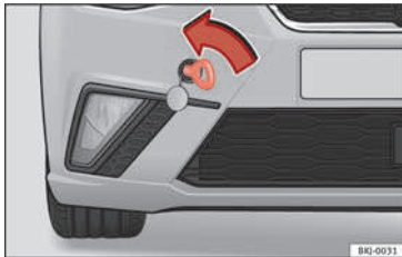
Fig. 70 Right side of the front bumper: Towing ring.
