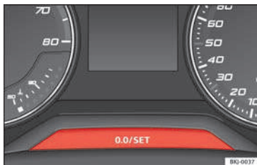
Fig. 107 Instrument panel: odometer and reset button.
