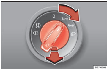
Fig. 124 Dash panel: light control.
