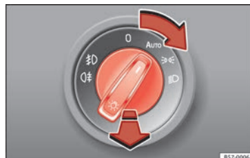
Fig. 32 Dash panel: light control.
