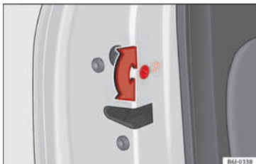
Fig. 121 Childproof lock on the left hand side door.
