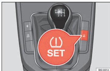
Fig. 197 Centre console: tyre monitoring system button.
