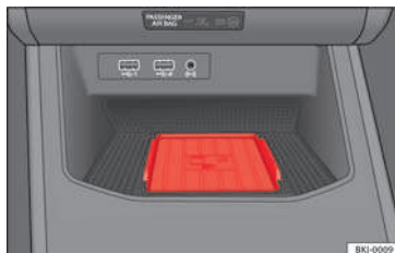
Fig. 112 Centre console: Connectivity Box.
