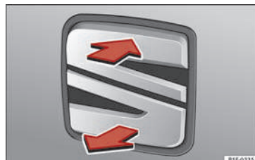
Fig. 5 Rear lid: opening from the outside.
