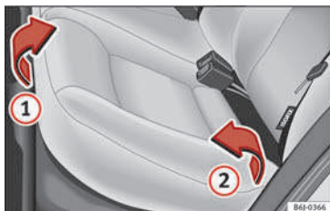
Fig. 131 Folding up the rear seat cushion.
