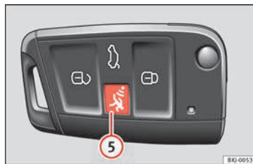
Fig. 115 Vehicle key with alarm button.
