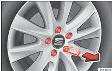
Fig. 65 Wheel: wheel bolts with caps.
