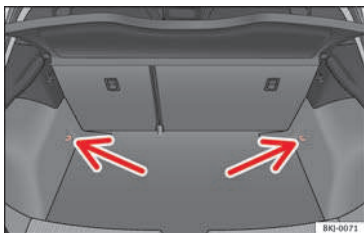
Fig. 142 Location of fastening rings in luggage compartment.
