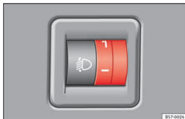
Fig. 125 Dash panel: headlight range control.
