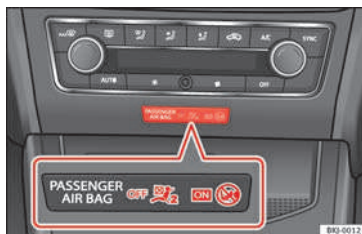
Fig. 47 Warning lamp for disabling the front passenger airbag.
