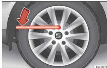
Fig. 66 Changing a wheel: loosen the wheel bolts.
