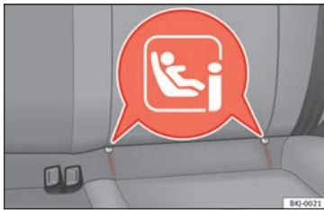
Fig. 26 ISOFIX/iSize securing rings.
