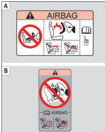
Fig. 23 Airbag stickers - version 1: on the front passenger's sun visor A and on the rear frame of the front passenger's door B .
