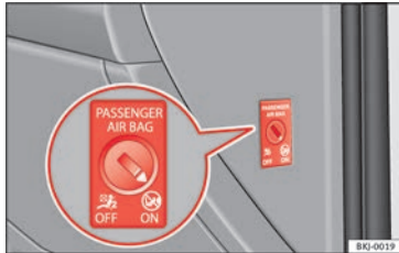
Fig. 19 Front passenger front airbag switch.
