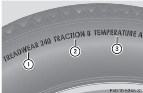
The Uniform Tire Quality Grading is a U.S. Government requirement designed to give drivers consistent and reliable information regarding tire performance. Tire manufacturers are required to grade tires based on three performance factors:
