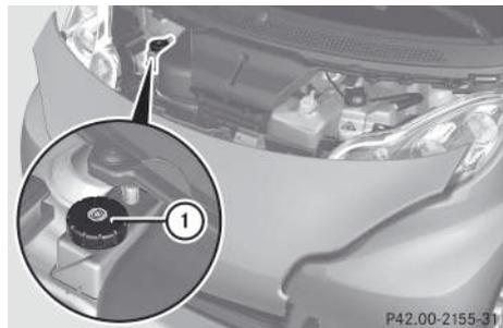
**Checking brake fluid level**
