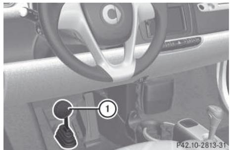
If a brake circuit has failed (▷ page 164), you must depress brake pedal **1** further down to achieve the same effect and the braking distance is increased.
