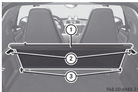
If you wish to use cargo compartment cover blind (1) as normal, assemble it in top mountings (2). If you do not need the cargo compartment cover blind, insert in bottom mountings (3).
