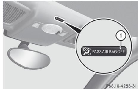
Passenger front air bag off indicator lamp ① illuminates when the passenger front air bag is deactivated.
