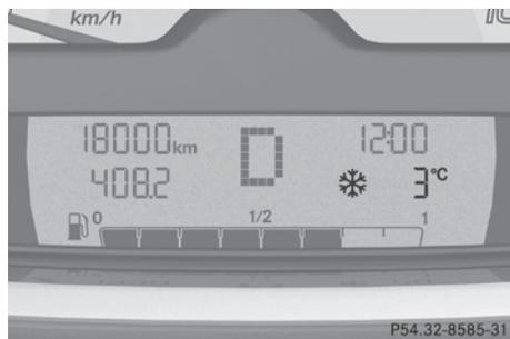
When the outside temperature falls below 3°C, the multifunction display makes you aware of the fact that the road may be icy. An additional freeze warning, i.e. an ice crystal symbol, in the multifunction display flashes. After 60 seconds, the freeze warning stops flashing but continues to be displayed. When the outside temperature rises above 3°C, the freeze warning goes out.
