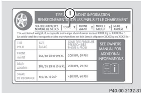
The seating capacity gives you important information on the number of occupants that can be in the vehicle. The Tire and Loading Information placard showing seating capacity ① is located on the driver's door B-pillar (▷ page 130).
