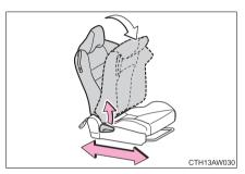
Lift the seatback angle adjustment lever.
