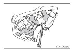
The pretensioner helps the seat belt to quickly restrain the occupant by retracting the seat belt when the vehicle is subjected to certain types of severe frontal collision and/or side collision.
