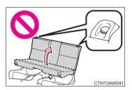
Make sure that the seatback is securely locked in position by lightly pushing it back and forth.
