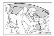
The SRS side airbag and SRS curtain shield airbag can function only when the engine switch is in the "ON" position.
